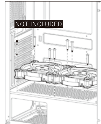
(6c) Install PSU Fans
