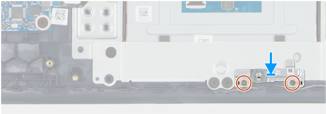
Figure 42. Installing the battery bracket
