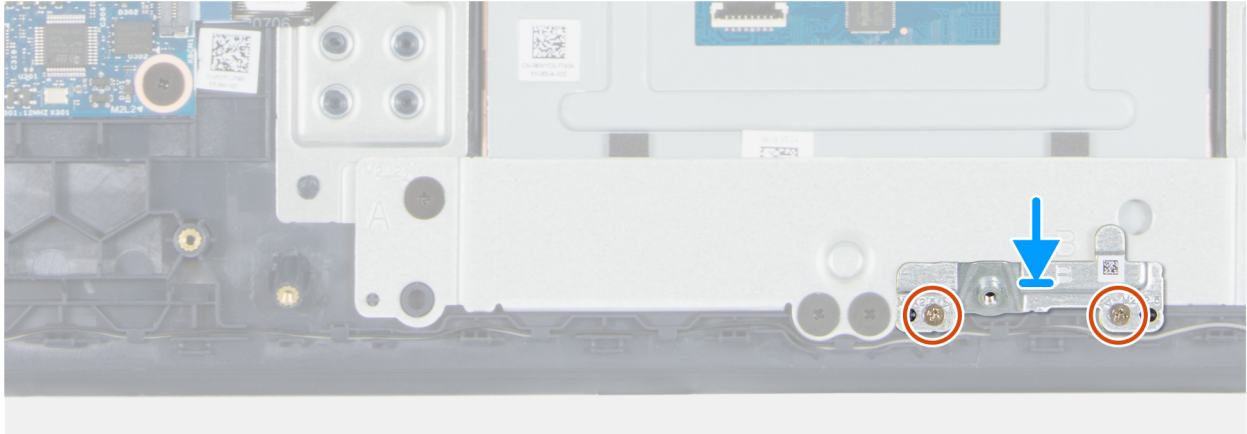
Figure 42. Installing the battery bracket
