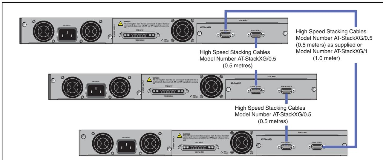
Figure 34. VCStack Ring Topology Using x610 Switches
