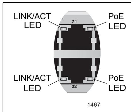
Figure 14. Port LEDs on PoE+ x610 Series Switches
