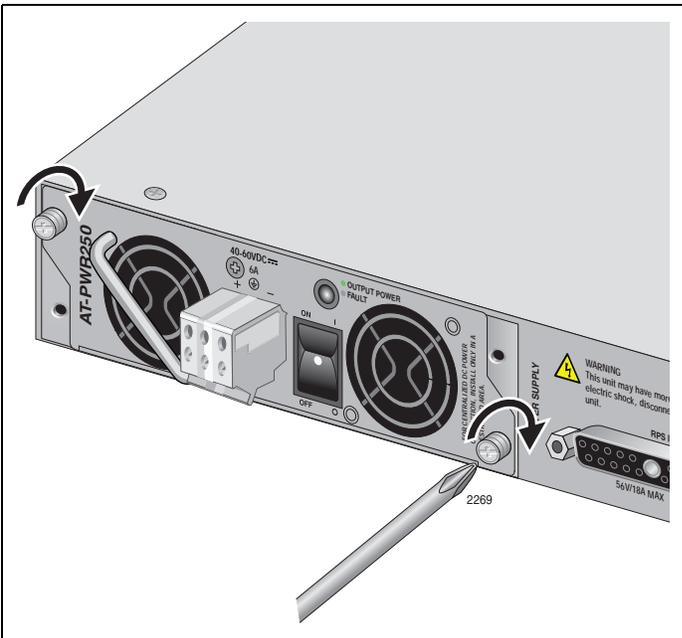
Figure 53. Securing the DC AT-PWR250 Power Supply Module
