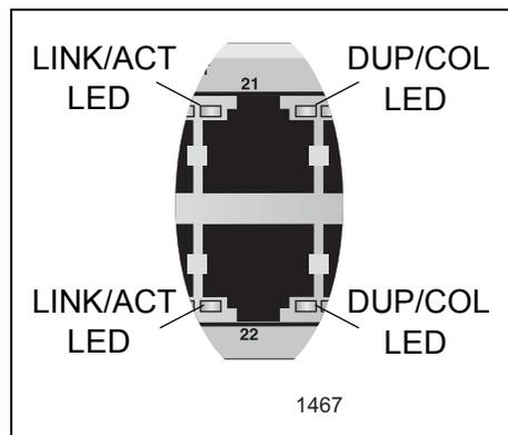
Figure 13. Port LEDs on non-PoE+ x610 Series Switches
