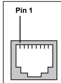
Figure 78. RJ-45 Connector and Port Pin Layout
