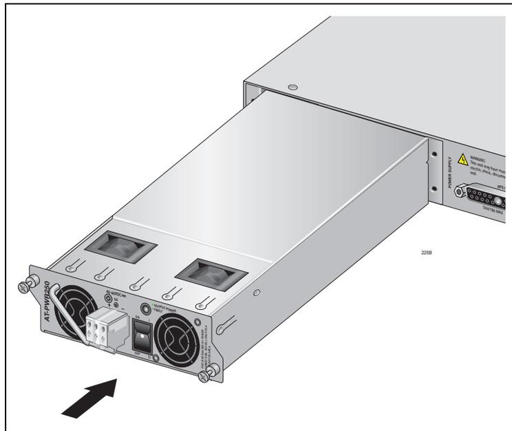
Figure 49. Installing the DC AT-PWR250 Power Supply Module
