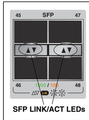
Figure 18. SFP LEDs on x610-48Ts and x610-48Ts-POE+ Switches
