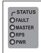
Figure 20. System STATUS LEDs on the Front Panel
