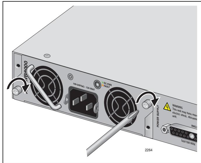
Figure 54. Securing the AT-PWR800 Power Supply Module
