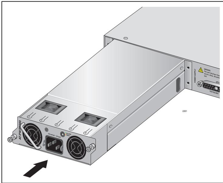
Figure 50. Installing the AT-PWR800 Power Supply Module
