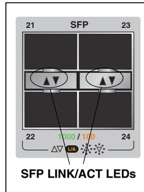
Figure 15. SFP LEDs on x610-24Ts and x610-24Ts-POE+ Switches
