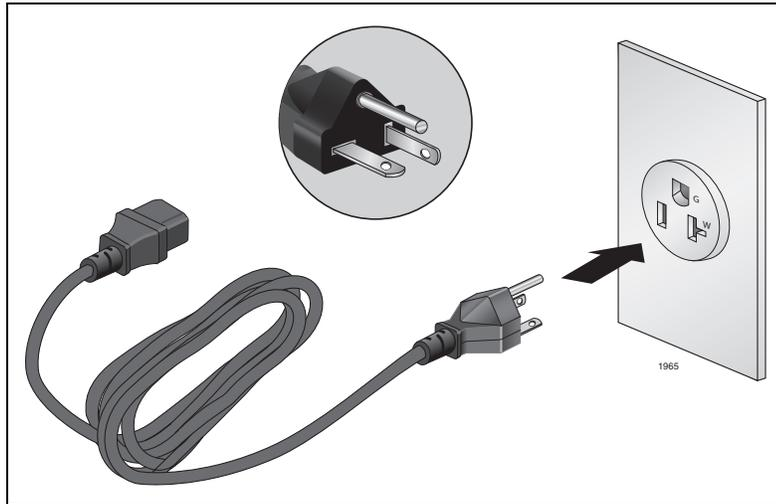
Figure 76. 100-125 VAC 125 V NEMA 5-20 Plug and Receptacle
