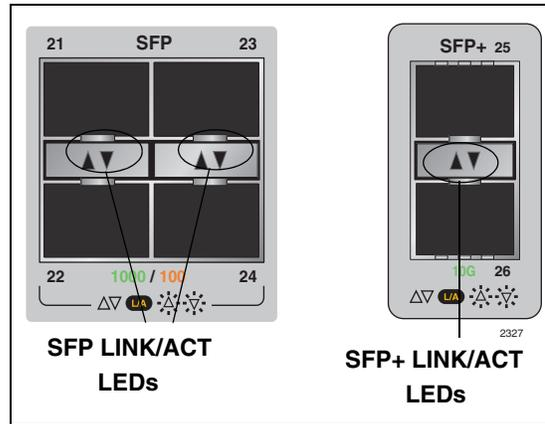
Figure 17. SFP and SFP+ LEDs on x610-24SPs/X Switch
