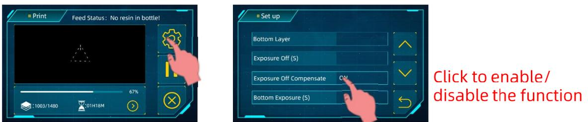
The compensation only works on bottom layers and layers with large area. In normal layers, off time is automatically added according to the area of layers; the larger the area, the longer the off time.
