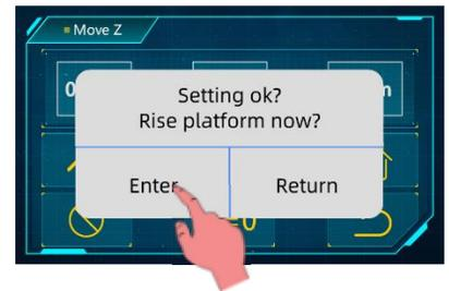
9. Detection: Raise printing platform until the curing screen can be observed completely. Return to Tools menu and click "Detection", set the test time and then click "Next". The curing screen should display a complete image as shown below.
