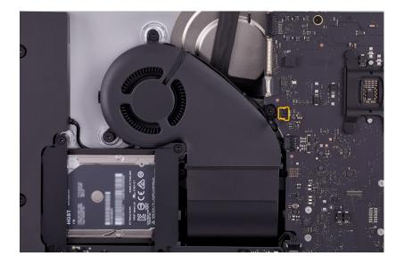
3. Remove the three T10 screws from the fan.
