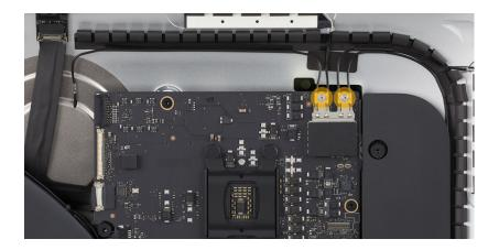
3. Use the antenna tool to disconnect the connector from the logic board.
