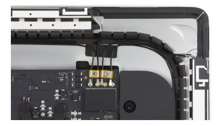
4. Use the blunt end of the antenna tool to reconnect the antenna to the logic board.
