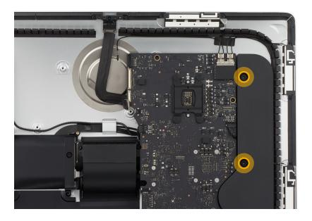
3. Use a black stick to disconnect the audio cable from the lower right corner of the logic board.
