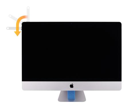
5. Roll the tool back and forth along the top and sides of the computer until the wheel moves with minimal resistance.
