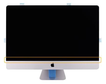
9. Hold the display removal tool against the sides of the display to check the alignment. Adjust the display placement if necessary.
