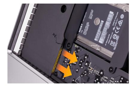
6. Remove the two T10 screws from the left speaker.
