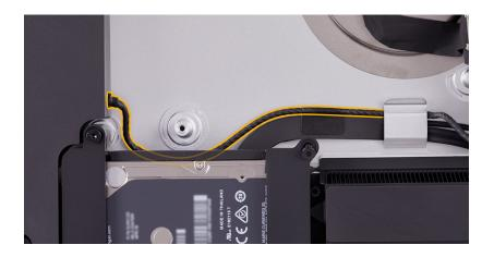
10. Reinstall the two T8 screws into the hard drive bracket.
