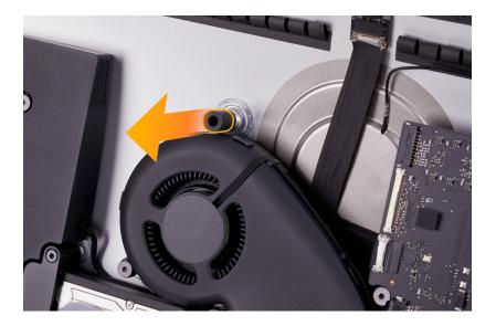
2. Use a black stick to disconnect the fan cable from the logic board.
