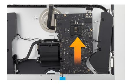
20. Remove the logic board from the rear housing.
