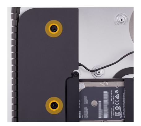
7. Pull the left speaker up just enough to see the power button cable. Remove the power button cable from the channel.
