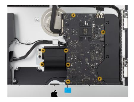
7. Replace the piece of round Mylar tape on the lower left logic board screw. If the Mylar tape is missing, cover the screw with a small piece of Kapton tape.
