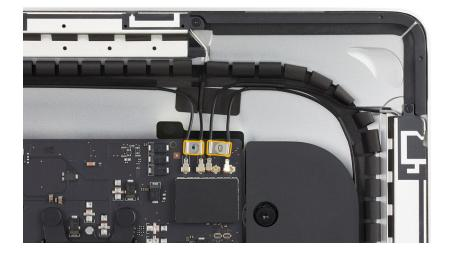
14. Use the antenna tool to reconnect the cable to the logic board.
