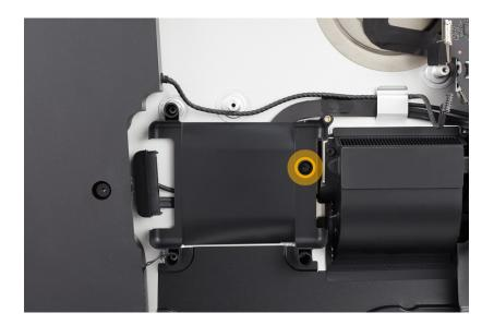
10. Remove the hard drive cable from the back of the hard drive cradle.
