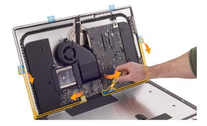
15. Remove the remaining release liners from the top and sides of the display.
