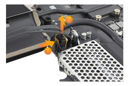
2. Gently pull the hard drive power cable connector to disconnect the cable from the logic board.
