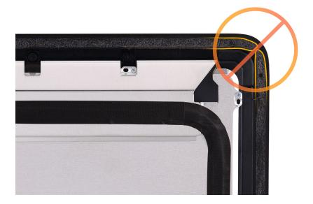
15. Use your fingers and the flat end of a black stick to peel residual adhesive upward from the bottom sides of the rear housing.
