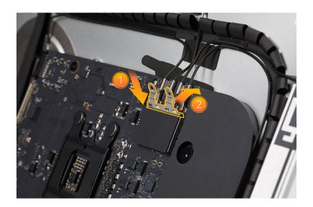
6. Reinstall the two T5 screws into the antenna cowling.
