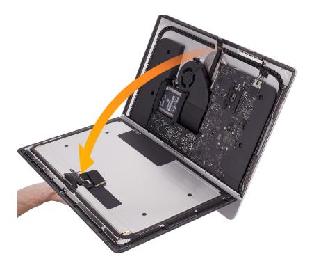
Locate the display adhesive tabs at the bottom corners of the display and pull each toward the center to release the display from the rear housing.
