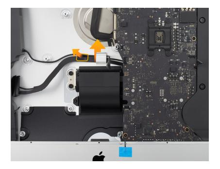
12. Hold the wireless card support tool by the handle. Lower the tool (1) so it rests on the edge of the logic board. Then slide the tool to the right (2) behind the logic board near the antenna connectors.
