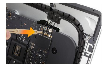
5. Reinstall the antenna cowling by engaging the teeth at an angle. Then position it over the antenna connectors.
