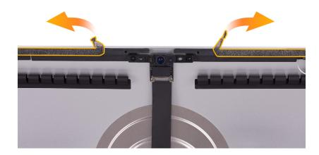
14. Use your fingers and the flat end of a black stick to peel residual adhesive outward from the top center of the display.
