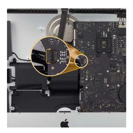
9. Remove the T8 screw from the hard drive cradle.
