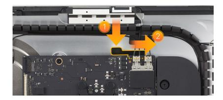
2. Remove the two T5 screws from the antenna cowling. Set the cowling aside for reuse.
