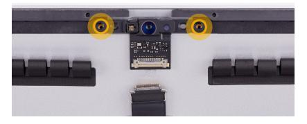
2. Reinsert the camera cable in the camera board connector. Flip the locking bar to secure the cable.
