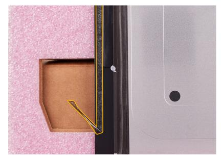
17. Use an IPA wipe to remove any remaining adhesive from the rear housing and display edges. Allow the surfaces to dry for 1 minute.
