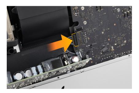
3. Reconnect the power supply signal cable.
