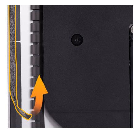
16. Use your fingers and the flat end of a black stick to peel residual adhesive upward from the bottom sides of the display.
