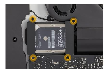
3. Remove the hard drive brackets. Do not remove the bumpers.
