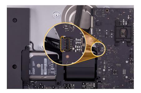
7. Reconnect the power button cable to the power supply.
