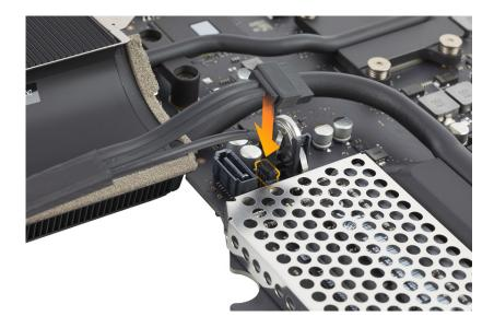
2. Reinsert the hard drive data connector into the logic board.
