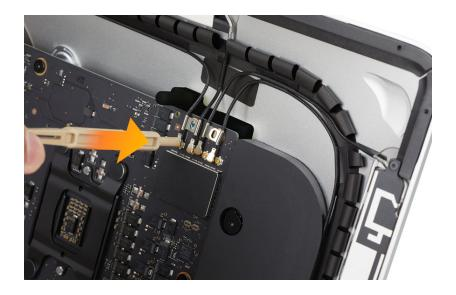
15. Reinstall the antenna cowling by engaging the teeth at an angle; then lay it down over the antenna connectors.
