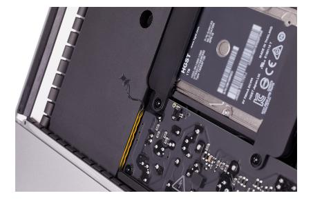
4. Fully reinsert the left speaker into the rear housing chin. Ensure that the power button cable does not bind or slip out of the routing channel as you position the speaker.
