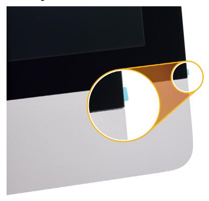
12. Anchor the display further with a vertical strip of painters tape on both ends of the horizontal strip.
