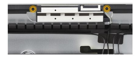
6. Remove the antenna from the rear housing.
