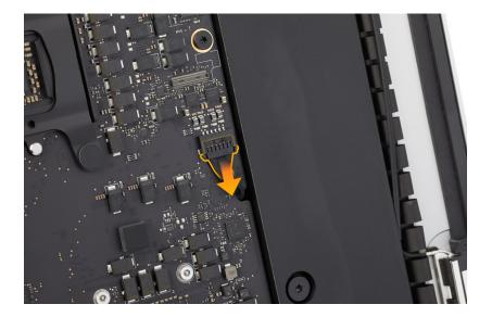
2. Remove the two T10 screws from the right speaker and disconnect the speaker.
