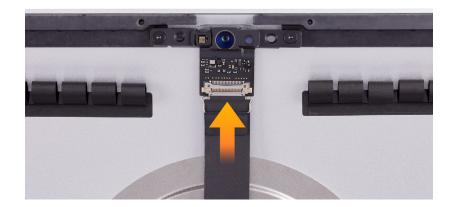
3. If the camera cable was replaced, connect the camera cable to the logic board connector. Flip the locking bar to secure the cable.
