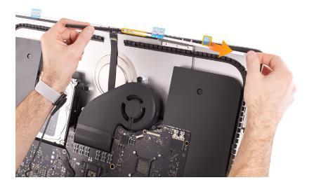
7. Use the two strips of display adhesive along the bottom edge. There are no guide holes on the display adhesive strips or along the bottom of the rear housing, so align the strips by hand.
