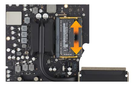
4. Hold the memory by the edges and gently remove it from the slot.
