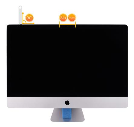
3. Continue to roll the tool around the top right corner and down the right side of the computer.
