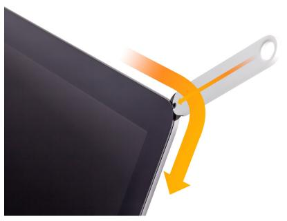
4. Roll the tool around the top left corner and down the left side of the computer.
