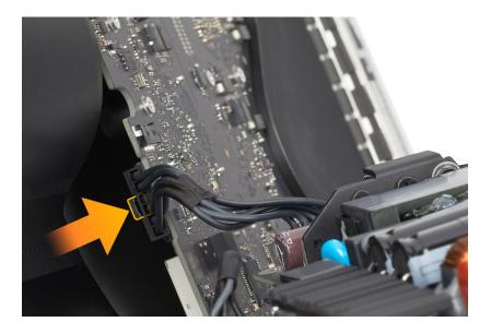
6. Disconnect the AC cable from the AC filter in the rear housing.
