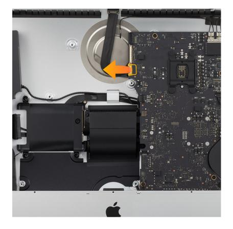
5. Flip the locking bar on the bottom section of the logic board. Gently pull the microphone flex cable out of the connector to disconnect it.
