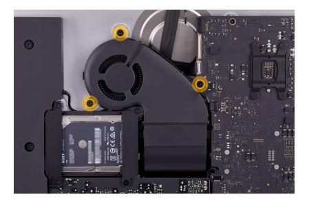
2. Reconnect the fan cable to the logic board. Ensure the cable is routed as shown.
