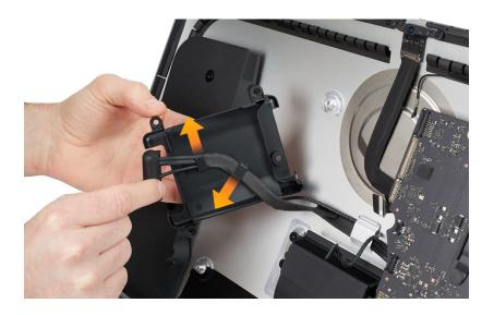
11. Loosen the black tape that adheres the speaker cable to the hard drive data and power cable. Remove the speaker cable and the hard drive data and power cable from the clip on the rear housing.
