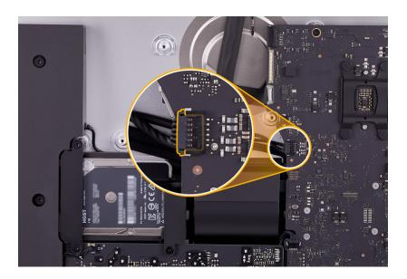
3. Remove the sticker that adheres the speaker cable to the hard drive data and power cable; then remove it from the clip.
