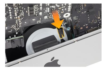
2. Slip the power supply under the rear housing chin. Reconnect the DC cable to the logic board.
