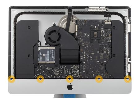
Note: For easier installation of the small chin strap screws, use a black stick to press the chin strap against the front frame if needed. Do not press on the chin. Always press on the back of the chin strap to bring it toward the screw.
