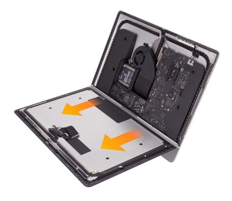
13. Use your fingers and the flat end of a black stick to peel residual adhesive outward from the top center of the rear housing.
