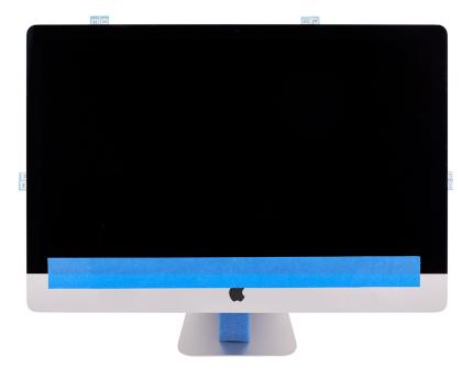
11. Step back and check the alignment of the display. If the display is not flush with the rear housing, adjust the display and recheck alignment.
