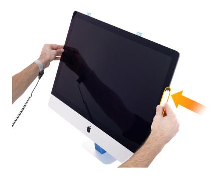
10. Anchor the display with a strip of painters tape. Place the tape horizontally where the bottom of the display meets the chin.
