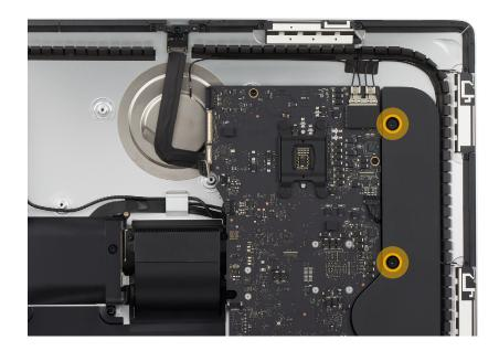
5. Tuck the antenna cable into the channel on the right side of the speaker.
