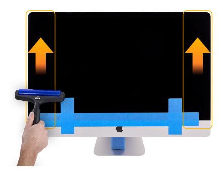
19. Roll the silicone display roller along the top in a horizontal back-andforth motion.
