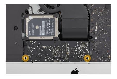
5. Reconnect the power button cable to the power supply and reroute it along the side of the left speaker.
