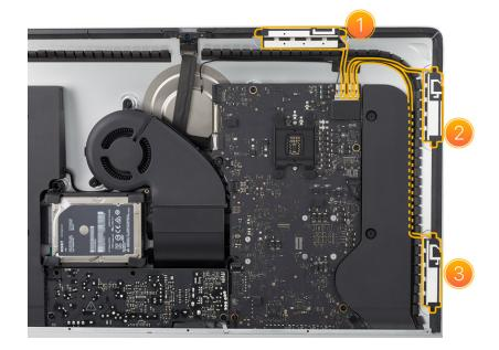
1. Hold the wireless card support tool by the handle, lower the tool so it rests on the edge of the logic board (1). Then slide the tool to the right behind the logic board near theantenna connectors (2).
