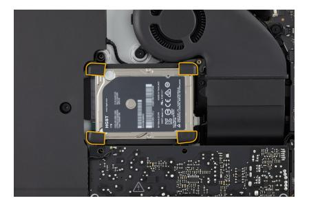
4. Disconnect the hard drive power and data cable from the hard drive.
