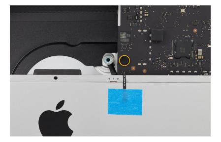
8. Reroute the hard drive data and power cable through the clips in the hard drive cradle.
