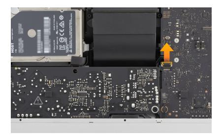
4. Remove the two T8 screws from the power supply.
