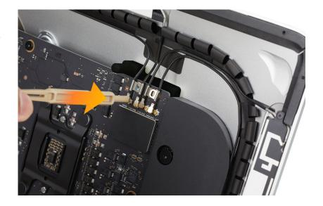
5. Remove the two T4 screws from the antenna.
