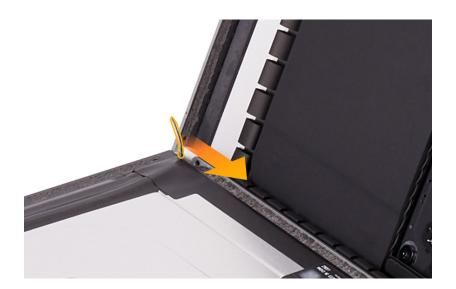
12. Pull the display from the rear housing and set it face down on a soft cloth on the display support stand.
