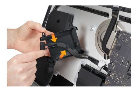
9. Reinstall the T8 screw in the hard drive cradle.
