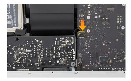
4. Reinstall the two T8 screws in the power supply.
