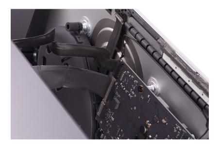
9. Disconnect the embedded DisplayPort (eDP) cable and the display backlight power cable.
