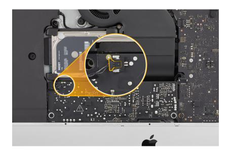
3. Disconnect the power supply signal cable.
