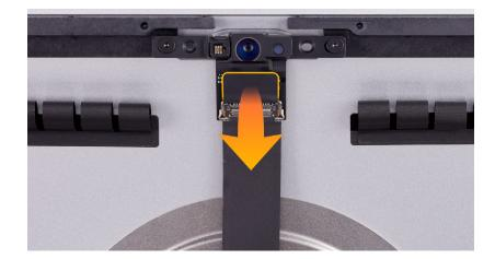
2. Remove the two T5 screws from the camera board.
