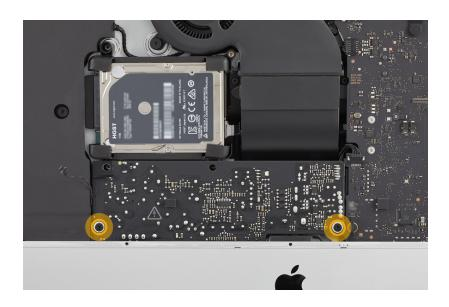
5. Slide the power supply out of the chin as far as it will go. Disconnect the DC cable from the logic board.
