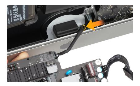
7. Lift the power supply up and out of the chin well.
