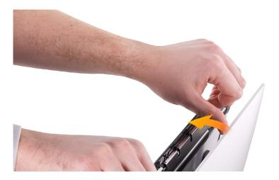
8. Tilt open the display just enough for your hand to reach the cables connecting the display to the logic board.
