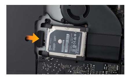
2. Position the hard drive brackets as shown. The brackets will only install one way.
