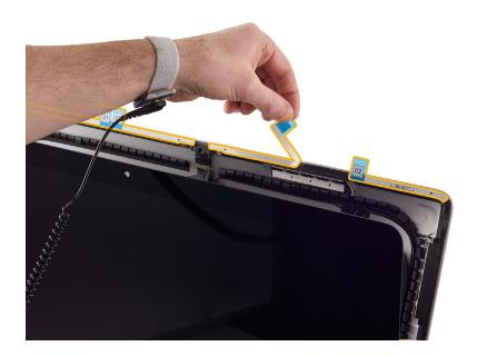
16. Tilt up the display, leaving enough room to connect the eDP cable and the display backlight power cable to the logic board. Ensure the connectors are firmly seated.
