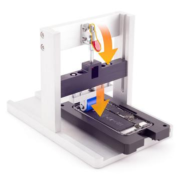
7. Slide the repair tray back and forth through the battery press three times to adhere the battery to the enclosure.
