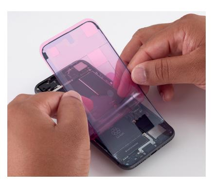
4. Use the black stick to press the display adhesive onto the perimeter of the enclosure.
