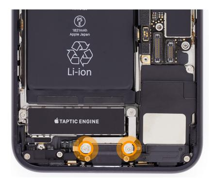
12. Use the black torque driver and Micro stix bit to install one new trilobe screw into the Taptic Engine connector cowling.
