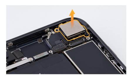
4. Use the flat end of the black stick to lift the end of the camera flex cable off the connector.
