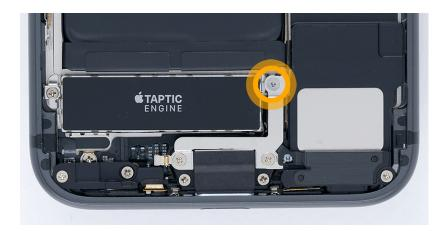
2. Use a torque driver and the JCIS bit to remove the two crosshead screws from the Taptic Engine connector cowling. Set aside the screws.
