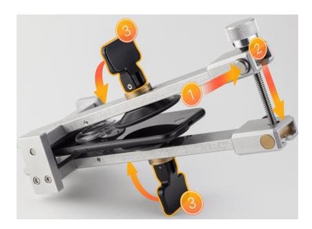
6. Press and hold the release button on the adapter and slowly separate the levers until you feel resistance.
