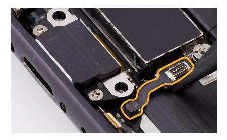
6. Press the end of the Taptic Engine flex cable to the Taptic Engine/dock connector.
