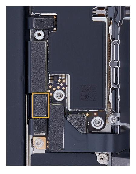
Use the black stick to gently lift the ends of the display flex cable (1) and Home button flex cable (2) off the connectors.
