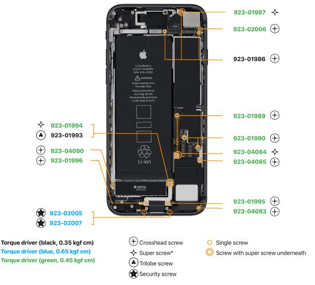
\*A super screw has a threaded hole that holds another screw.
