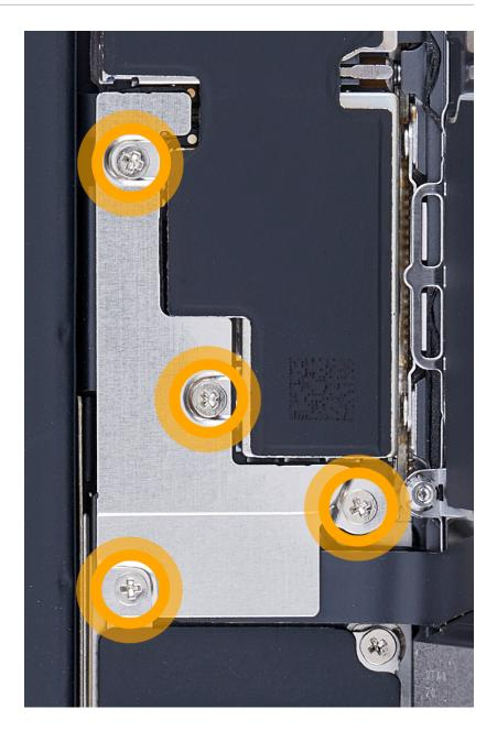
15. Use a torque driver and the JCIS bit to remove the four crosshead screws from the battery/display connector cowling. Set aside the screws.
