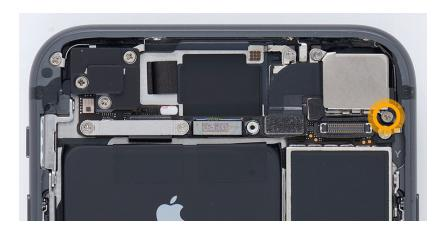
7. Fully torque the two screws into the camera cowling.
