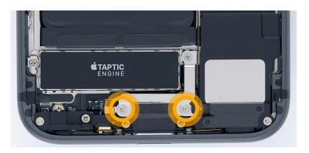
3. Remove the Taptic Engine connector cowling and save it for reassembly.
