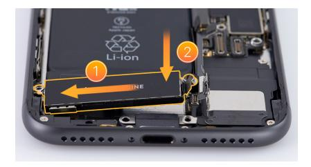
2. Use ESD-safe tweezers to grasp the grounding clip as shown and reinstall it into the enclosure. If the grounding clip is broken or bent, replace it with a new one.
