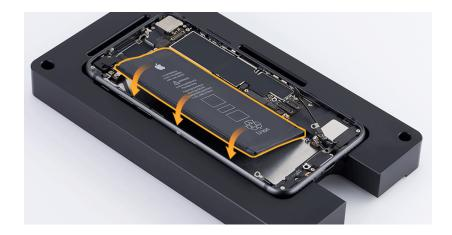
5. The repair tray has a slot in the center. Position the repair tray and enclosure into the battery press with the slot over the pin as shown.
