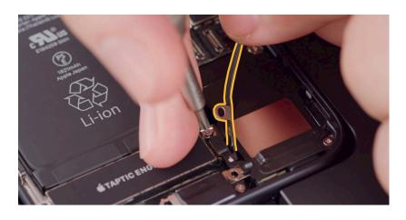
9. The Taptic Engine flex cable lies under the lower antenna flex cable. Use the black stick to gently lift the end of the lower antenna flex cable off the top of the Taptic Engine flex cable.
