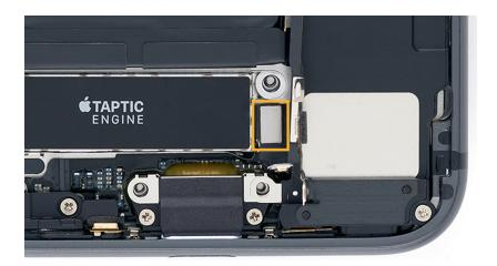
9. Adhere the end of the lower antenna flex cable to the top of the Taptic Engine flex cable.
