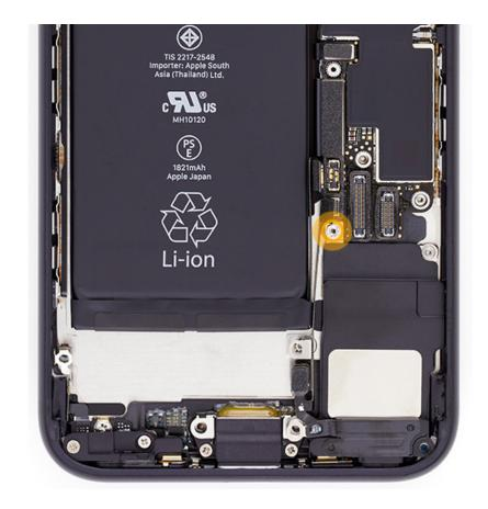
2. Use a torque driver and the super screw bit to remove the super screw from the speaker. Set aside the screw. 3. Gently insert the black stick under the lower right corner of the logic board (1). Lift the logic board just enough to slide the speaker under it and release the speaker from the speaker port (2). Lift the speaker out of the enclosure.
