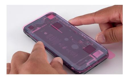
3. The replacement display adhesive has a top release liner, a middle release liner, and a bottom release liner. Grasp the tab on the bottom release liner. Then slowly pull the bottom release liner (1) out from under the adhesive (2) while pressing the adhesive onto the enclosure.
