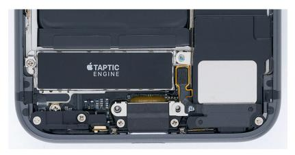
9. Press the upper end of the Wi-Fi antenna to the upper connector.
