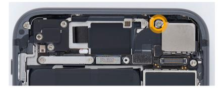
3. Remove the camera cowling and save it for reassembly.
