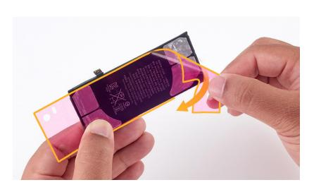
Rest the right edge of the battery in the enclosure.
