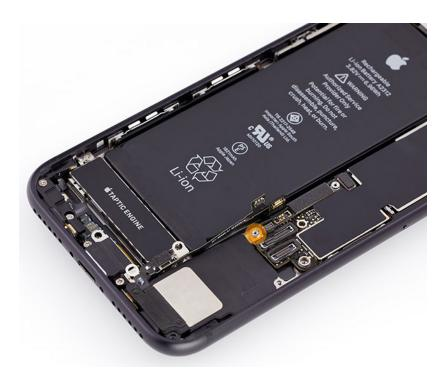
6. Use the green torque driver and JCIS bit to install two new crosshead screws into the speaker.
