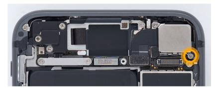
2. Use a torque driver and the super screw bit to remove the super screw from the camera cowling. Set aside the super screw.
