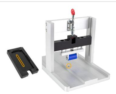
6. Flip down the red lever to lower the roller onto the battery.
