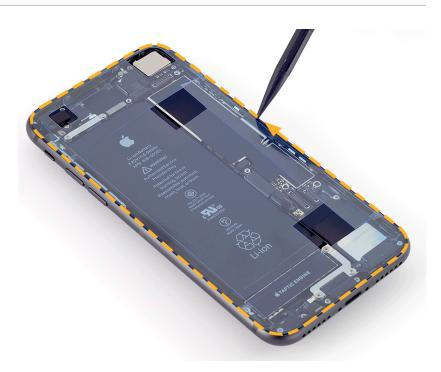
5. Remove the center section of the top release liner first (1). Then remove the three sections running along the top (2), right (3), and bottom (4).
