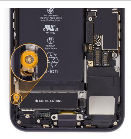
5. Use ESD-safe tweezers to remove the grounding clip. Save the grounding clip for reassembly.
