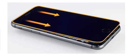
12. Insert the wheel of the adhesive cutter into the top of the iPhone between the display and the enclosure. Run the cutter around the top and sides of the iPhone until the display is free.
