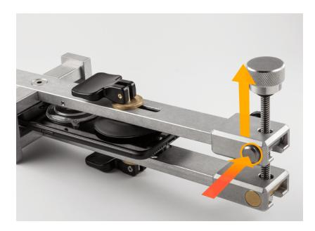
Slowly turn the knob on the adapter until the display begins to separate from the enclosure.
