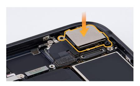
5. Use the green torque driver and super screw bit to partially install one new super screw into the camera cowling. Don't fully tighten the super screw yet.
