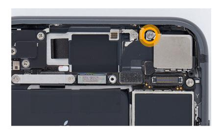
Use the green torque driver and JCIS bit to partially install one new crosshead screw into the camera cowling.
