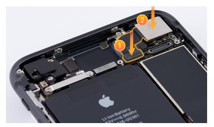
4. Position the camera cowling on the camera.
