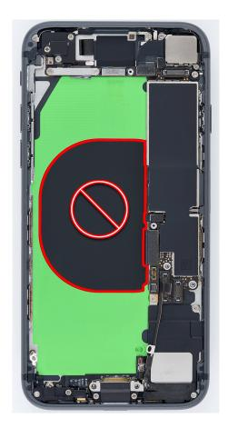
2. Peel the pink release liner from the underside of the replacement battery.
