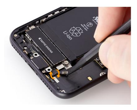
3. Ensure that the Taptic Engine/dock connector is parallel to the right side of the enclosure.
