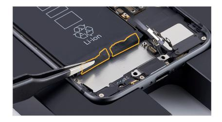
2. Hold down the iPhone with one hand. With the other hand, grasp one adhesive tab and slowly pull it toward the bottom of the iPhone. As the adhesive strip stretches, grasp it closer to the battery and continue pulling until you've removed the entire strip.
