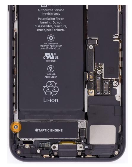
3. Use the green torque driver and JCIS bit to install one new crosshead screw into the Taptic Engine.
