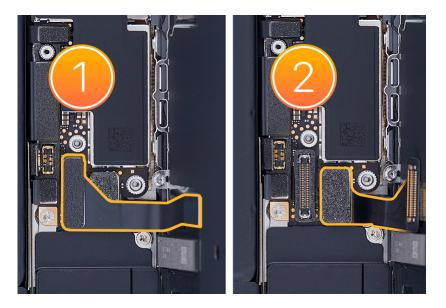
19. Use a torque driver and the JCIS bit to remove the three crosshead screws from the camera connector cowling. Set aside the screws.
