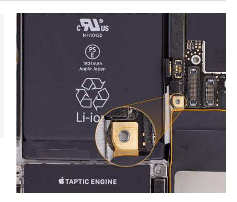
4. Insert the black stick under the lower right corner of the logic board. Tilt the top of the speaker down and slide it slightly under the logic board (1). Lay the bottom of the speaker in the enclosure. Then slide the bottom of the speaker into the speaker port (2).
