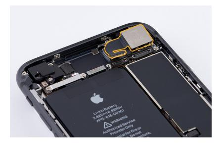
Press the end of the camera flex cable to the connector (1). Gently press the camera into the enclosure (2).
