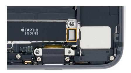
Adhere the end of the lower antenna flex cable to the top of the Taptic Engine flex cable.
