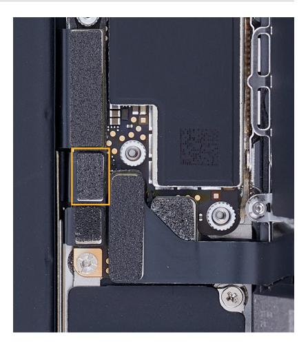
12. Press the end of the battery flex cable to the connector.
