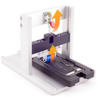
9. Remove the repair tray from the battery press.
