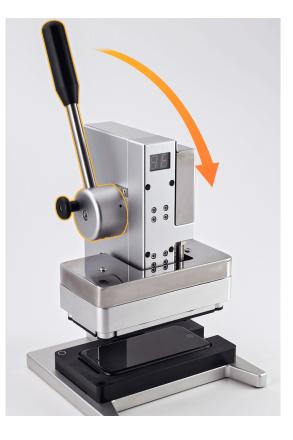
21. Wait until the timer on the display press beeps. Then hold down the lever (1), pull out the release knob (2), and lift up the lever (3).
