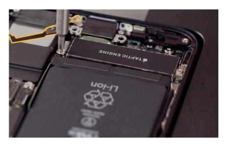
5. Inspect the Taptic Engine/ dock connector to ensure that it's attached to the coaxial connector on the enclosure.
