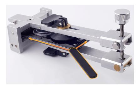
9. Press and hold the release button on the adapter to pull up the lever (1). Then flip the handles to release the two black suction cups (2). Pull the tabs on the clear suction cups to release the iPhone (3).
