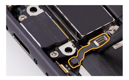
8. Press the end of the Taptic Engine flex cable to the Taptic Engine/dock connector.
