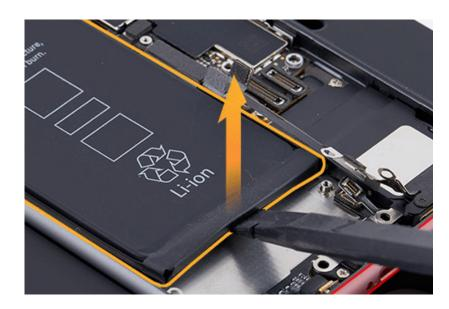
10. Remove the battery from the enclosure. Then inspect the enclosure for damage. If the enclosure is damaged, replace the iPhone.
