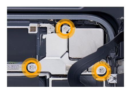
20. Remove the camera connector cowling and save it for reassembly.
