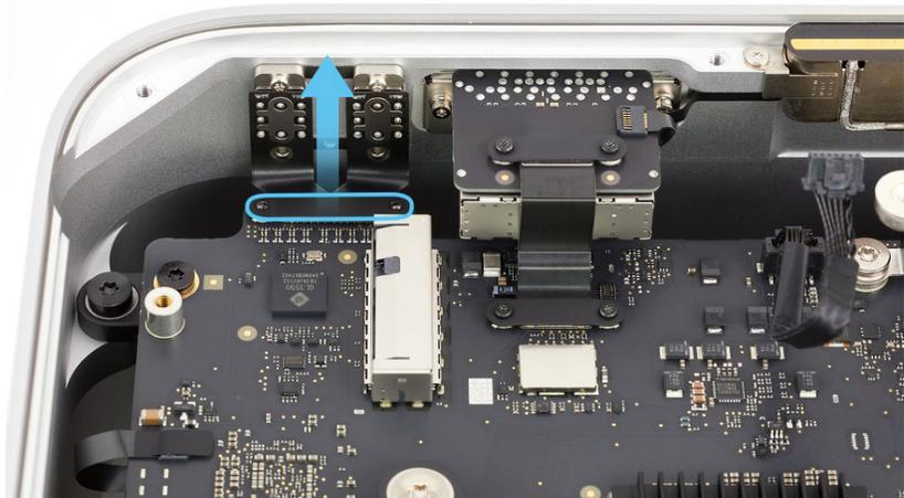
5. Use the flat end of the black stick to lift the end of the front USB-C flex cable off the connector.
