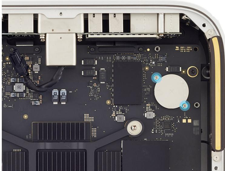
2. Lift the battery cover with the battery off the logic board.
