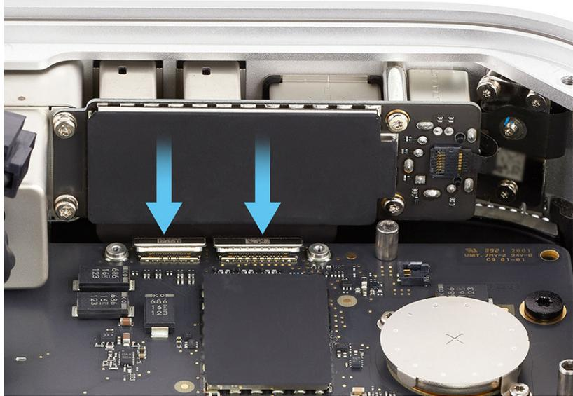
19. Position the combination I/O board connector cowling over the ends of the USB-A flex cable and HDMI flex cable. Then use the green torque driver and Torx T3 half-moon bit to reinstall the two T3 screws (923-07105) into the cowling.
