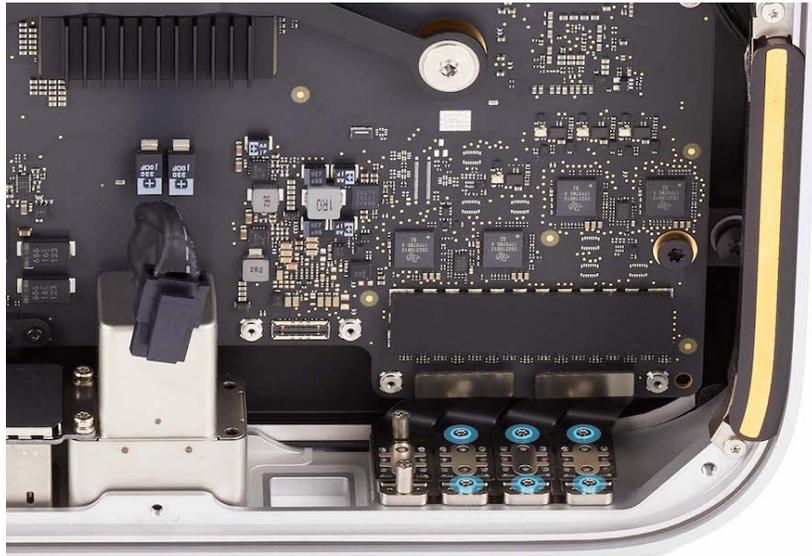
6. Use the T7 screwdriver to remove the two T7 standoff screws (923-07103) from the back Thunderbolt 4 ports.
