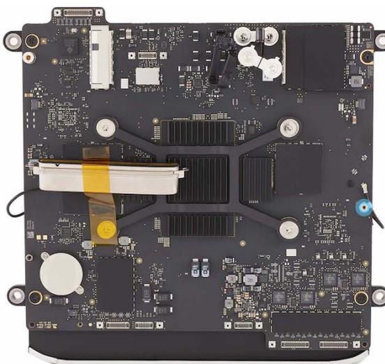
6. Use the blunt end of the antenna tool to press the end of the antenna coaxial cable to the connector.
