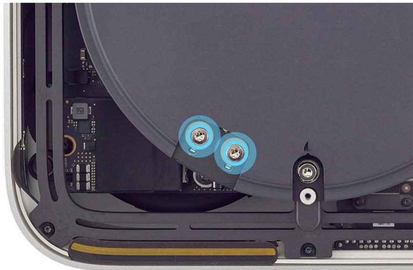
4. Use the adjustable torque driver and 10IP bit to remove the four 10IP screws (923-07096) from the power supply.
