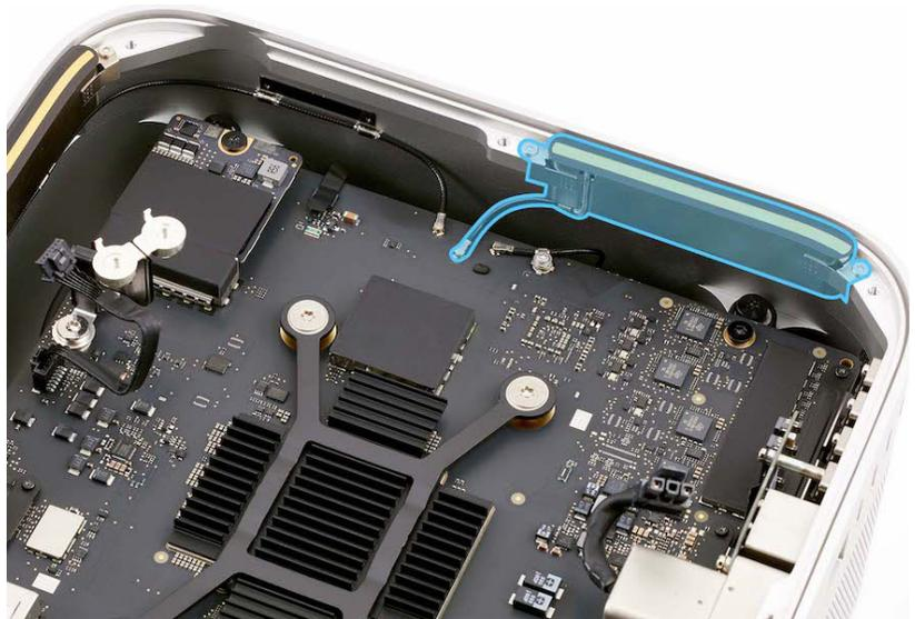
2. Use the antenna tool to lift the end of the antenna coaxial cable off the connector.
