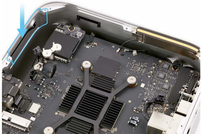
2. Insert the Torx T5 bit into the 10–34 Ncm adjustable torque driver. Set the torque value to 11.5 Ncm.
