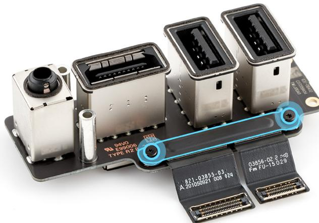
15. Use the black stick to lift the ends of the USB-A flex cable and HDMI flex cable off the connectors. Save the flex cables for reassembly.
