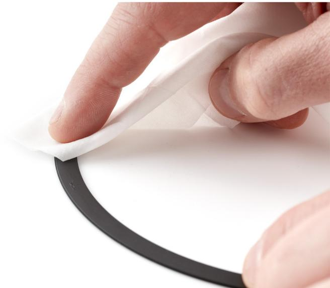
6. Use ESD-safe tweezers to pick up the adhesive on the bottom cover. Then pull the adhesive to remove it. Repeat this process until all the adhesive is removed from the bottom cover.
