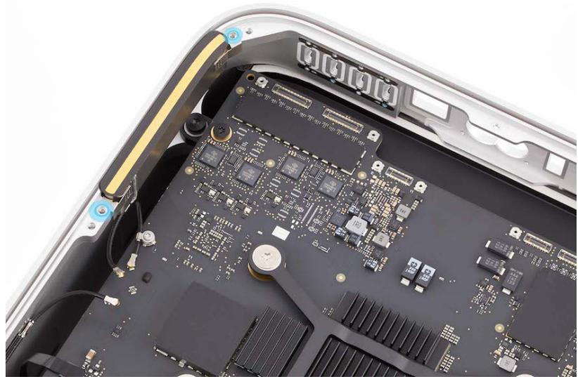
21. Use ESD-safe tweezers to position the ends of the two antenna coaxial cables over the connectors.
