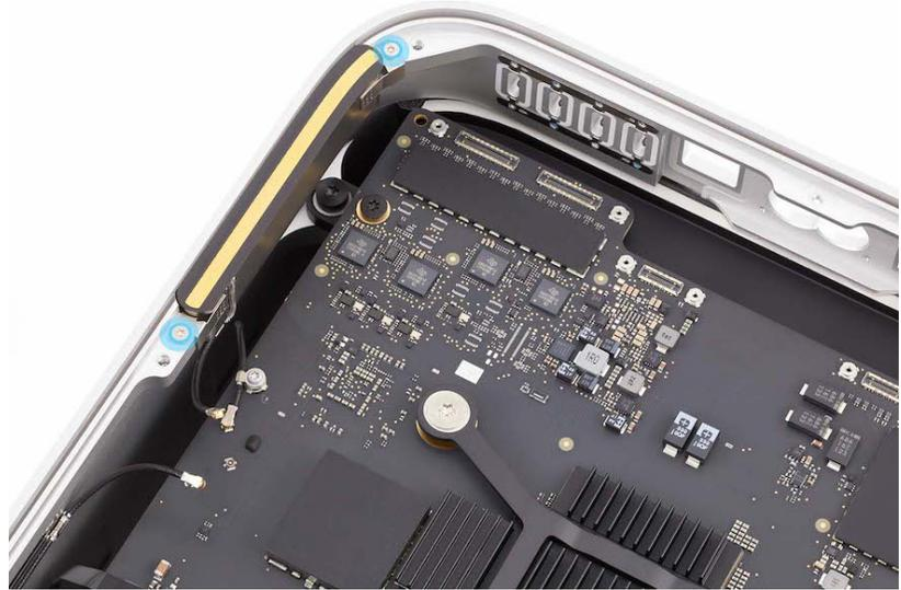
8. Lift antenna 2 out of the housing. Save antenna 2 for reassembly.
