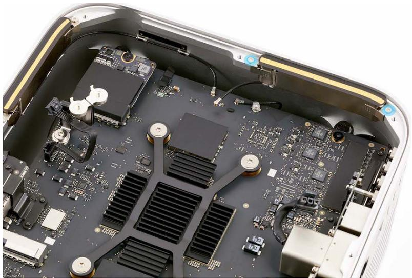
4. Lift antenna 2 out of the housing.
