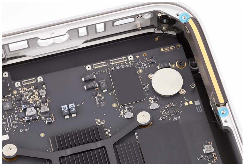
17. Use the black stick to press the antenna coaxial cable into the antenna coaxial cable grounding clips in the housing.
