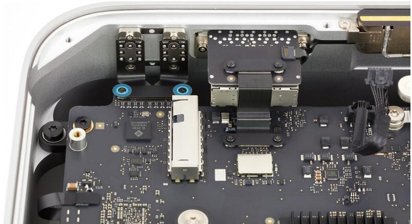
4. Remove the front USB-C ports connector cowling and save it for reassembly.
