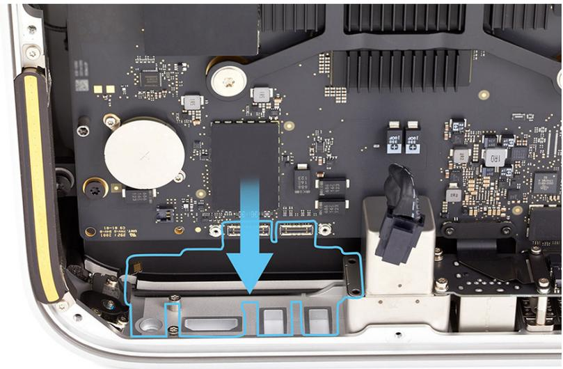
7. Use the T6 screwdriver to partially reinstall the two T6 screws (923-07100) into the combination I/O board.
