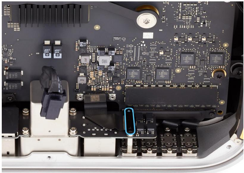
5. Use the T4 screwdriver to partially reinstall the two T4 screws (923-07099) into Ethernet board connector cowling 2.
