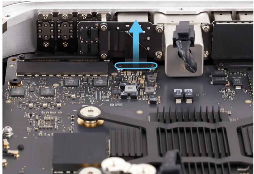
3. Use the black stick to lift the end of the Ethernet board flex cable off the connector on the logic board.
