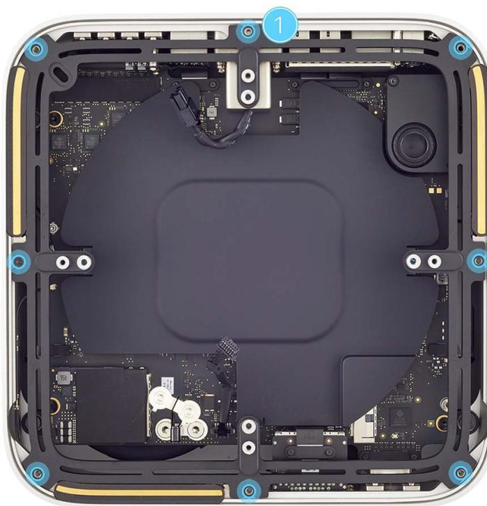
5. Insert the Torx T6 bit into the 10–34 Ncm adjustable torque driver. Set the torque value to 29.5 Ncm.
