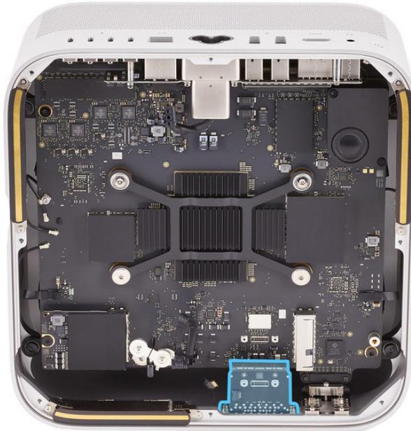
8. Use the T5 screwdriver to remove the two T5 screws (923-07109) from the SDXC card slot board.
