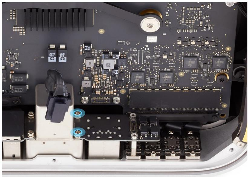
9. Lift the Ethernet board out of the housing.
