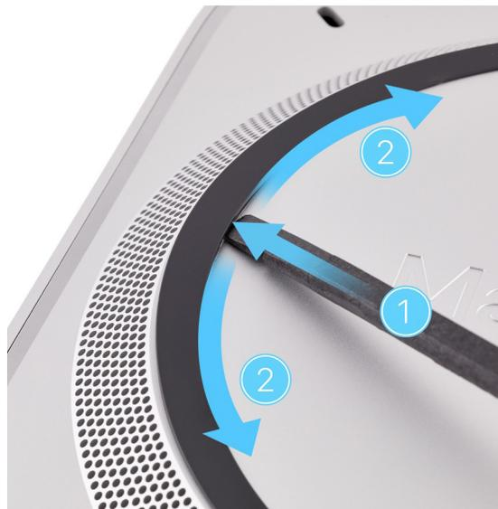
3. Remove the bottom cover screw pad from the bottom cover.
