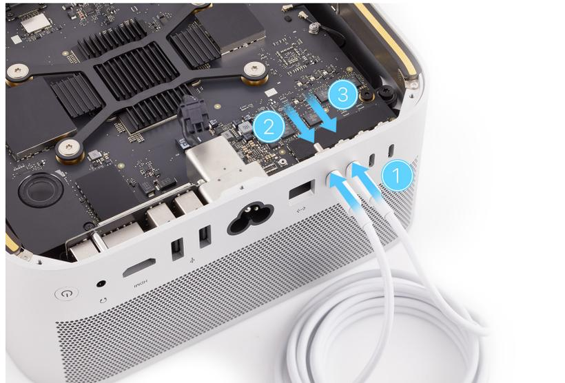
13. Press evenly along the length of each connector to ensure that they're fully connected to the logic board.
