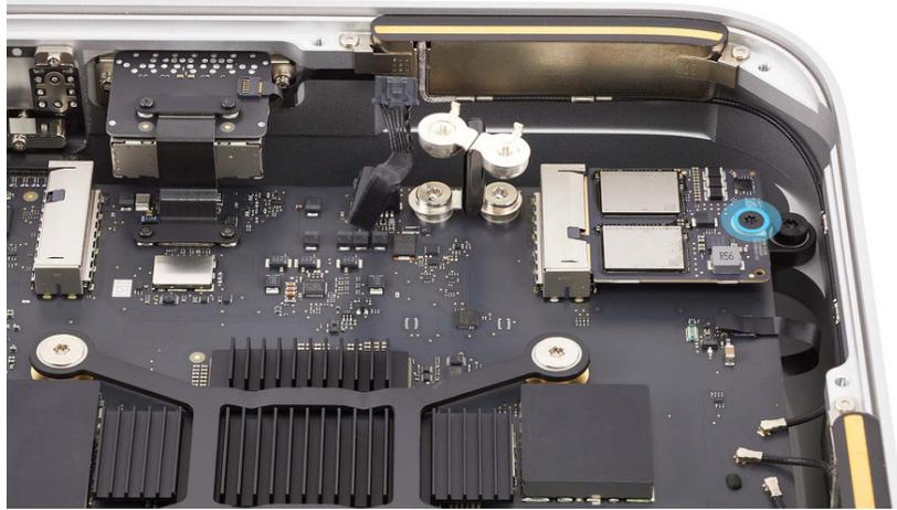
4. Grasp the sides of the SSD module and firmly pull it from the SSD module connector.
