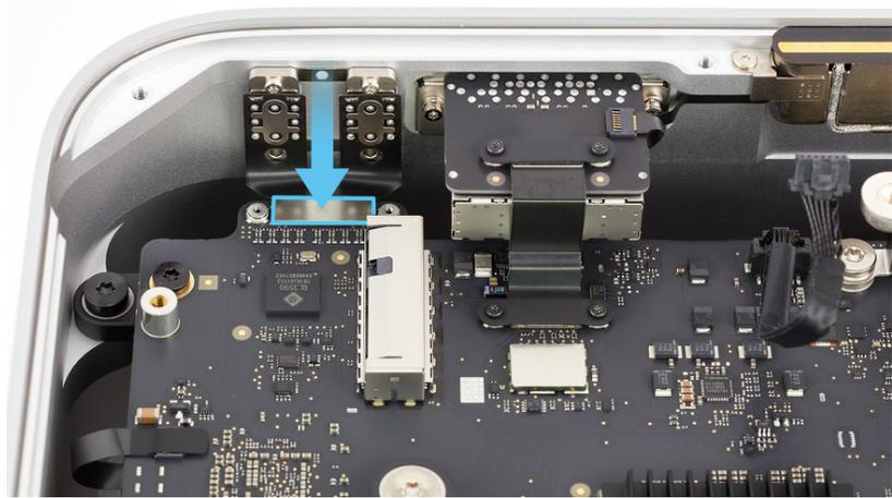
9. Position the front USB-C ports connector cawling over the end of the front USB-C flex cable.
