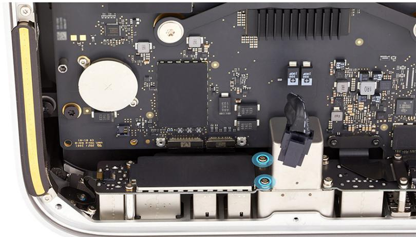
11. Lift the combination I/O board out of the housing.
