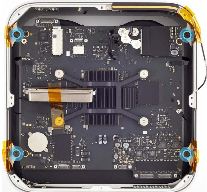
15. Tilt up the logic board as shown.
