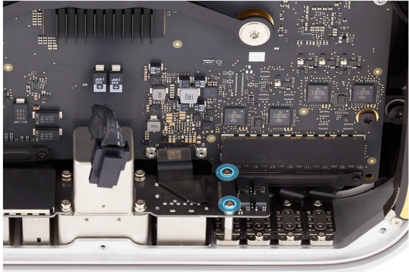
6. Remove Ethernet board connector cowl 2 and save it for reassembly.
