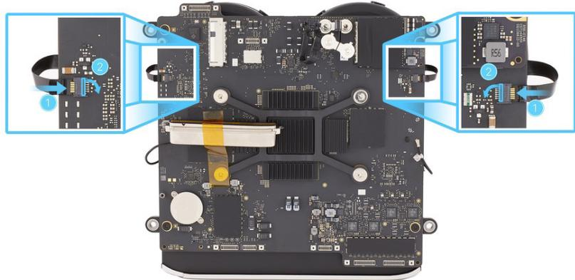
6. Press the polyester film tabs over the ends of the two fan flex cables.
