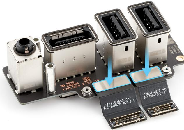
3. Position the second combination I/O board connector cowl over the connectors.
