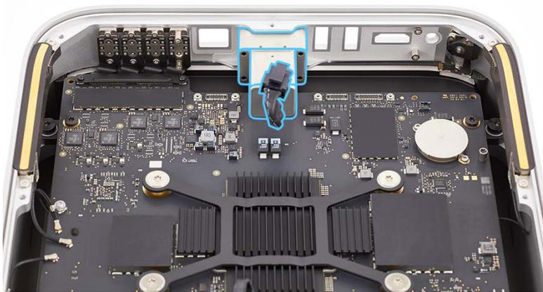
2. Reinstall the [combination input/output board](#) and [Ethernet board](#) to secure the power cord port in the housing.
