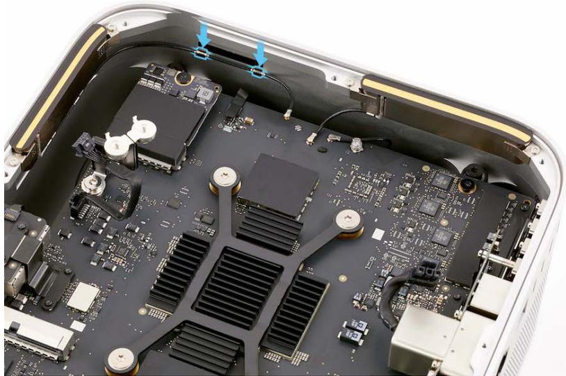
5. Use the blunt end of the antenna tool to press the end of the antenna coaxial cable to the connector.
