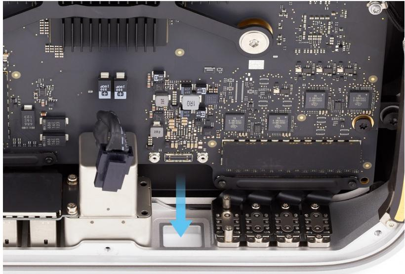
2. Use the T6 screwdriver to partially reinstall the two T6 screws (923-07100) into the Ethernet board.
