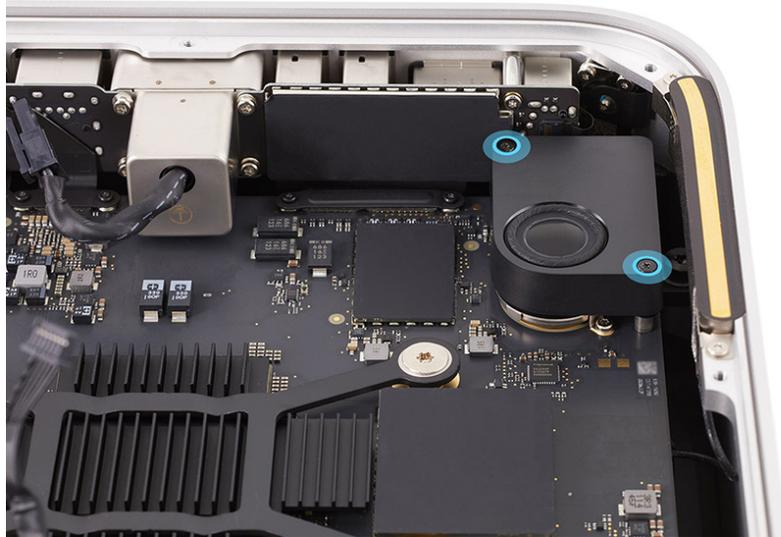
2. Slightly lift the speaker. Use the flat end of the black stick to lift the end of the speaker flex cable off the connector on the logic board.
