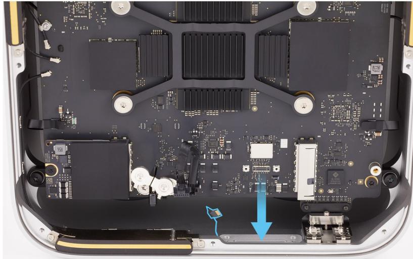
3. Use the T5 screwdriver to reinstall the two T5 screws (923-07109) into the SDXC card slot board.
