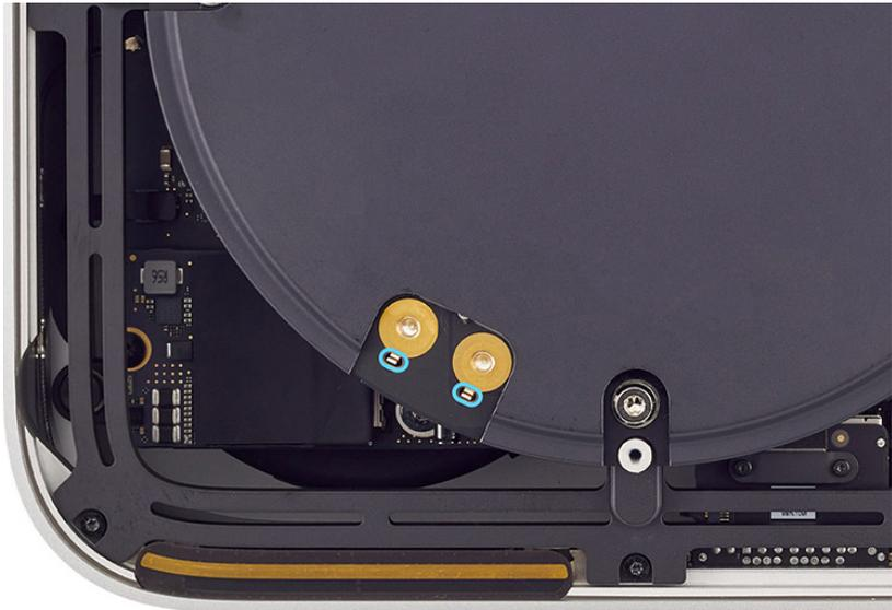
6. Keep the 10IP bit in the 0.3–1.2 Nm adjustable torque driver. Ensure that the torque value is still set to 0.7 Nm.
