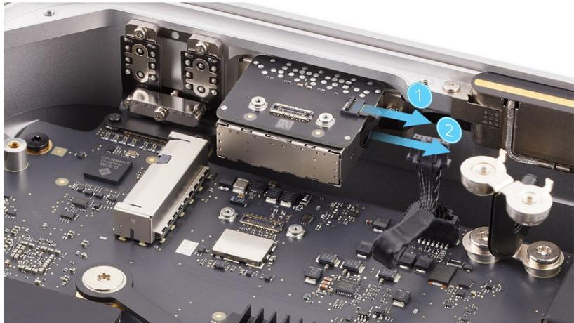
7. Stand the computer on its front with the back ports facing up.
