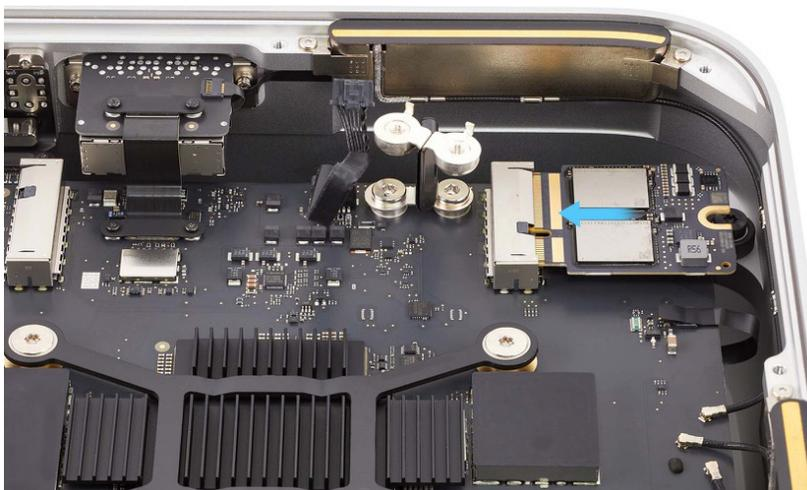
4. Use the T8 screwdriver to reinstall the T8 screw (923-02313) into the SSD module.
