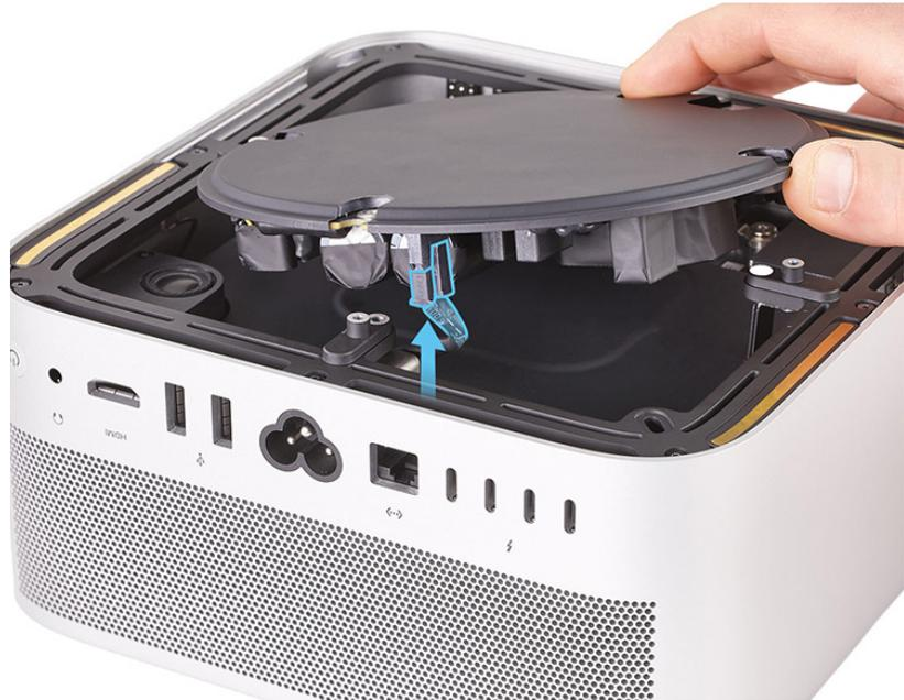
4. Rotate the computer so the front ports are facing you. Slightly tilt up the power supply. Slide the end of the power supply signal cable into the connector. Then tilt down the power supply onto the internal frame.
