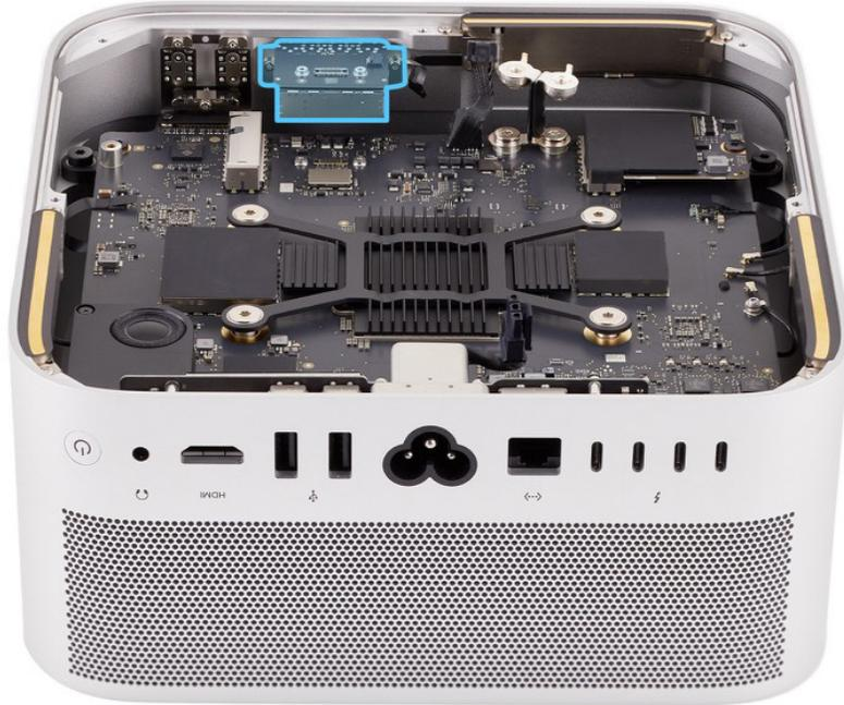
5. Slide the end of the status indicator light flex cable into the connector (1). Then flip down the locking lever (2). Press the status indicator light flex cable to adhere it to the side of the SDXC card slot board.
