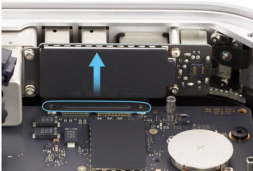
3. Use the black stick to lift the ends of the USB-A flex cable and HDMI flex cable off the connectors.
