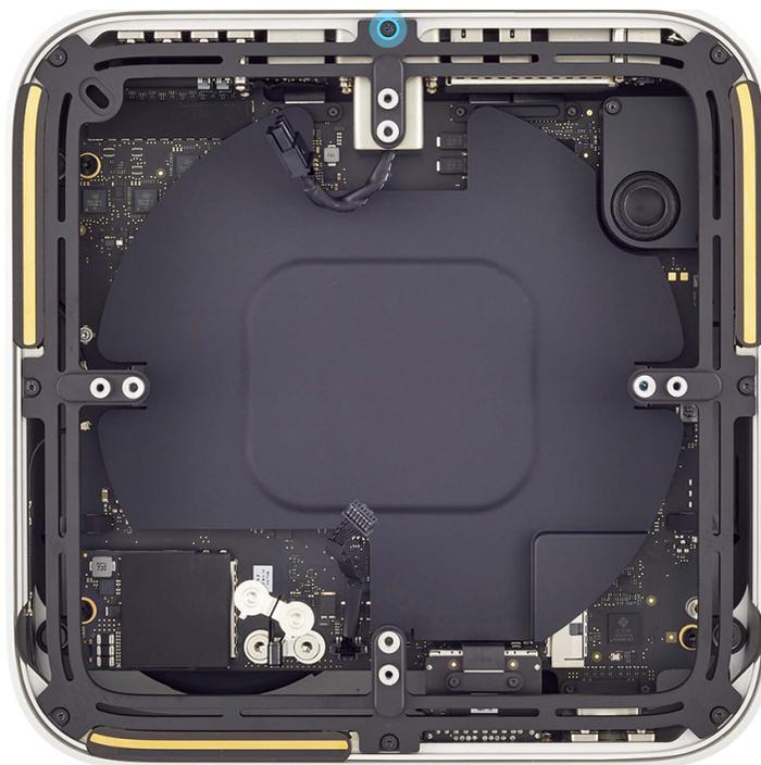
7. Remove the Torx T6 bit from the 10–34 Ncm adjustable torque driver. Insert the Torx T6 bit into the 0.3–1.2 Nm adjustable torque driver. Set the torque value to 0.6 Nm.
