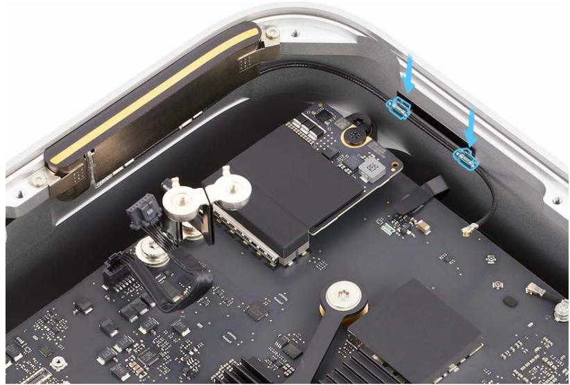
18. Rotate the computer so the front ports are facing you. Position antenna 2 in the housing.
