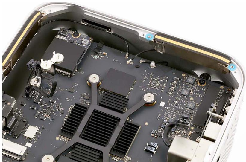
4. Use the blunt end of the antenna tool to press the end of the antenna coaxial cable to the connector.
