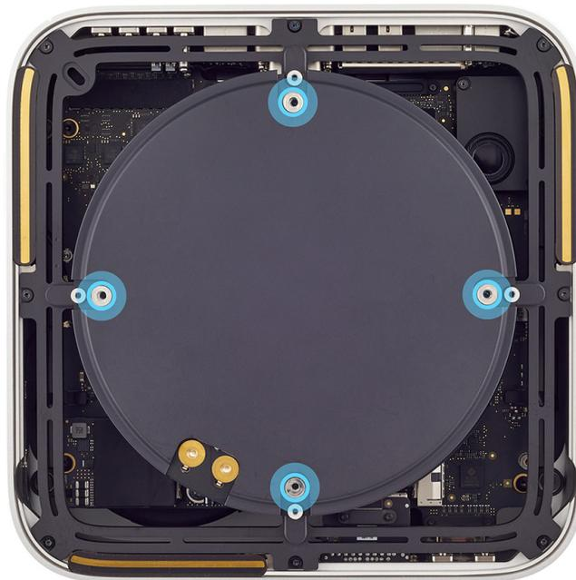
8. Keep the 10IP bit in the 0.3–1.2 Nm adjustable torque driver. Set the torque value to 0.6 Nm.
