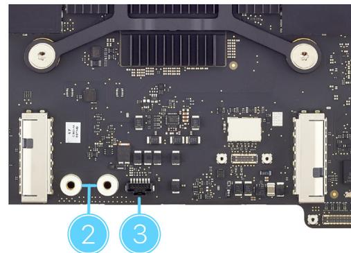
5. Insert one end of the power supply signal cable into the connector on the replacement logic board.
