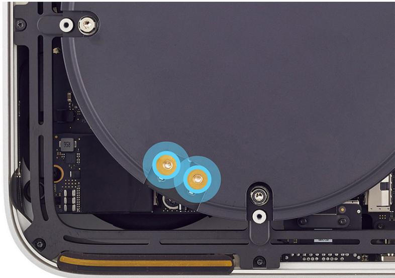
10. Adhere a replacement bus bar insulator cover over the two screws.
