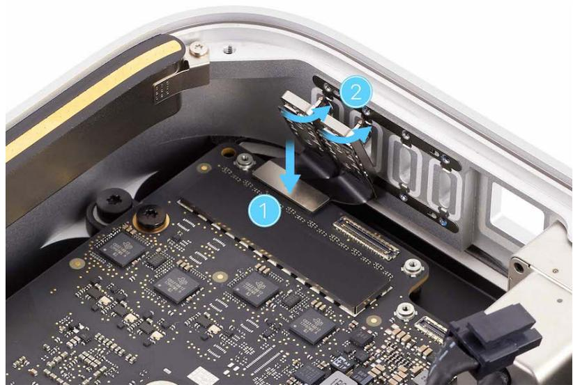
3. Position the back Thunderbolt 4 ports in the housing and press the end of the back Thunderbolt 4 ports flex cable to the connector (1). Then insert the back Thunderbolt 4 ports into the opening in the housing (2).
