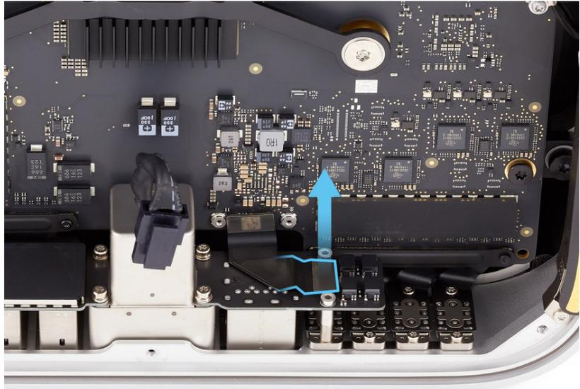
8. Use the T6 screwdriver to remove the two T6 screws (923-07100) from the Ethernet board and power cord port.
