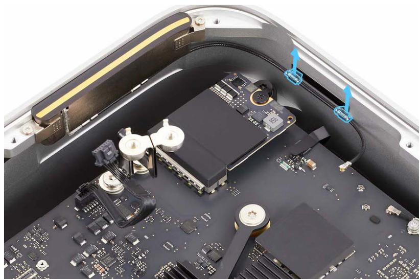
11. Use Kapton tape to secure the antenna coaxial cable to the housing.
