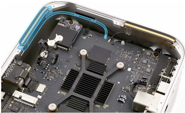
2. Use the antenna tool to lift the end of the antenna coaxial cable off the connector.
