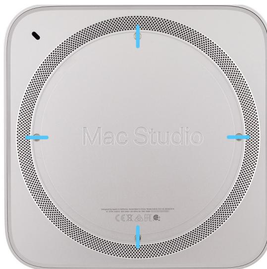
8. Peel the four release liners off the adhesive strips as you press the bottom cover screw pad to adhere it to the bottom cover.
