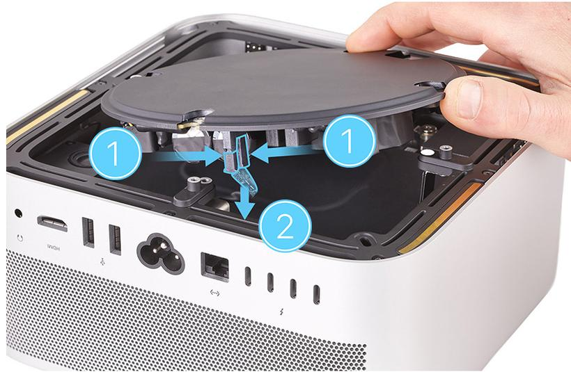
8. Lift the power supply off the internal frame and out of the housing.
