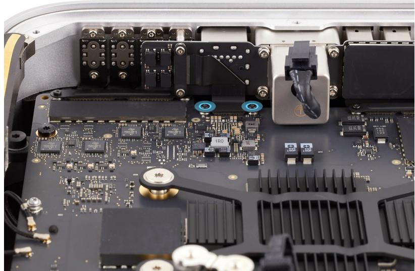
2. Remove Ethernet board connector cowling 1 and save it for reassembly.
