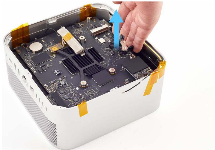
16. Continue to tilt up the logic board. Slide it slightly toward the front of the housing until you see a gap between the back of the housing and the logic board (1). Ensure that the antenna coaxial cable (2) and fan flex cables (3) are free of the housing.
