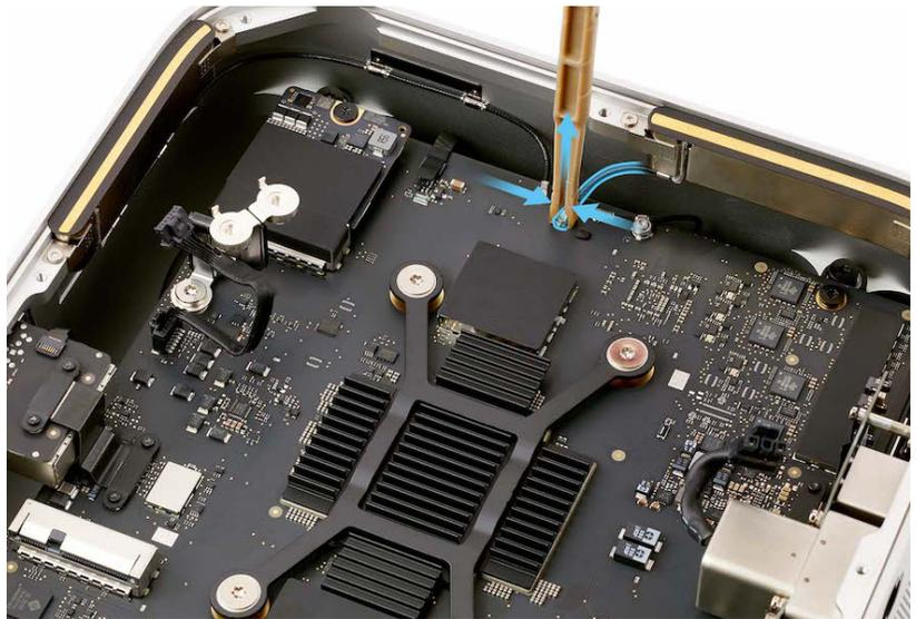
3. Use the T5 screwdriver to remove the two T5 screws (923-07101) from antenna 2.
