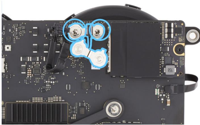
21. Remove the bus bar and save it for reassembly.
