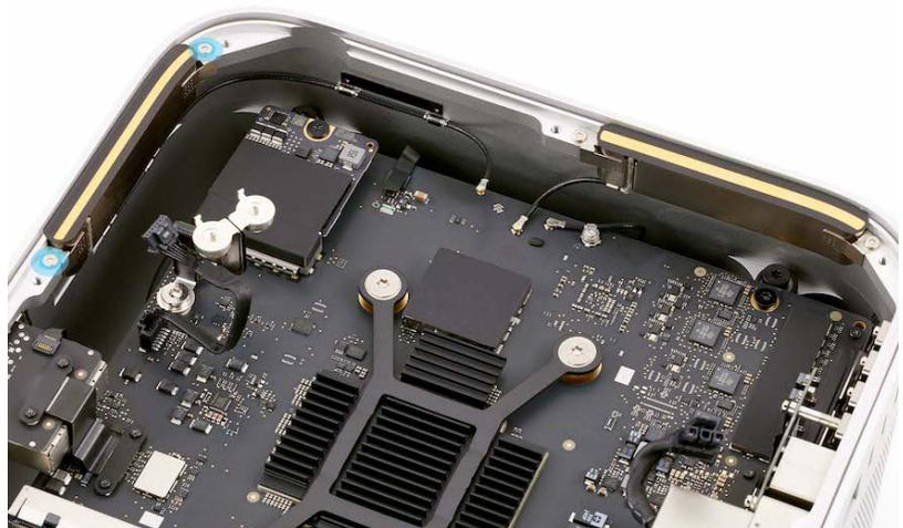
5. Lift antenna 3 out of the housing.
