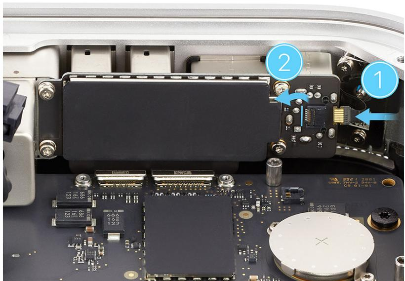
18. Press the ends of the combination I/O board flex cables to the connectors.
