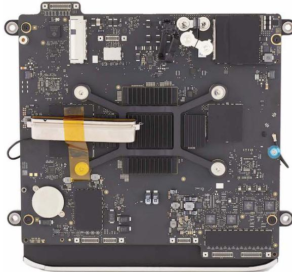
3. Use the antenna tool to lift the end of the antenna coaxial cable off the connector.
