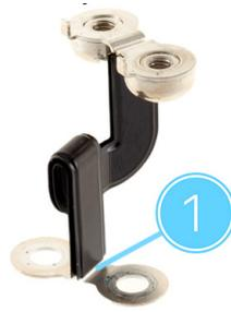
4. Use the adjustable torque driver and 10IP bit to reinstall the two 10IP screws (923-07098) into the bus bar and replacement logic board.
