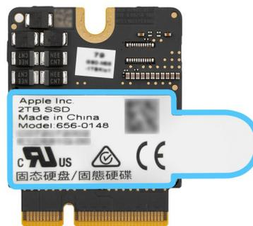
2. Each SSD module has a serial number that ends in 00 or 01. Identify the corresponding SSD module connector for the SSD module.
