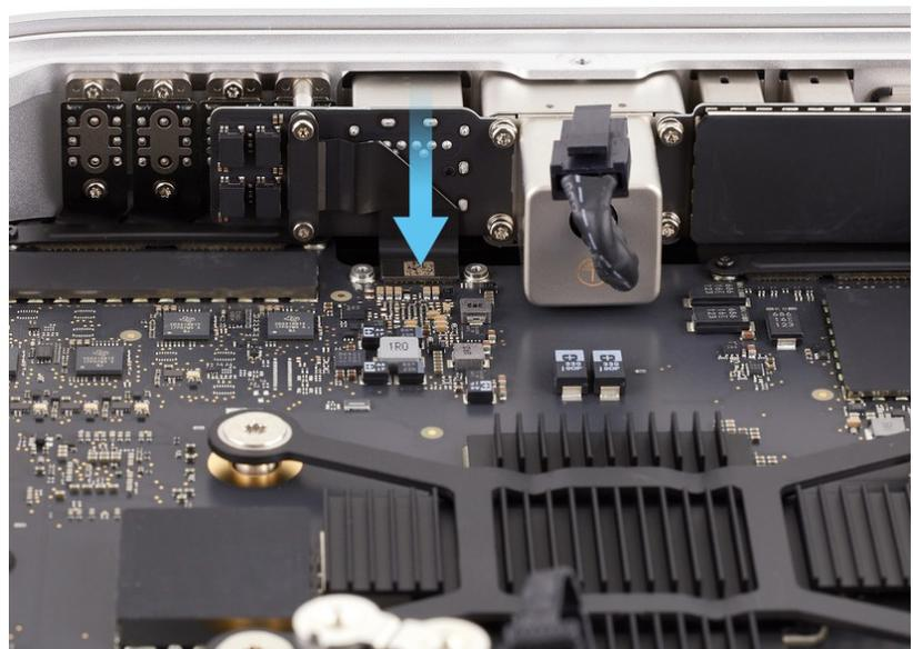
12. Position Ethernet board connector cawling 1 over the end of the Ethernet board flex cable.
