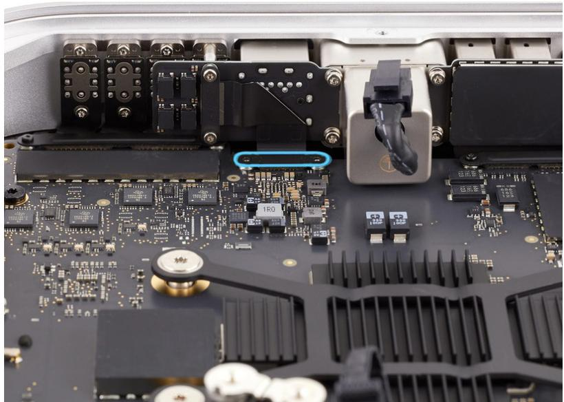
13. Use the green torque driver and Torx T3 half-moon bit to reinstall the two T3 screws (923-07105) into the cawling.
