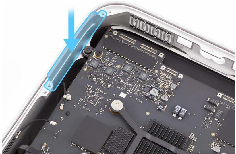
19. Insert the Torx T5 bit into the 10–34 Ncm adjustable torque driver. Set the torque driver to 11.5 Ncm.
