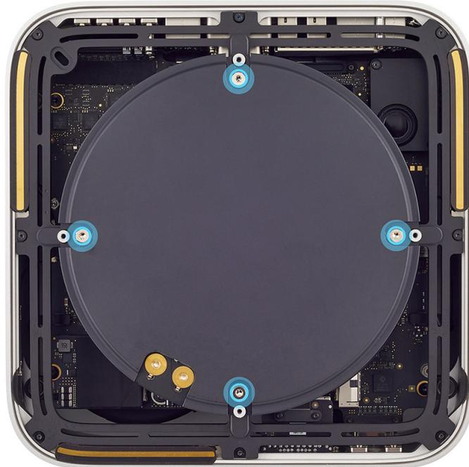
5. Slightly tilt up the power supply. Pinch the end of the power supply signal cable. Pull the end of the power supply signal cable to slide it out of the connector. Then tilt down the power supply onto the internal frame.
