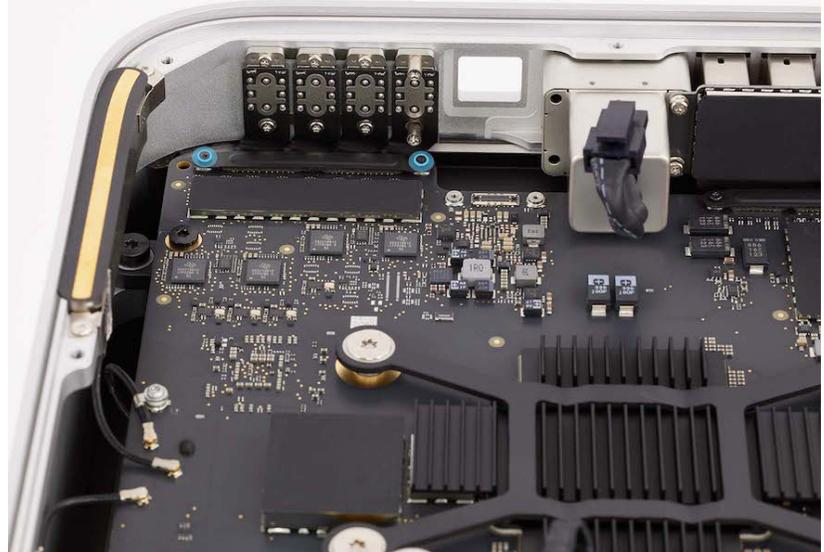
2. Remove the cowling and save it for reassembly.
