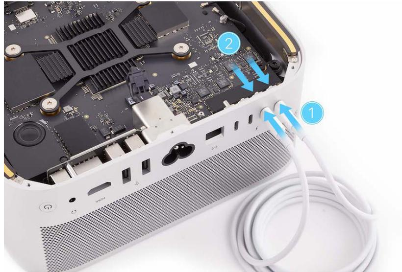
10. Plug both ends of the USB-C charge cable into two back Thunderbolt 4 ports (1) as shown to ensure back Thunderbolt 4 ports alignment. Adjust the alignment of the ports until both ends of the USB-C cable are easy to insert and remove.
