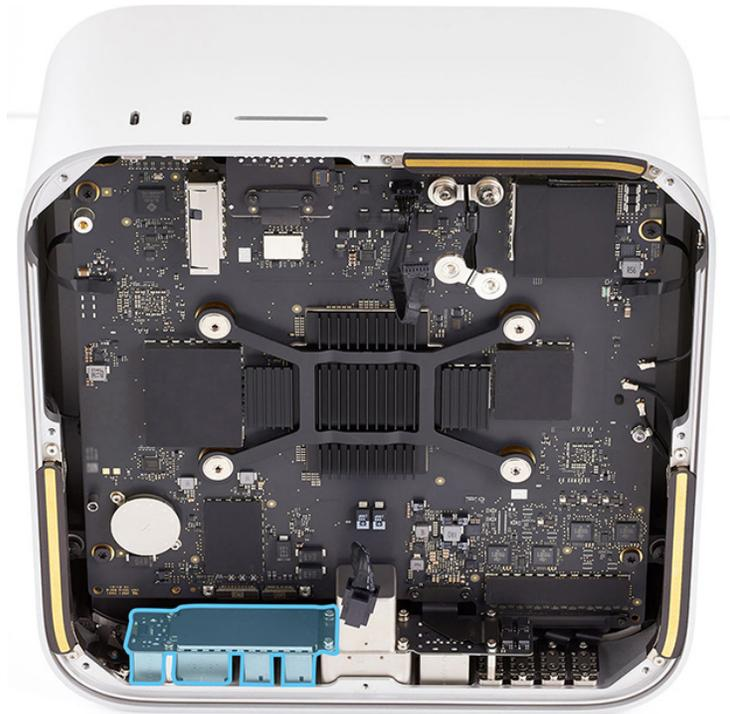
9. Use the T4 screwdriver to remove the two T4 screws (923-07111) from the combination I/O board.
