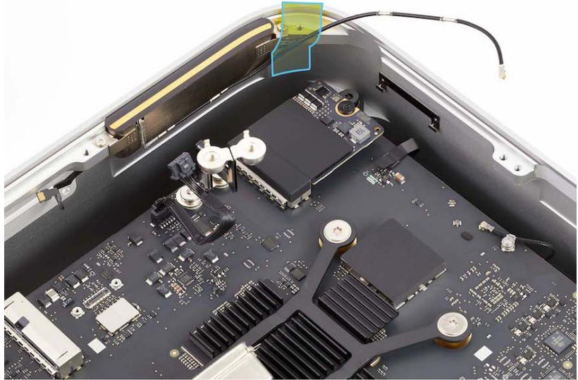
12. Apply Kapton tape inside the housing near the four logic board screws to avoid damaging the housing.
