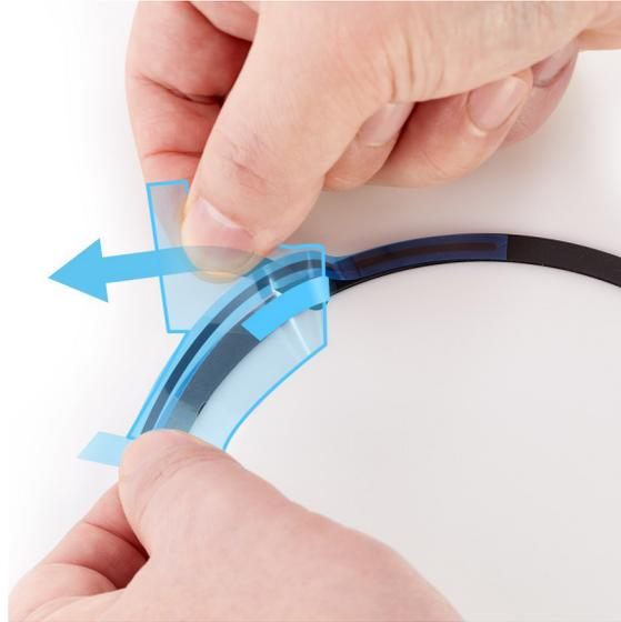
6. Gently run the flat end of the black stick along the length of the adhesive strips to adhere them to the bottom cover screw pad.
