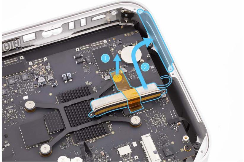
15. Insert the Torx T5 bit into the 10–34 Ncm adjustable torque driver. Set the torque driver to 11.5 Ncm.
