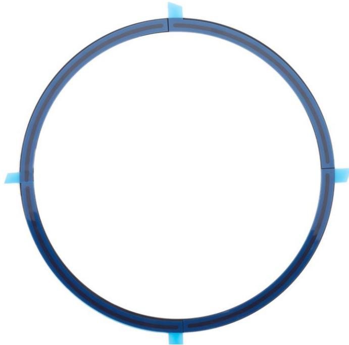
7. Position the bottom cover screw pad in the channel of the bottom cover with the flat side of the bottom cover screw pad facing up. Align the four release liner tabs with the four screws on the bottom cover.
