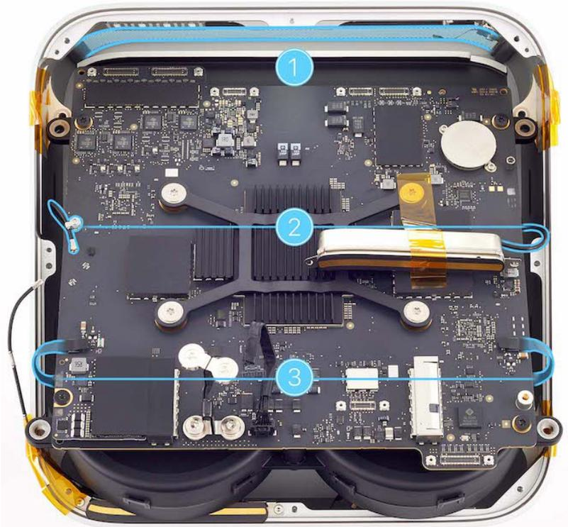
17. Hold the logic board by the edges until the fan is above the edge of the housing. Then support the logic board from under the fan and lift the logic board and fan out of the housing.
