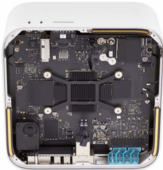
5. Use the T5 screwdriver to remove the six T5 screws (923-07093) from the back Thunderbolt 4 ports.
