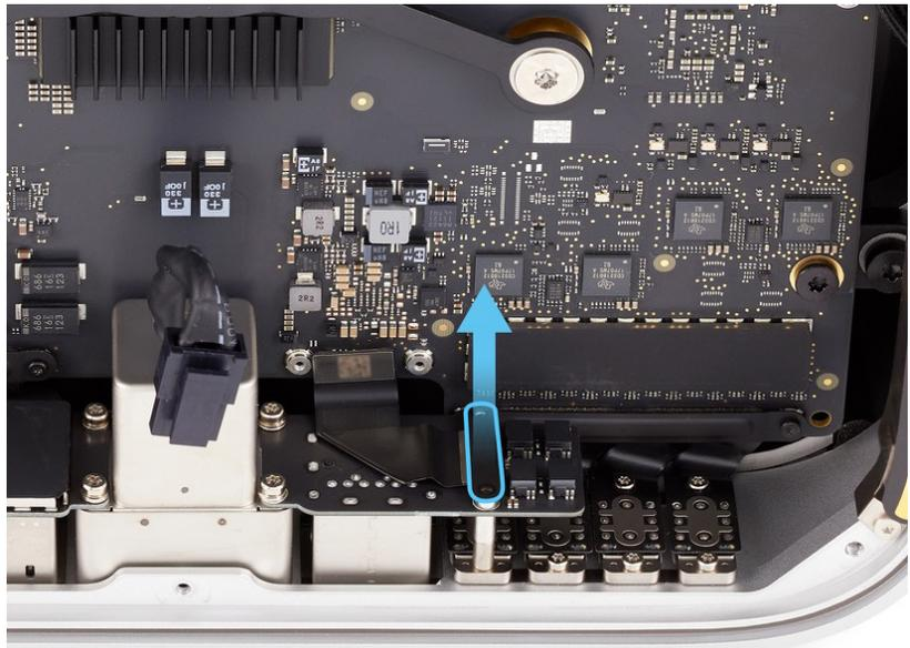
7. Use the black stick to lift the end of the Ethernet board flex cable off the connector on the Ethernet board.
