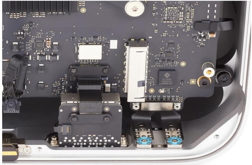
8. Lift the front USB-C ports out of the housing.
