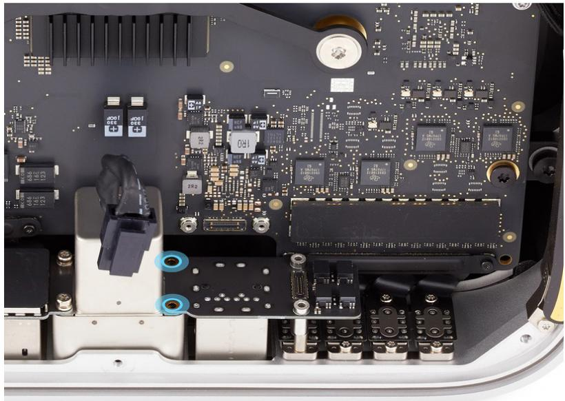
3. Press the end of the Ethernet board flex cable to the connector on the Ethernet board.
