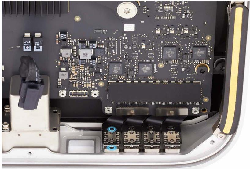
6. Use the T5 screwdriver to partially reinstall the six T5 screws (923-07093) into the back Thunderbolt 4 ports.
