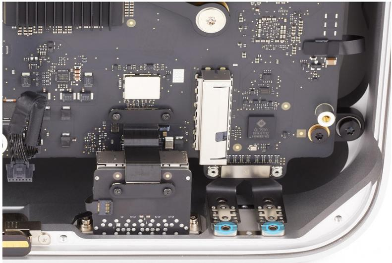
3. Align the two pins on the front USB-C bracket with the two holes in the front USB-C ports. Use the T5 screwdriver to partially reinstall the captive T5 screw on the bracket.
