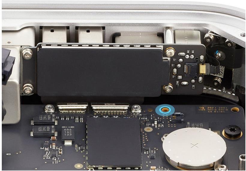
16. Slide the end of the power button flex cable into the connector (1). Then flip down the locking lever (2).
