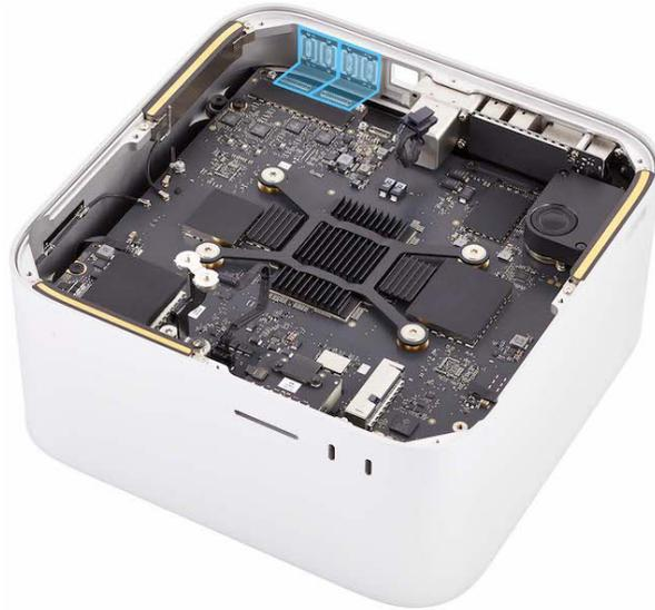
2. Position the back Thunderbolt 4 ports in the housing and press the end of the back Thunderbolt 4 ports flex cable to the connector (1). Then insert the back Thunderbolt 4 ports into the opening in the housing (2).
