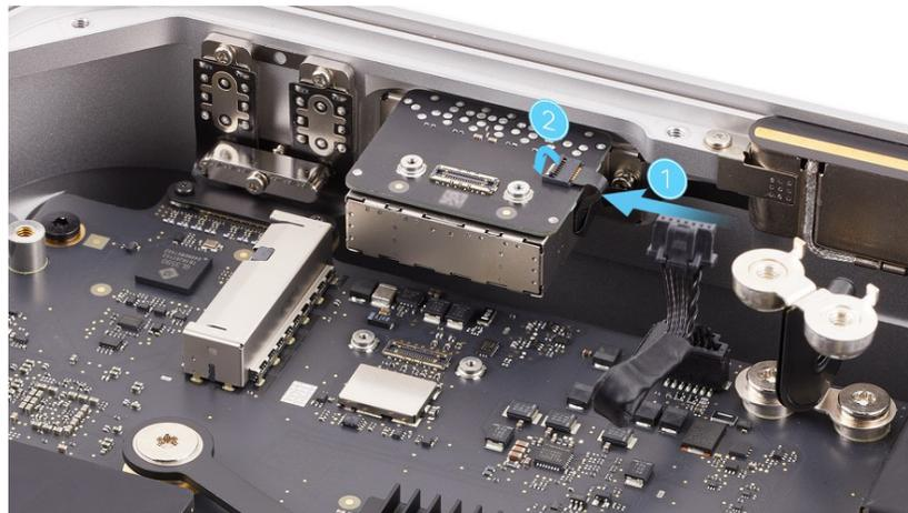
6. Position the ends of the SDXC card slot board flex cable over the connectors. Press the ends of the flex cable to the connectors.
