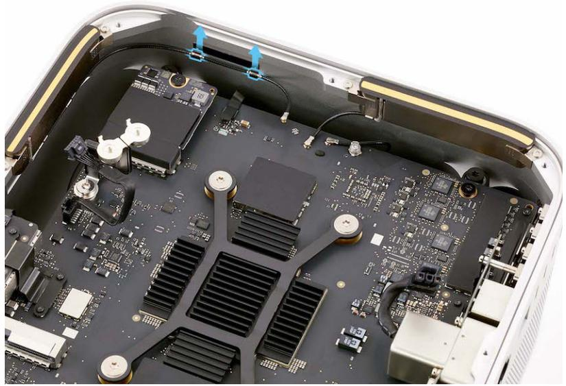
4. Use the T5 screwdriver to remove the two T5 screws (923-07101) from antenna 3.
