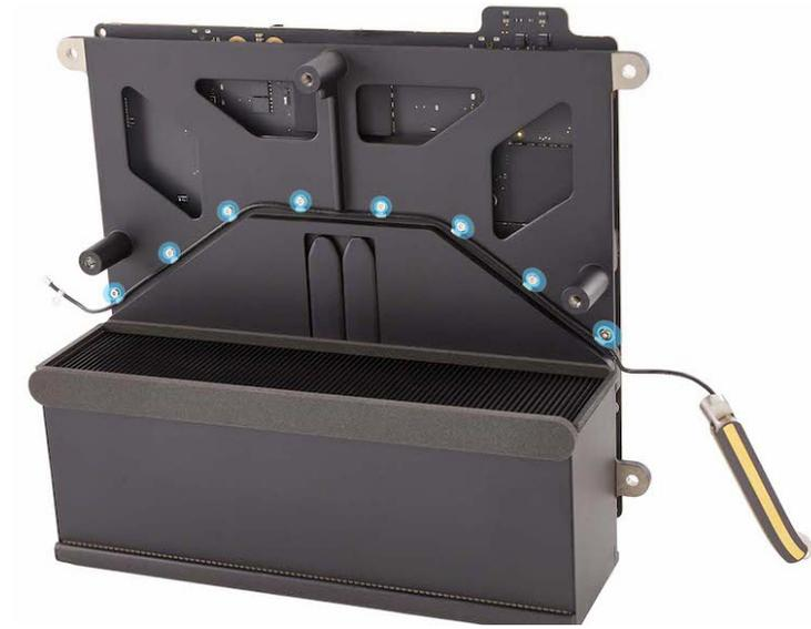
5. Remove antenna 1 from the logic board.
