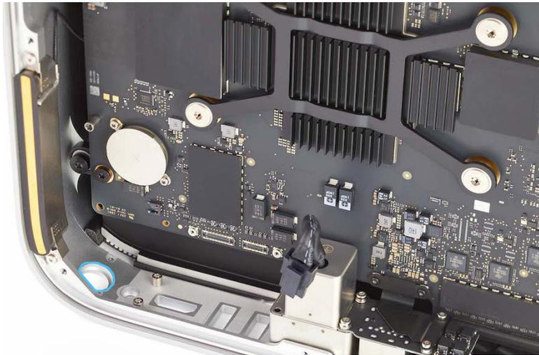
2. Use the T3 screwdriver to reinstall the three T3 screws (923-07541) into the power button.
