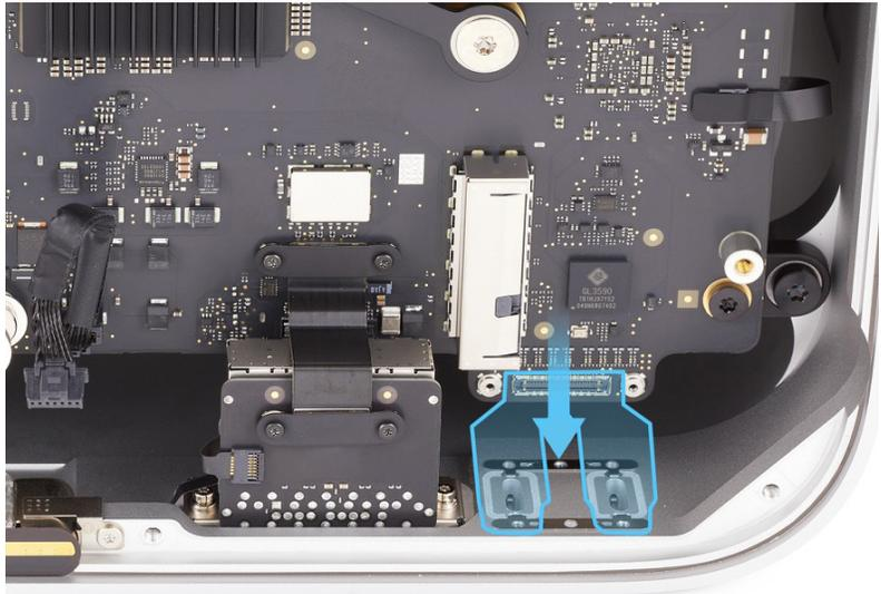
2. Use the T5 screwdriver to partially reinstall the two T5 screws (923-07093) into the front USB-C ports.
