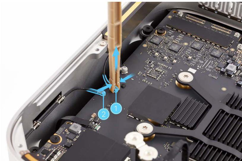
6. Keep the Torx T5 bit in the 10–34 Ncm adjustable torque driver. Set the torque value to 11.5 Ncm.
