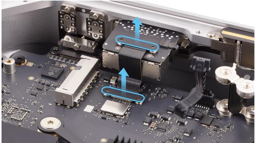
4. Use the black stick to lift both ends of the SDXC card slot board flex cable off the connectors.
