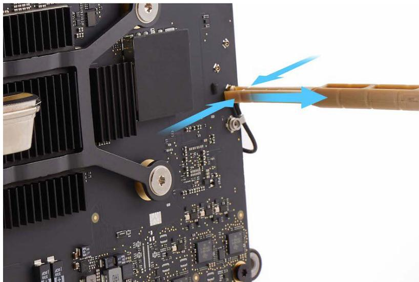
4. Rotate the logic board to access the other side. Use the T5 screwdriver to remove the eight T5 screws (923-07102) from the antenna coaxial cable routing clips.
