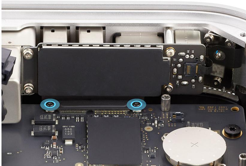
2. Remove the combination I/O board connector cowl and save it for reassembly.
