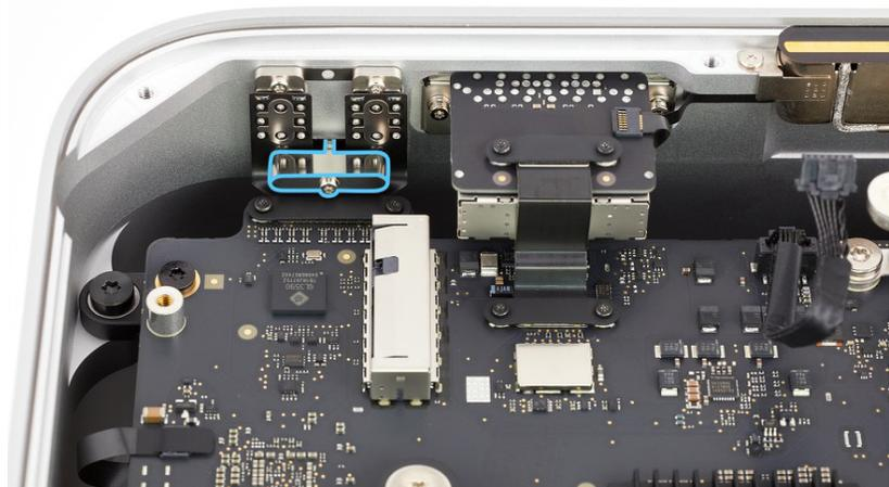
3. Use the T3 screwdriver to remove the two T3 screws (923-07105) from the front USB-C ports connector cowling.
