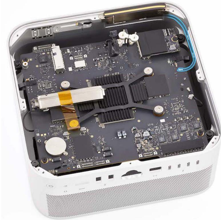
10. Lift the antenna coaxial cable out of the antenna coaxial cable grounding clips in the housing.
