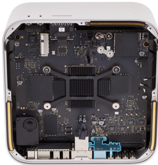
5. Use the T4 screwdriver to remove the two T4 screws (923-07099) from Ethernet board connector cowl 2.
