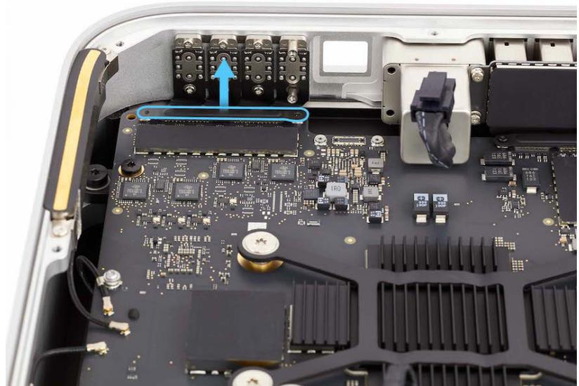
3. Use the black stick to lift the ends of the back Thunderbolt 4 ports flex cables off the connectors.
