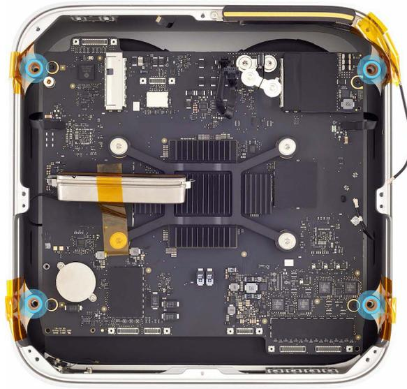
12. Remove the Kapton tape from the housing and the antenna coaxial cable.
