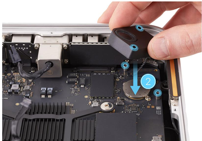
4. Insert the Torx T5 bit into the 10–34 Ncm adjustable torque driver. Set the torque value to 13 Ncm.
