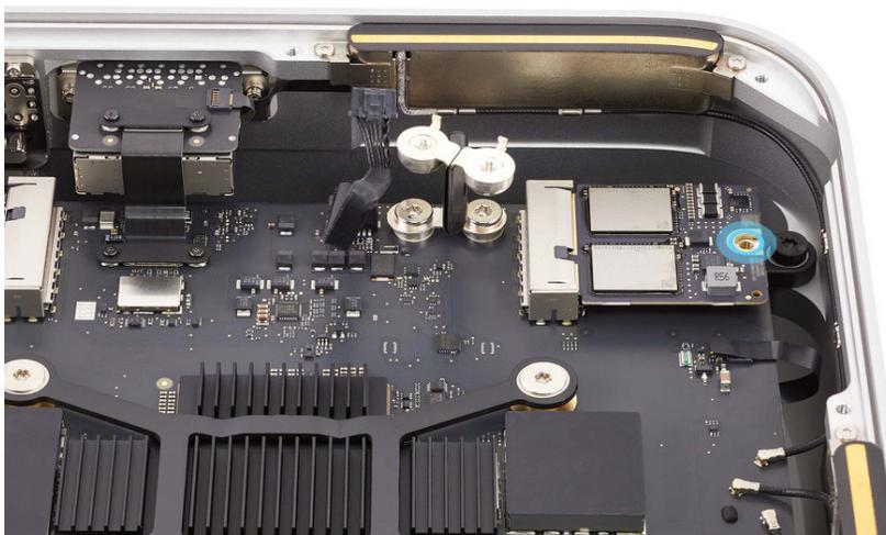
5. If you're reinstalling the existing SSD module, skip to reassembly step 6. If you're installing a replacement SSD module, peel a replacement SSD module cover from the adhesive backing.
