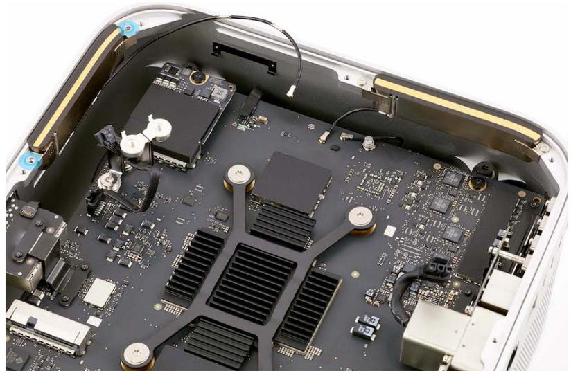
4. Use the black stick to press the antenna coaxial cable into the antenna coaxial cable grounding clips in the housing.
