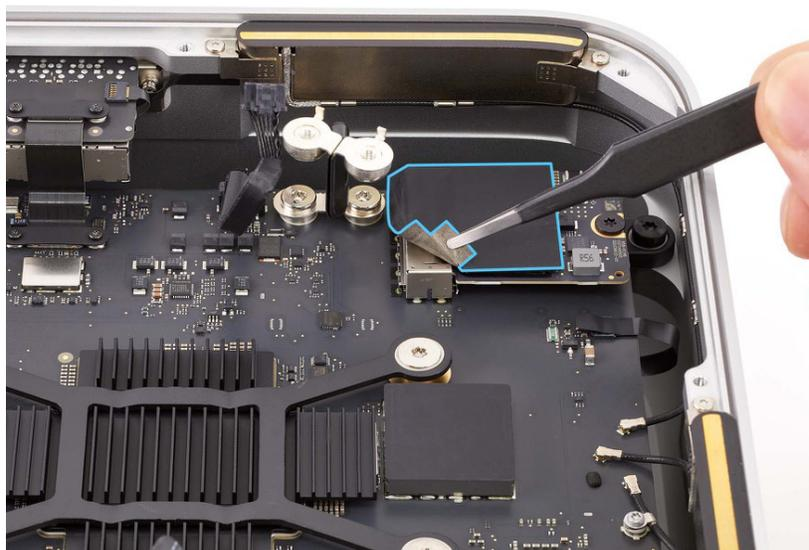
3. Use the T8 screwdriver to remove the T8 screw (923-02313) from the SSD module.
