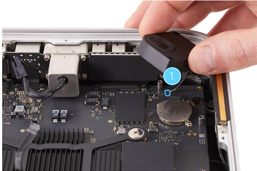
3. Align the screw holes in the speaker with the two speaker standoff screws on the logic board (2).
