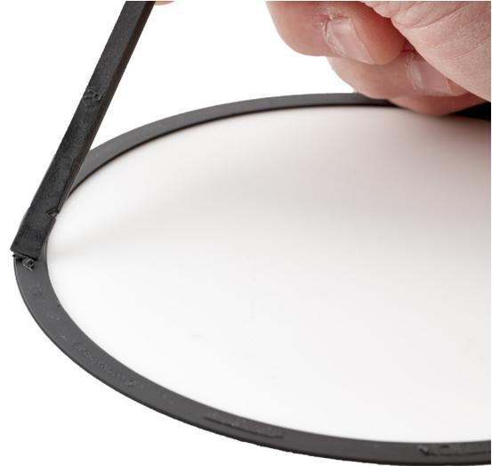
5. Use ethanol wipes or IPA wipes to clean any adhesive residue from the underside of the bottom cover screw pad. Save the bottom cover screw pad for reassembly.
