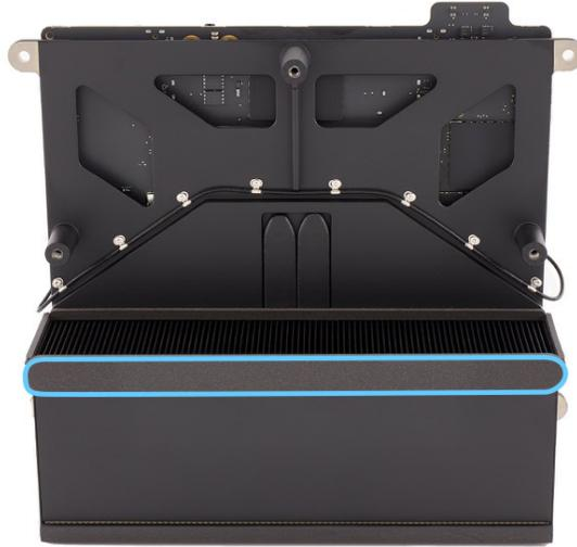
2. Insert the Torx T10 bit into the 0.3–1.2 Nm adjustable torque driver. Set the torque value to 0.95 Nm.
