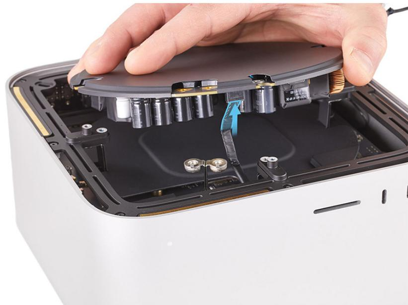
5. Ensure that the two pins on the bus bar are aligned with the two alignment holes in the power supply.
