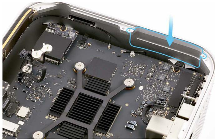
2. Insert the Torx T5 bit into the 10–34 Ncm adjustable torque driver. Set the torque value to 11.5 Ncm.
