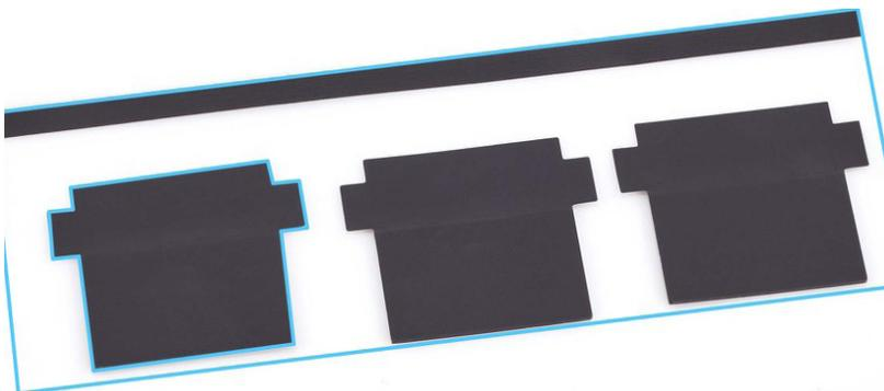
6. Position the SSD module cover over the SSD module and connector as shown. Then fold the three polyester film tabs over the edges of the SSD module connector. Press the tabs onto the sides of the connector.
