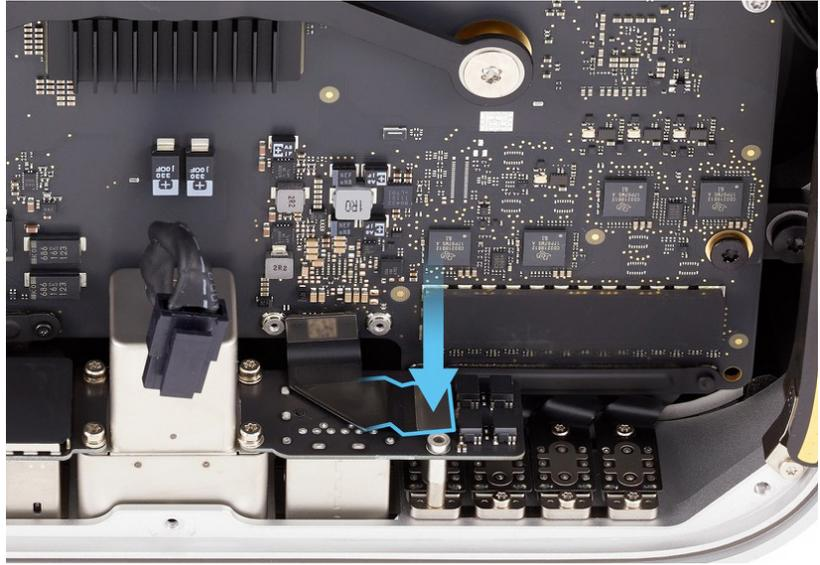
4. Position Ethernet board connector cowl 2 over the connector.
