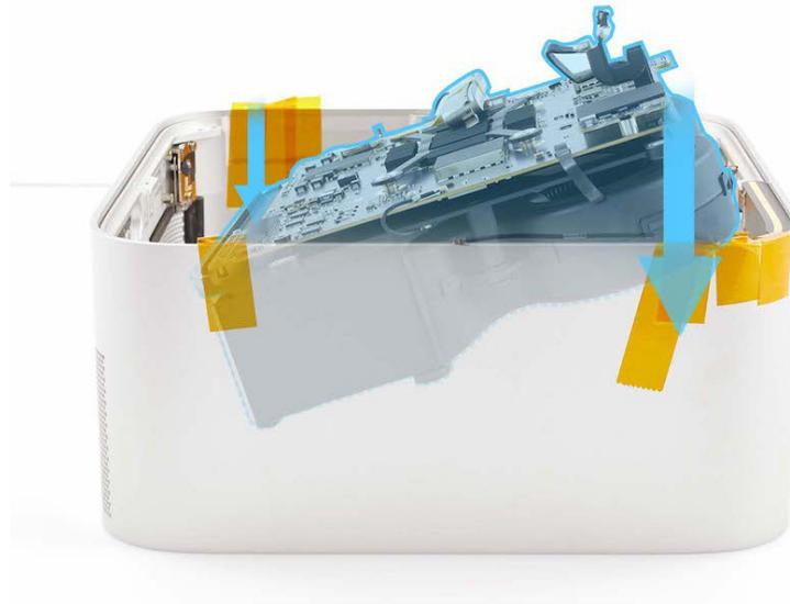
9. Continue to tilt down the logic board (1) and slide it toward the back of the housing (2). After the fan is below the edge of the housing, slide the logic board fully toward the back of the housing.
