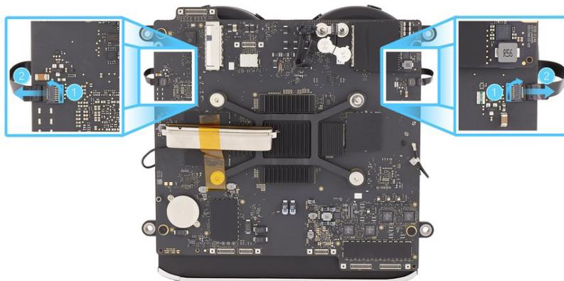
4. Rotate the logic board to access the other side. Use the T10 screwdriver to remove the three T10 screws (923-0333) from the fan.
