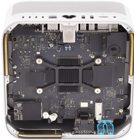
7. Use the T5 screwdriver to remove the two T5 screws (923-07093) from the front USB-C ports.
