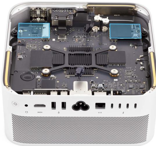
2. Use ESD-safe tweezers to peel the SSD module cover off the SSD module.
