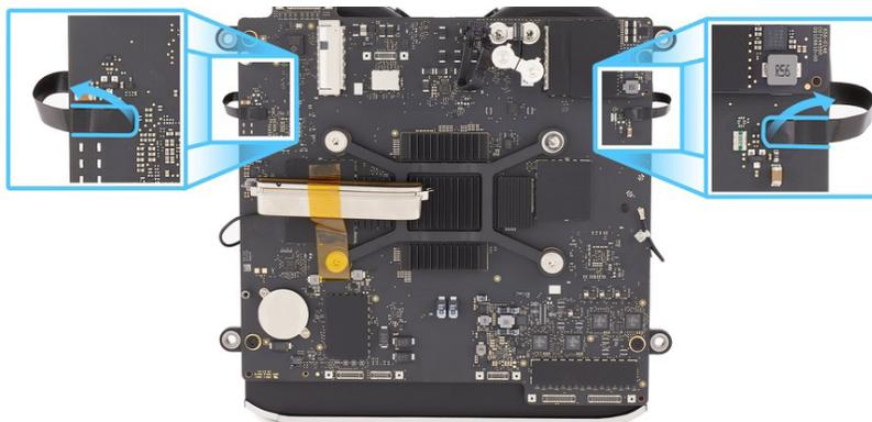
3. Use the black stick to flip up the locking levers on the two fan connectors (1). Then slide the ends of the two fan flex cables out of the connectors (2).
