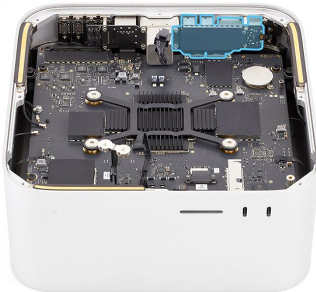
14. Insert the Torx T8 bit into the 10–34 Ncm adjustable torque driver. Set the torque value to 16 Ncm.
