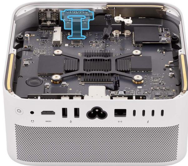
2. Use the T3 screwdriver to remove the four T3 screws (923-07105) from the two SDXC card slot board connector cowlings.
