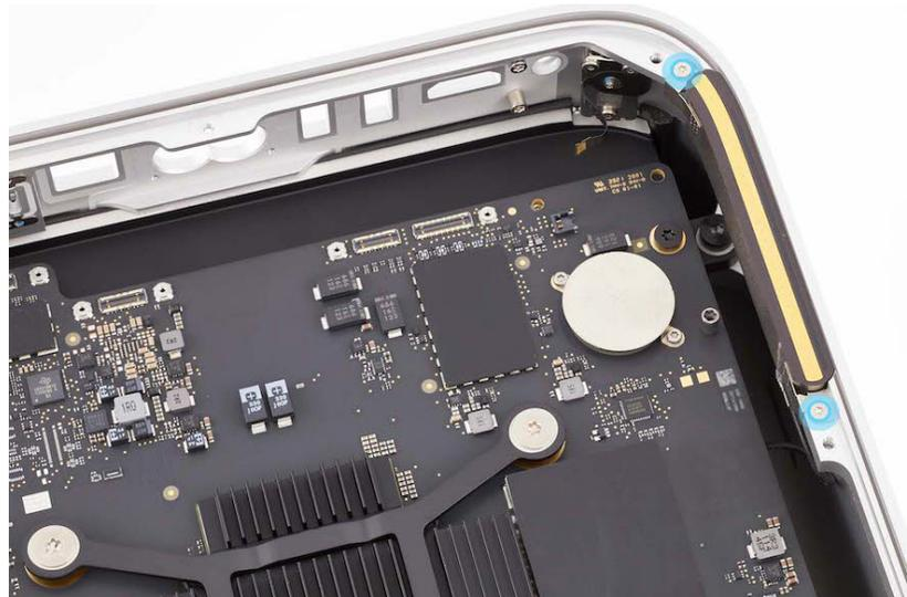
4. Lift antenna 1 from the housing (1). Then secure antenna 1 to the logic board with a piece of Kapton tape (2).
