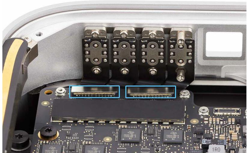
14. Position the back Thunderbolt 4 ports connector cowling over the ends of the back Thunderbolt 4 ports flex cables. Then use the green torque driver and Torx T3 half-moon bit to reinstall the two T3 screws (923-07105) into the cowling.
