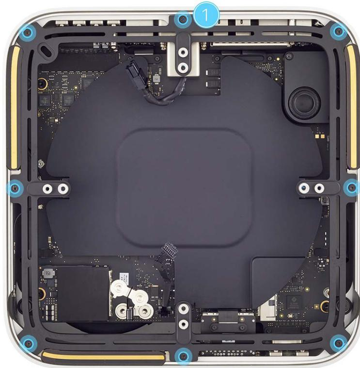
3. Move the power cord port cable (1) and power supply signal cable (2) out of the way as you lift the internal frame out of the housing.
