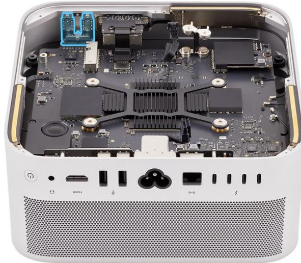
2. Use the T5 screwdriver to fully loosen the T5 screw on the front USB-C bracket. Remove the bracket and save it for reassembly.
