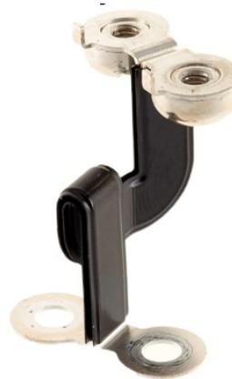
22. Remove the power supply signal cable and save it for reassembly.
