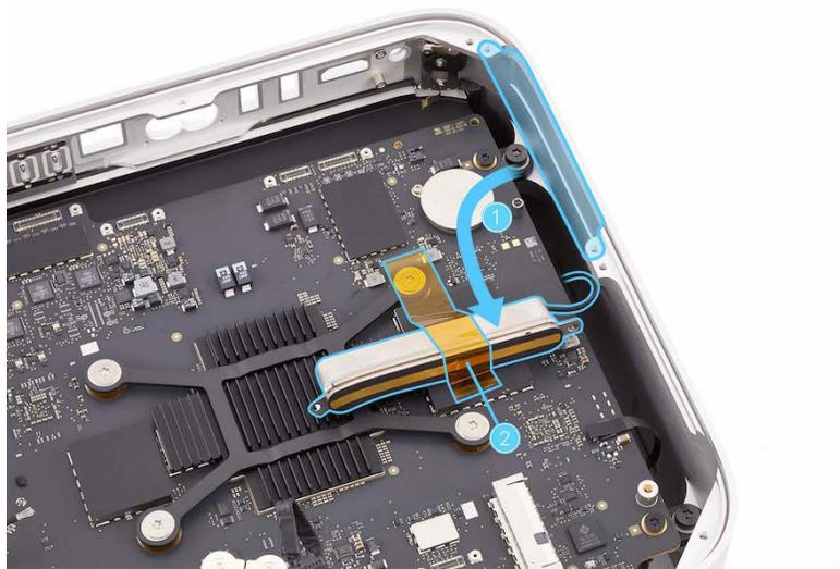
5. Rotate the computer to access the other side as shown. Use the antenna tool to lift the ends of two of the three antenna coaxial cables off the connectors on the logic board.
