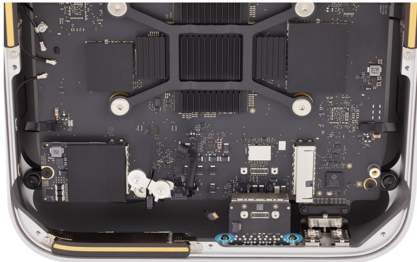
9. Lift the SDXC card slot board out of the housing.
