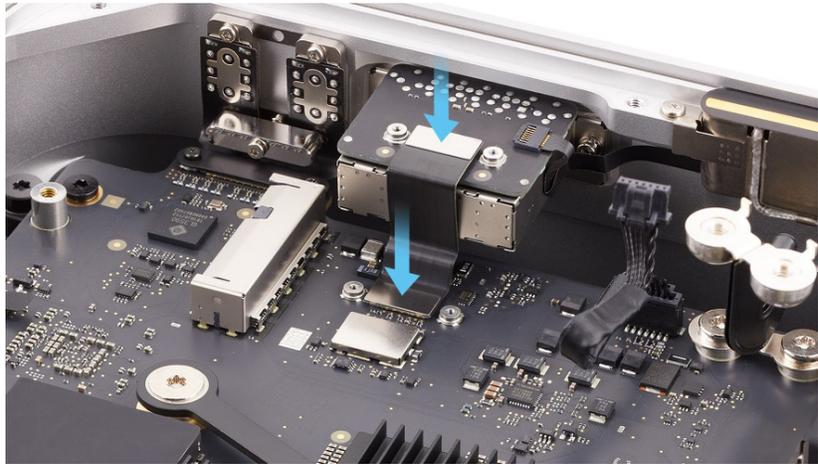
7. Position the SDXC card slot board connector cowlings over the ends of the flex cable. Then use the green torque driver and Torx T3 half-moon bit to reinstall the four T3 screws (923-07105) into the two cowlings.
