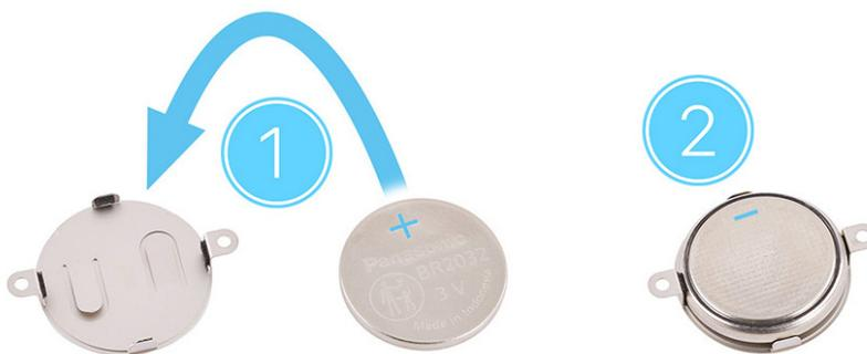
2. Turn over the battery cover with the battery and position it on the logic board. Align the screw cutouts in the battery cover with the screw holes in the logic board.
