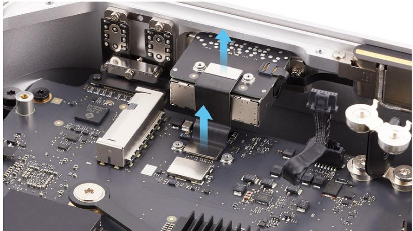
5. Use the flat end of the black stick to flip up the locking lever on the status indicator light flex cable.
