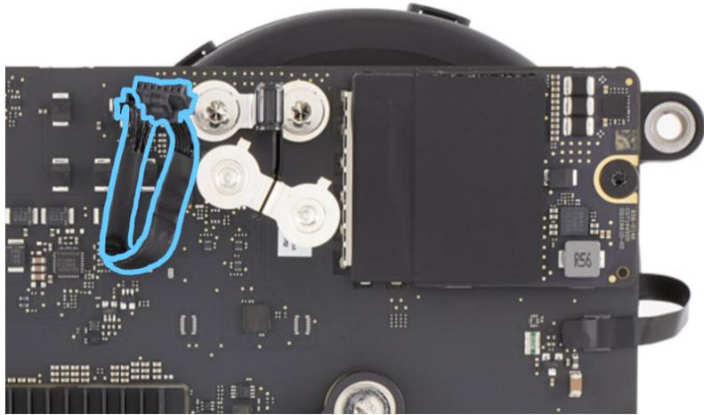
23. Remove the [SSD modules](#), [fan](#), and [antenna 1](#) from the logic board and save them for reassembly.
