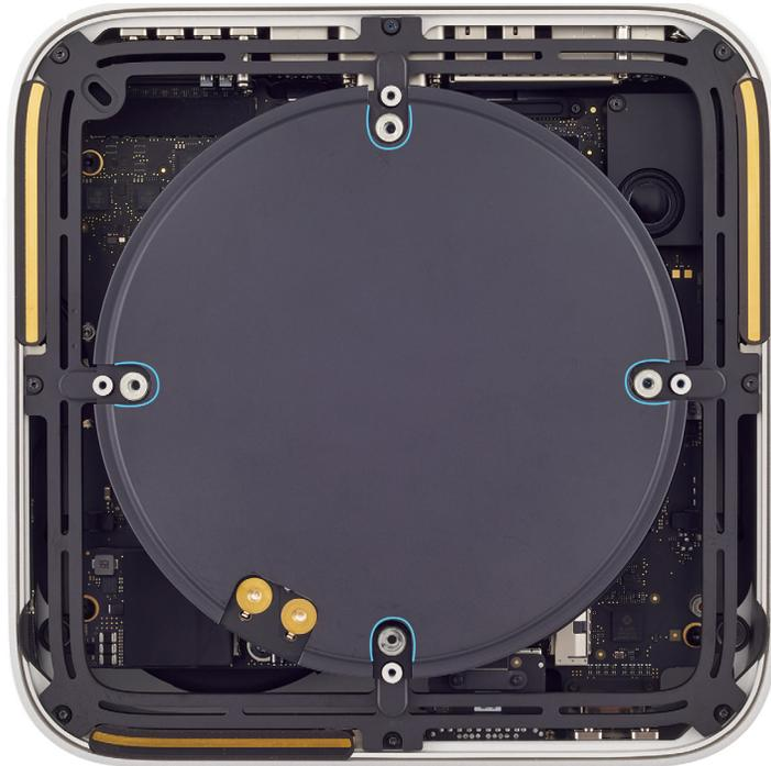
3. Rotate the computer so the back ports are facing you. Slightly tilt up the power supply. Slide the end of the power cord port cable into the connector. Ensure that the clip is engaged. Then tilt down the power supply onto the internal frame.
