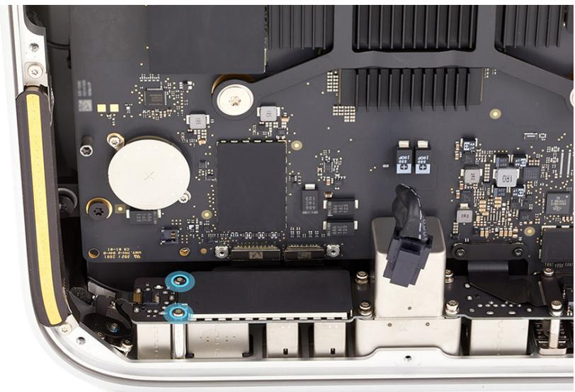
10. Use the T6 screwdriver to remove the two T6 screws (923-07100) from the combination I/O board and power cord port.
