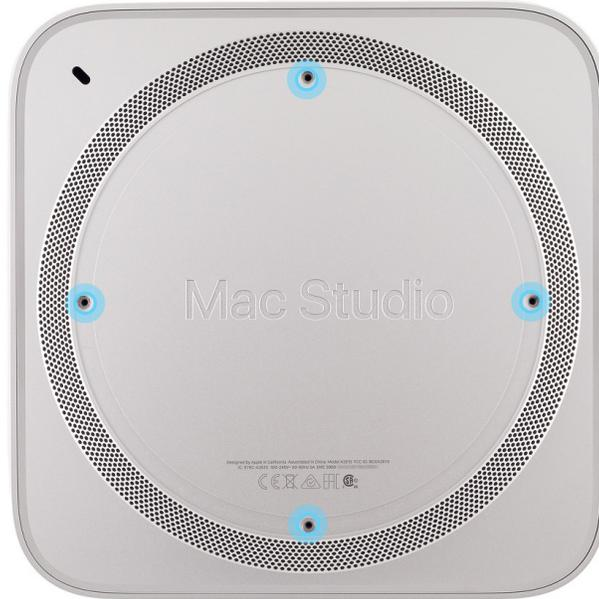
4. Identify the underside of the bottom cover screw pad.
