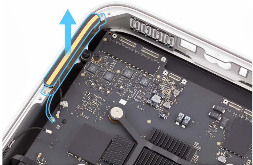
9. Rotate the computer as shown to access antenna 3.
