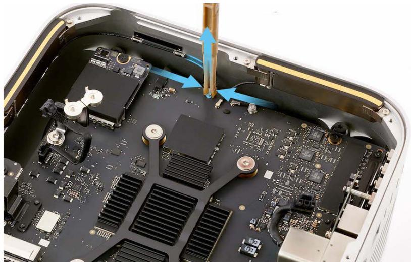
3. Lift the antenna coaxial cable out of the antenna coaxial cable grounding clips in the housing.
