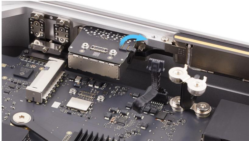
6. Slide the end of the status indicator light flex cable out of the connector (1). Then gently peel the flex cable off the side of the SDXC card slot board (2).
