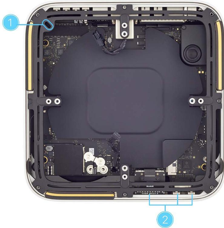
3. Use the T6 screwdriver to partially reinstall one T6 screw (923-07112) (1) over the power cord port.
