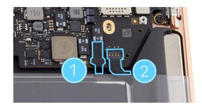
Position the ends of the antenna coaxial cables over the connectors. Use the blunt end of the antenna tool to press the ends of the antenna coaxial cables to the connectors.
