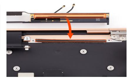
13. Lower the antenna module into the top case with the gasket side down. Route the TCON board through the opening of the antenna module.
