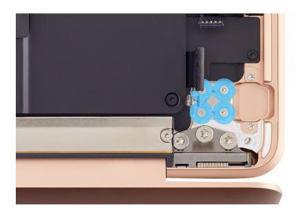
10. Use the T3 screwdriver to partially reinstall the two middle T3 screws (923-02888) into the flexible cowling.
