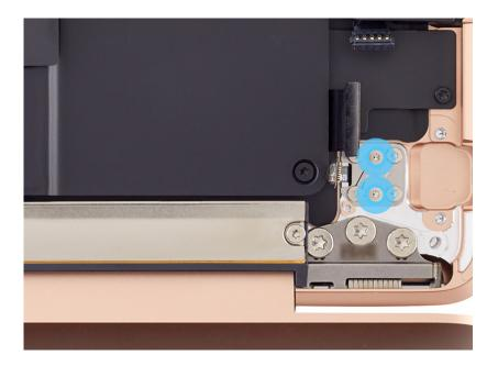
11. Use the T3 screwdriver to fully reinstall the four corner T3 screws. Then use the same screwdriver to fully reinstall the two middle T3 screws.
