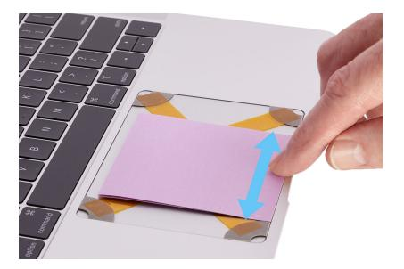
16. If the trackpad is at the correct height, continue to step 17. If the trackpad edges are higher or lower than the top case, remove the sticky notes, gap offsets, and Kapton tape. Place the computer on the edge of the table with the display hanging down. Use the T5 screwdriver to remove the four outer corner T5 screws (923-02880), and repeat removal steps 6 through 12. Then follow reassembly steps 1 through 15.
