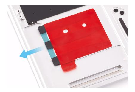
5. Use the flat end of the black stick to press the tabs onto the top case.
