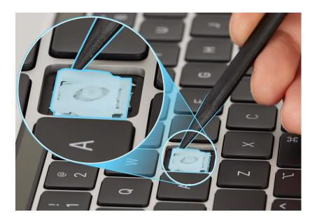
2. Use tweezers to lift the scissor mechanism out of the well.
