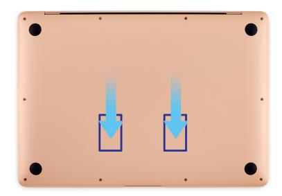
6. Ensure that the screw holes in the bottom case align with the screw holes in the top case.
