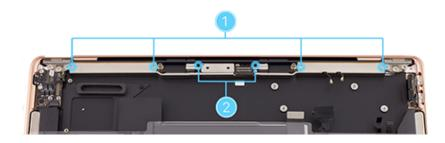
3. Gently slide the flat end of the black stick below one of the four screw holes (1) to loosen the antenna module from the tape on the top case. Then rotate the black stick until you feel a click (2).
