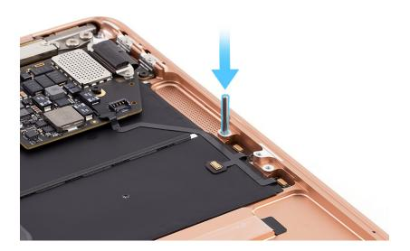
10. Turn the two alignment pins clockwise to screw them into the screw holes.
