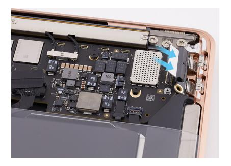
2. Use the T5 screwdriver to partially reinstall the two T5 screws (923-03975) into the I/O board.
