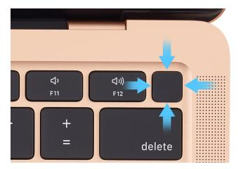
14. Press the Touch ID button to ensure that it clicks. If the button doesn't click, determine the required shim size. Then repeat the Touch ID board removal procedure to install the shim.
