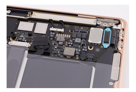
3. Lift the end of the I/O board flex cable off the connector.
