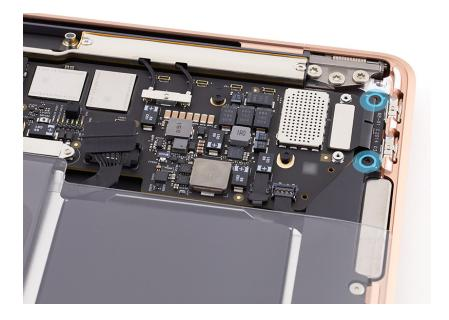
3. Plug both ends of the USB-C charge cable into the ports to ensure I/O board alignment. Adjust the alignment of the I/O board until the ends of the cable are easy to insert and remove.
