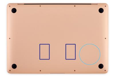
8. Lift the bottom case off the top case. Set the bottom case faceup on a clean, flat surface.
