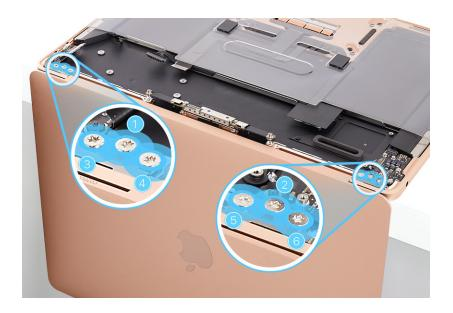
4. Close the display and adjust it until it's flush with the top case.
