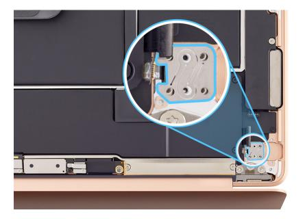
9. Use the T3 screwdriver to partially reinstall the four corner T3 screws (923-02888) into the Touch ID board flexible cowling.
