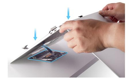
6. Slide the end of the IPD flex cable into the connector. Then flip down the locking lever.
