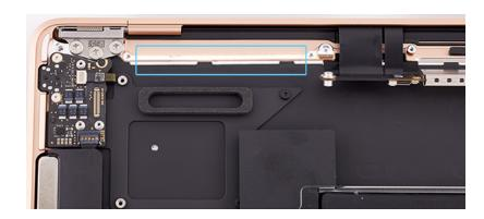
7. Inspect the gaskets for damage on the right and left sides of the antenna module. If the gaskets look like these examples, skip to step 13.
