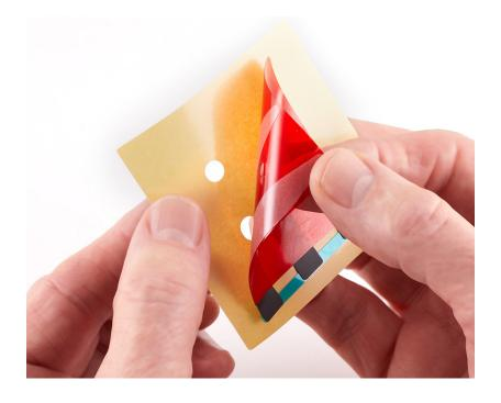
3. Align the battery adhesive over the corner of the top case as shown.
