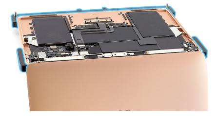
15. Align the holes on the press plate over the pins on the support frame. Lower the press plate onto the battery.
