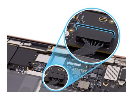
2. Press the end of the battery flex cable to the connector (1). Then flip the locking bar all the way down (2).
