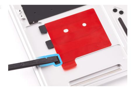
6. Press the top release liner to remove any air bubbles and adhere the battery adhesive strips onto the top case.
