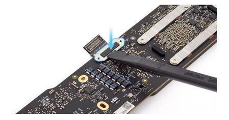
2. Use the T3 screwdriver to reinstall the two T3 screws (923-02890) into the eDP flex cable with connector cowling.
