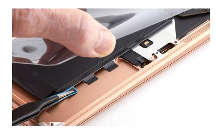
8. Gently peel the battery adhesive tab off the top case. Slowly pull the adhesive tab past the battery cover. As the adhesive strip stretches, twist the tweezers to wrap the strip around them. Continue to slowly pull and twist the tweezers until you've removed the entire strip. Then lower the corner of the battery cover.
