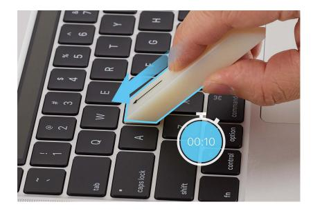
5. Tilt up the keycap lever in the direction of the arrow until you feel the snaps release.
