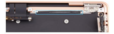
2. If the tape is wrinkled or misaligned but not torn (1), use the pointed end of the black stick to smooth it (2). Then skip to step 7. If the tape is torn away from the top case (3), use ESD-safe tweezers to remove the tape.
