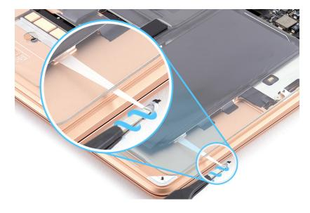
9. Repeat steps 6 through 8 to remove the two remaining battery adhesive strips from this side and the three adhesive strips from the other side. Then continue to step 10.
