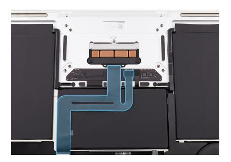
Lift the computer off the table and allow the IPD flex cable to pass through the opening in the top case.
