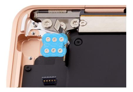
2. Use ESD-safe tweezers to remove the Touch ID board flexible cowling. Save the flexible cowling for reassembly.
