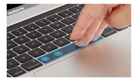
4. Tap the key repeatedly to verify that it springs back each time. If the keycap doesn't appear to be correctly installed, repeat all removal and reassembly steps with a new keycap.
