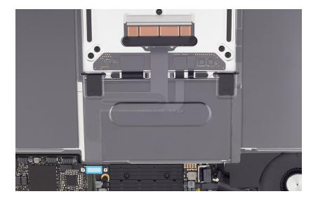
5. Use the T5 screwdriver to remove the middle T5 screw (923-03002) and the eight corner T5 screws (923-02880).
