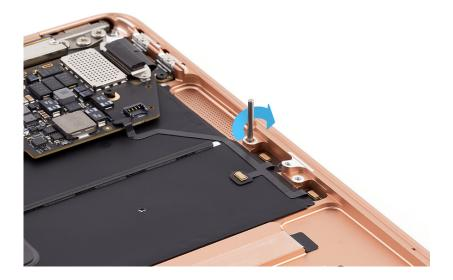
11. Align the screw holes on the battery tray over the alignment pins and lower the battery onto the top case.
