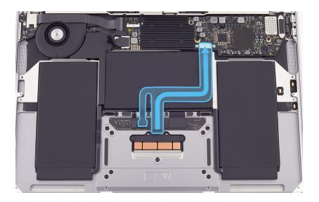
24. Place the battery cover on the battery and press the black tabs into the clips on the top case until you feel a click.
