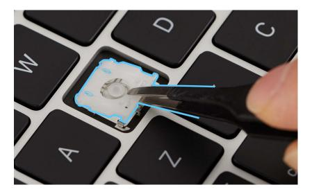
3. Use the black stick to engage the scissor pins with the lower hooks. The pin is engaged as shown (1). The pin is not engaged as shown (2).
