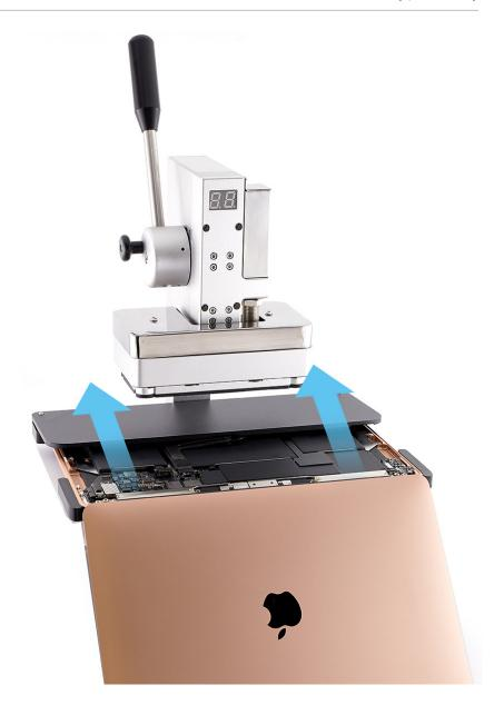
17. Ensure that the support frame is aligned with the back of the iPhone display press as shown.
