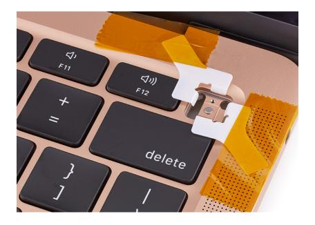
6. Stand the computer on its side. Route the Touch ID board flex cable through the slot in the top case. Then position the Touch ID board in the opening in the top case.
