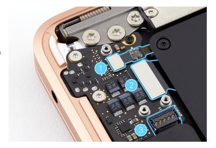
6. Plug the EarPods into the 3.5 mm headphone jack to ensure audio board alignment. Adjust the alignment of the audio board until the plug is easy to insert and remove.
