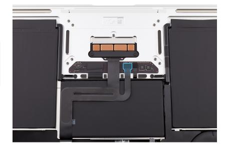
7. Place the battery cover on the battery and press the black tabs into the clips on the top case until you feel a click.
