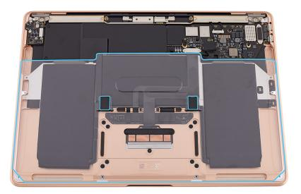
6. Tilt up the side of the battery cover to access the battery adhesive tabs. Press and hold the battery cover tab to ensure that it remains clipped into the top case.
