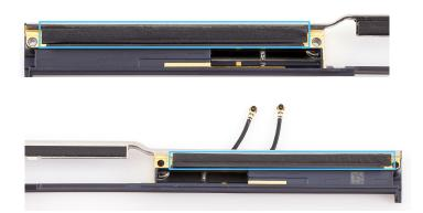
If one or both of the gaskets are wrinkled (1), use the flat end of the black stick to smooth them (2). Then skip to step 13. If one or both of the gaskets are torn (3), use ESD-safe tweezers to remove the gaskets.
