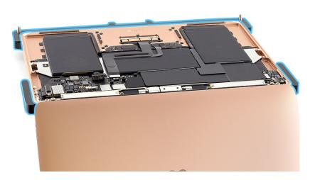
15. Align the holes on the press plate over the pins on the support frame. Lower the press plate onto the battery.
