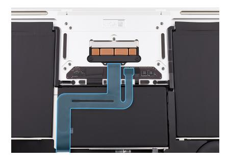
9. Lift the computer off the table and allow the IPD flex cable to pass through the opening in the top case. Leave the trackpad flat on the table to keep the shims in place.
