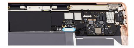
4. Use the black stick to lift the end of the IPD flex cable off the connector.
