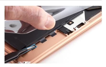
8. Gently peel the battery adhesive tab off the top case. Slowly pull the adhesive tab past the battery cover. As the adhesive strip stretches, twist the tweezers to wrap the strip around them. Continue to slowly pull and twist the tweezers until you've removed the entire strip. Then lower the corner of the battery cover.
