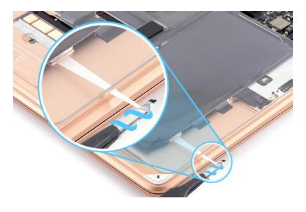
9. Repeat steps 6 through 8 to remove the two remaining battery adhesive strips from this side and the three adhesive strips from the other side. Then continue to step 10.
