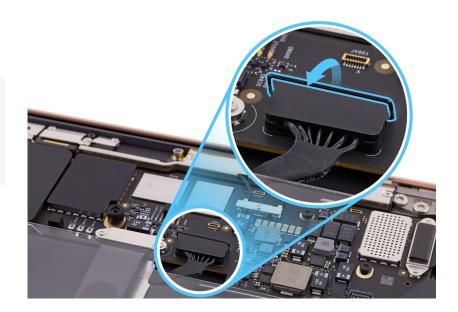
11. Use the flat end of the black stick to lift the end of the battery flex cable off the connector.
