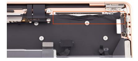
Inspect both sides of the top case for damage to the tape. If the tape looks like these examples, skip to step 7.
