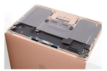
3. Use the T8 screwdriver to partially reinstall the six T8 screws (923-03997) into the display hinges in the order shown.
