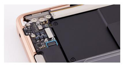
Place the flat end of the black stick under the left speaker flex cable to loosen the adhesive and peel the flex cable from the logic board. Then use the black stick to lift the end of the flex cable off the connector.
