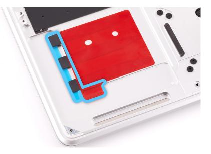
4. Remove the tab release liner strip out from under the three adhesive tabs.
