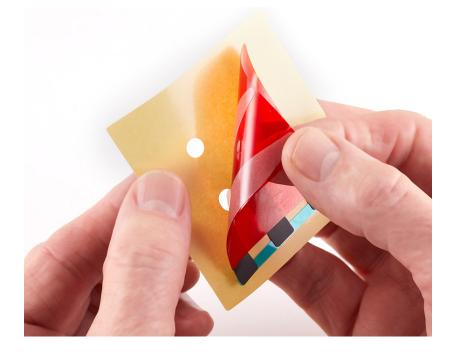
3. Align the battery adhesive over the corner of the top case as shown.
