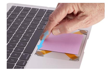
15. To verify the bottom of the trackpad is at the correct height, align a stack of two sticky notes on the trackpad's bottom edge. Ensure that the two sticky notes are flush with the top case.
