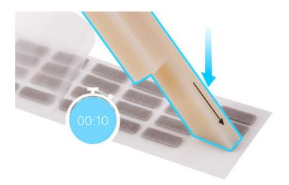
2. Lift the keycap lever and the adhesive to separate them from the white liner.
