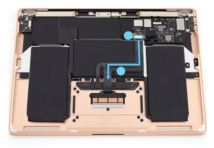
5. Place the battery cover on the battery. Then press the black tabs into the clips on the top case until you feel a click.
