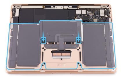
10. Flip up the locking bar on the end of the battery flex cable.
