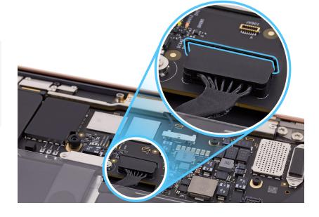
2. Press the end of the battery flex cable to the connector (1). Then flip the locking bar all the way down (2).
