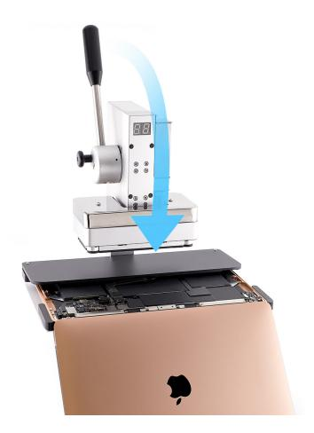
Wait until the timer on the iPhone display press beeps (1). Pull down the lever slightly and pull out the release knob (2). Then lift the lever (3).
