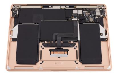
22. Press the end of the IPD flex cable to the connector (1). Then gently adhere the flex cable to the battery (2).
