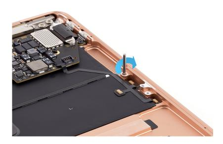
Align the screw holes on the battery tray over the alignment pins and lower the battery onto the top case.
