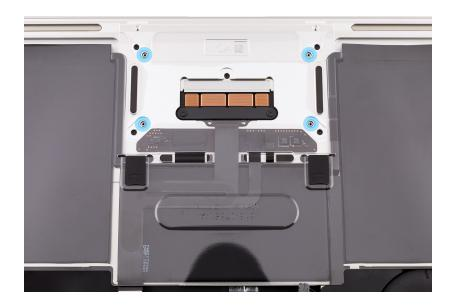
22. Hold the battery cover by the edges and lift it off the top case.
