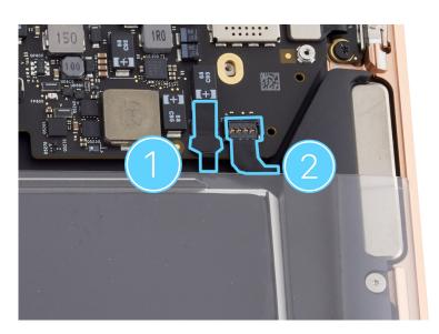
6. Use the antenna tool to lift the ends of the two antenna coaxial cables from the connectors.
