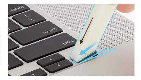
Push the keycap lever toward the hinge to release the keycap (1). Lift the keycap lever to release the keycap from the snaps (2).
