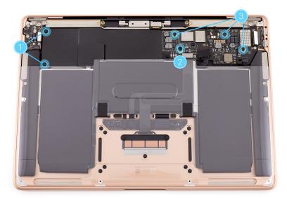
8. Hold the logic board by the edges. Then tilt up the logic board and slide it out of the top case.
