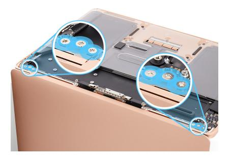
3. Pull the display toward you about 15 degrees (1). Move the display away from you to allow the hinges to clear the edge of the top case. Then lift the display up and out of the top case (2).
