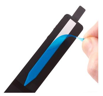
If you're reinstalling the existing speakers, peel the adhesive backing off the speaker adhesive strips. 2. Press one speaker adhesive strip onto the back of the speaker. Then peel the release liner off the adhesive strip as shown.
