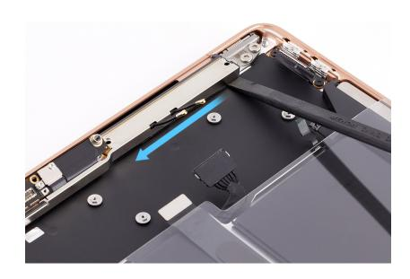
6. Lift the antenna module out of the top case.
