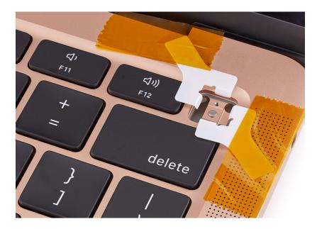
Stand the computer on its side. Route the Touch ID board flex cable through the slot in the top case. Then position the Touch ID board in the opening in the top case.
