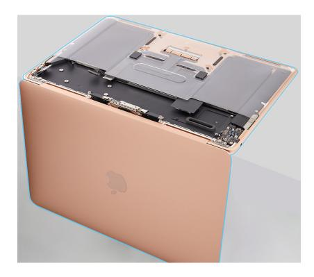
Use the T8 screwdriver to remove the six T8 screws (923-03997) from the display hinges.
