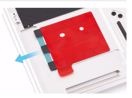
5. Use the flat end of the black stick to press the tabs onto the top case.
