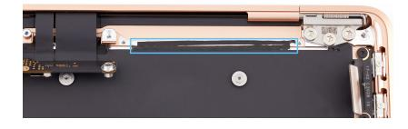
If the tape is wrinkled or misaligned but not torn (1), use the pointed end of the black stick to smooth it (2). Then skip to step 7. If the tape is torn away from the top case (3), use ESD-safe tweezers to remove the tape.
