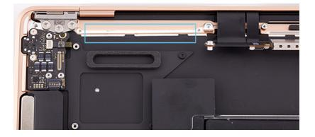
Inspect the gaskets for damage on the right and left sides of the antenna module. If the gaskets look like these examples, skip to step 13.
