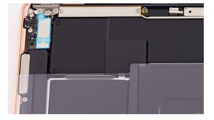
Place the pointed end of the black stick under the right speaker flex cable. Then use the black stick to lift the end of the flex cable off the connector.
