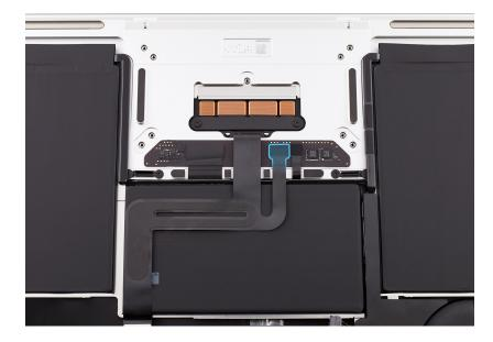
8. Gently peel the IPD flex cable off the battery.
