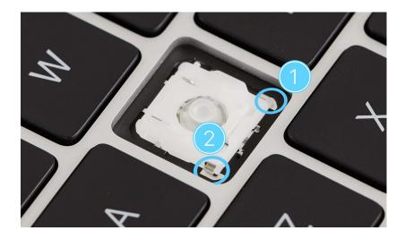
4. Use the black stick to gently move the scissor mechanism up and down. Ensure that the scissor mechanism moves easily and lies flat when released.
