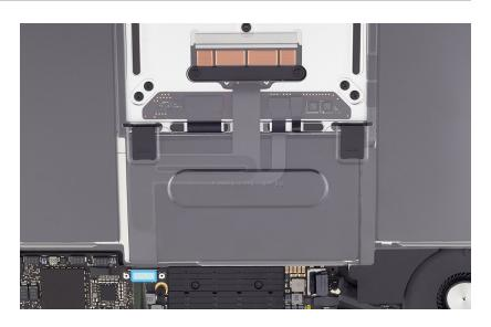
5. Use the T5 screwdriver to remove the middle T5 screw (923-03002) and the eight corner T5 screws (923-02880).
