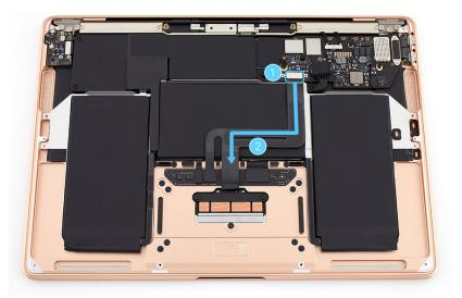
23. Place the battery cover on the battery. Then press the black tabs into the clips on the top case until you feel a click.
