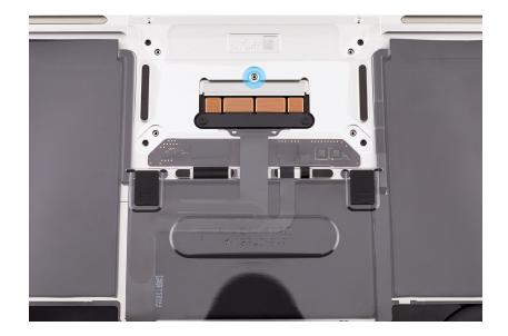
20. Insert the Torx T5 bit into the 10-34 Ncm adjustable torque driver. Set the torque value to 16 Ncm.
