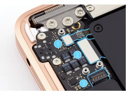
Plug the EarPods into the 3.5 mm headphone jack to ensure audio board alignment. Adjust the alignment of the audio board until the plug is easy to insert and remove.
