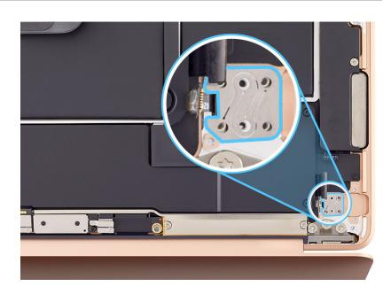
Use the T3 screwdriver to partially reinstall the four corner T3 screws (923-02888) into the Touch ID board flexible cowling.
