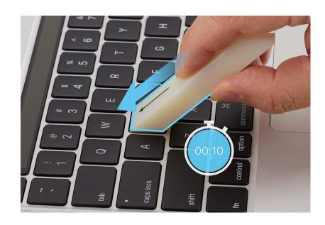
5. Tilt up the keycap lever in the direction of the arrow until you feel the snaps release.
