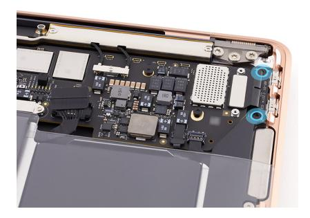
5. Hold the edges of the I/O board and gently slide it out of the ports.
