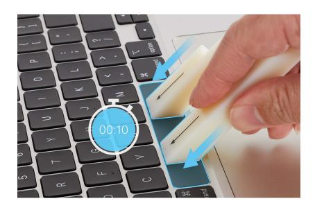
7. Tilt up the keycap levers in the direction of the arrows until you feel the snaps release.
