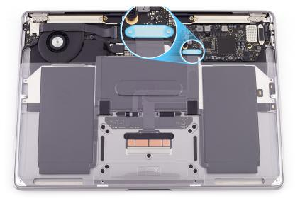
27. Turn over the computer. Use the flat end of the black stick to lift off the gap offsets and Kapton tape.
