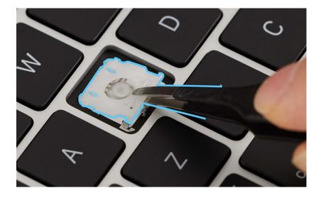
3. Use the black stick to engage the scissor pins with the lower hooks. The pin is engaged as shown (1). The pin is not engaged as shown (2).
