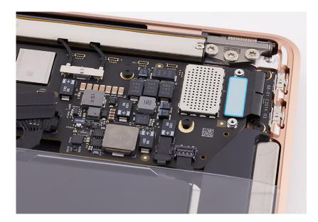
4. Use the T5 screwdriver to remove the two T5 screws (923-03975) from the I/O board.
