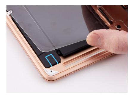
Use the T3 screwdriver to reinstall the T3 screw (923-03850). Then lower the corner of the battery cover.
