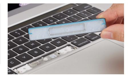
1. Position the keycap in the well and insert the top link bar into the metal hooks that are on each side of the well.
