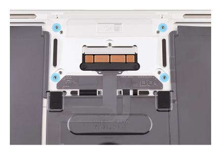
10. Turn over the computer. Insert one gap offset in each of the four corners of the trackpad. Then secure each gap offset with a piece of Kapton tape.
