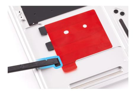
6. Press the top release liner to remove any air bubbles and adhere the battery adhesive strips onto the top case.
