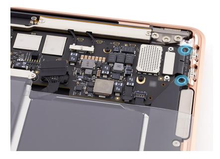
Plug both ends of the USB-C charge cable into the ports to ensure I/O board alignment. Adjust the alignment of the I/O board until the ends of the cable are easy to insert and remove.
