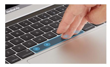
4. Tap the key repeatedly to verify that it springs back each time. If the keycap doesn't appear to be correctly installed, repeat all removal and reassembly steps with a new keycap.
