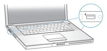
To use a USB device with your computer, connect the device to the computer. Your computer automatically detects newly connected devices and loads the correct software to work with the device.
