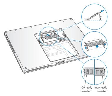
*Note:* Make sure your memory is installed according to this illustration, where the gold contacts are almost completely inserted into the connector.
