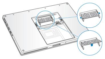
4 Insert the memory card at a 25-degree angle. Line up the notch in the card with the small tab in the memory slot and slide the card into the slot until the gold edge is almost invisible. Then firmly push the memory card into the memory slot. You might feel some resistance. 5 Gently spread the small tabs in the memory slot away from the notches and push the memory card down until the two snaps on either side of the card lock into place.
