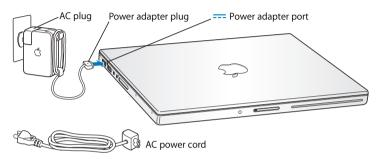
To extend the reach of your power adapter, you can attach the AC power cord. First, pull up on the AC plug to remove it from the adapter, and then attach the included AC power cord to the adapter. Plug the other end into a power outlet. For an illustration, see page 30.
