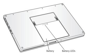
If the battery icon in the Finder menu bar is set to show the percentage of charge, you might sometimes notice that the battery does not attain a full 100 percent charge when the power adapter is attached. This is normal behavior; battery life is maximized if charging is not continuously cycled on and off when the battery's charge capacity is between 95 and 100 percent. When the battery level eventually drops below 95 percent, it will charge all the way to 100 percent.
