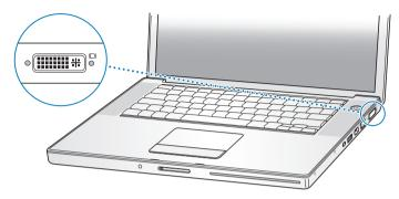
When an external monitor or TV is connected, you can either have the same image appear on both the built-in display and the external monitor (known as *video mirroring*) or use the external monitor to extend the size of the Mac OS desktop (known as *dual-display* or *extended desktop mode*). By default, your MacBook Pro starts up in dual-display mode. Press the F7 (曰) key to switch between dual-display and video-mirroring modes.
