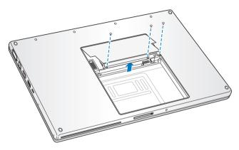
**2** Touch a metal surface inside the computer to discharge any static electricity from your body.
