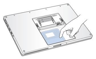
3 If you already have a memory card installed in the slot, remove it. Spread the tabs in the slot away from the notches in the memory card. The card should pop up slightly. Lift the memory card to a 25-degree angle and then gently slide the card out of the memory slot.
