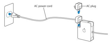
For best results, always use the AC power cord and connect it to a grounded power outlet when one is available. Use only the AC power cord that came with your power adapter. Make sure to push the power plug snugly into the power adapter port on the computer to ensure it is engaged and power is flowing to the computer. If the cord is plugged in properly, you will see an indicator light on the end of the cord that plugs into your MacBook Pro.
