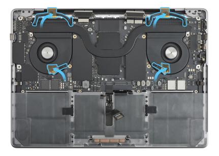
15. Use the black stick to slightly lift the edge of the logic board as shown.
