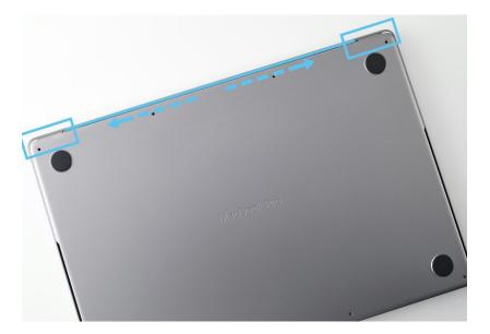
10. Put on the gloves. Hold the bottom case by the front corners and slowly push it away from you to align it with the display hinge and top case.
