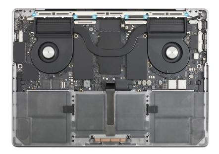
4. Position the ends of the antenna coaxial cables over the connectors. Use the blunt end of the antenna tool to press the ends of the antenna coaxial cables to the connectors.
