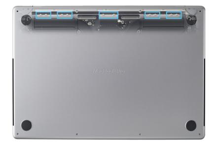
12. Lift the front edge of the bottom case no more than 1 inch (2.5 cm) to align the thermal fan ducts.
