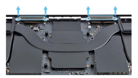
4. Lift the display cable bumpers out of the top case. Save them for reassembly.
