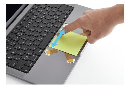
13. To verify that the bottom of the trackpad is at the correct height, align a stack of two sticky notes on the trackpad's bottom edge. Ensure that the two sticky notes are flush with the top case.
