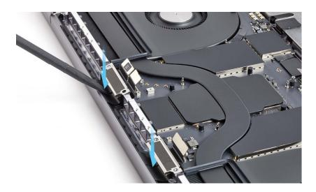
10. Use the black stick to tuck each display flex cable into the gap between the logic board and the internal frame. Ensure that the display flex cable clips are fully clipped onto the internal frame.
