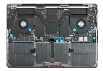
11. Use ESD-safe tweezers to remove the polyester film covers from the four T5 screws. Save the covers for reassembly. Then use the T5 screwdriver to remove the four T5 screws (923-07039).
