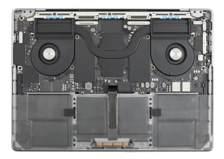
3. Use the T5 screwdriver to reinstall two outer T5 screws (923-06850) and four middle T5 screws (923-07032).
