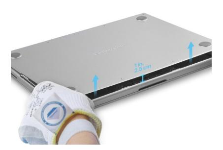
13. Press both sides of the bottom case simultaneously until you feel the two internal clips snap into place (1). Then simultaneously press the two areas in the middle (2) to attach the two remaining internal clips.
