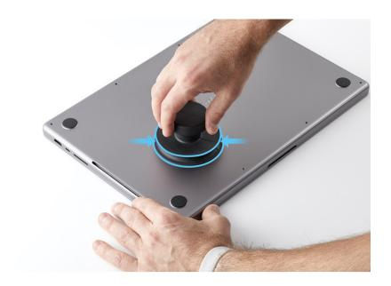
7. Move the suction cup to the lower right corner and press the top to attach it to the bottom case.
