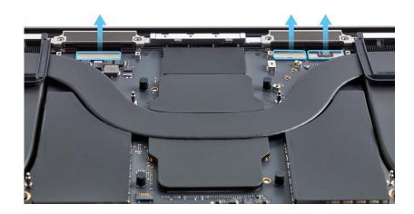
3. Lift the display cable clips off the internal frame of the top case. Gently fold them back over the edge of the top case to reveal the display cable bumpers underneath.
