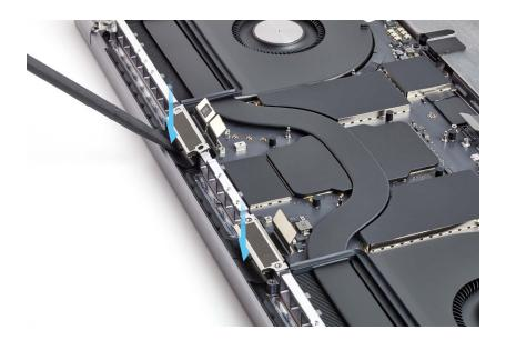
32. Use the black stick to tuck the display flex cables into the gap between the logic board and internal frame. Ensure that the display cable clips are fully clipped onto the internal frame.
