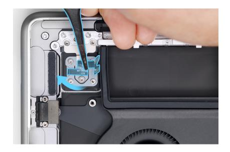
2. Use the T3 screwdriver to remove the two T3 screws (923-06940) from the Y-shaped cowling.
