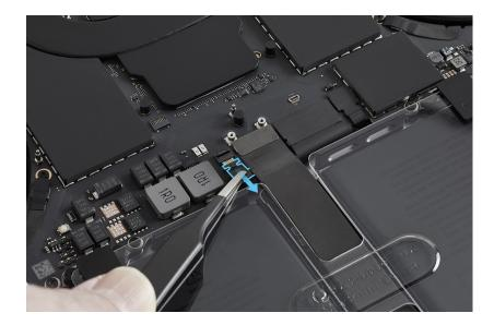
17. Lift the end of the trackpad flex cable off the connector on the logic board.
