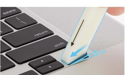
6. Push the keycap lever toward the hinge to release the keycap (1). Lift up the keycap lever to release the keycap from the snaps (2).
