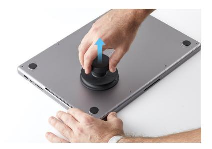
6. Squeeze the edges of the suction cup to release it.
