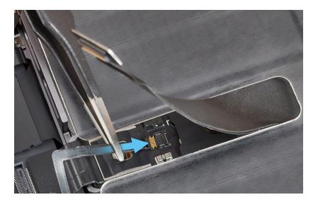
2. Use the black stick to flip down the locking lever on the BMU flex cable connector.
