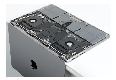
2. Use the T5 screwdriver to remove the eight outer T5 screws (923-06941) and the two inner T5 screws (923-06941).
