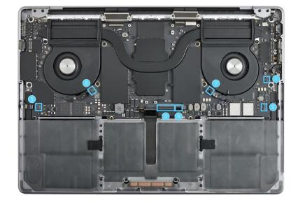
9. Use ESD-safe tweezers to loosen the adhesive and peel the left and right fan flex cables from the logic board.
