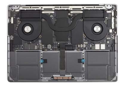
14. Use the T3 screwdriver to remove the two T3 screws (923-06851) from the trackpad connector cowling. Remove the cowling and save it for reassembly.
