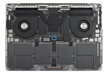
7. Hold the battery cover by the edges and lift it off the top case.
