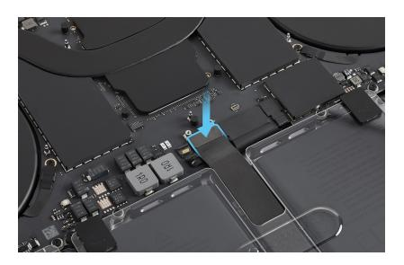
4. Use ESD-safe tweezers to slide the end of the BMU flex cable into the connector.
