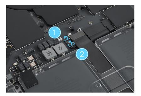
6. Position the trackpad flex cable cowling over the end of the trackpad flex cable. Then use the T3 screwdriver to reinstall the two T3 screws (923-06851) into the cowling.
