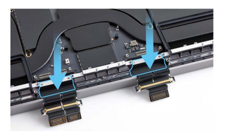
8. Align the display flex cables around the edge of the display cable bumpers (1). Then press the display flex cable clips down over the bumpers and onto the internal frame (2).
