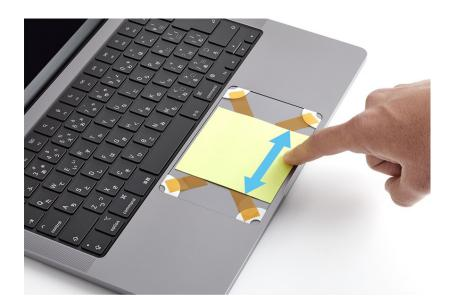
14. If the trackpad is at the correct height, continue to step 15. If the trackpad edges are higher or lower than the top case, remove the sticky notes, gap offsets, and Kapton tape. Place the computer on the edge of the table with the display hanging down. Use the T5 screwdriver to remove the four outer side T5 screws and repeat removal steps 2 through 6. Then follow reassembly steps 1 through 12.
