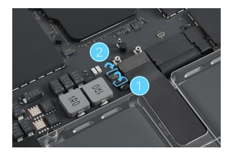
16. Use ESD-safe tweezers to gently grasp the end of the BMU flex cable and slide it out of the connector.
