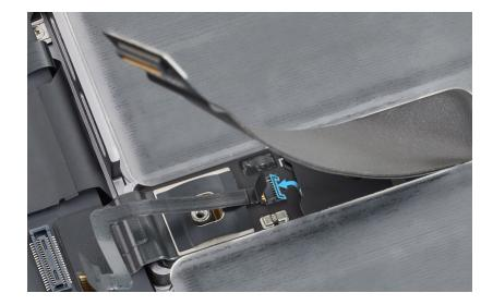
4. Use ESD-safe tweezers to gently slide the end of the BMU flex cable out of the connector.
