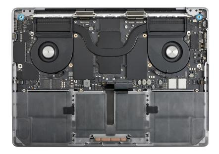
27. Use the T5 screwdriver to fully reinstall the 10 T5 screws.
