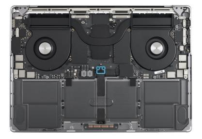
15. Gently peel the polyester film tab off the locking lever of the battery management unit (BMU) flex cable (1). Then use the black stick to flip up the locking lever (2).
