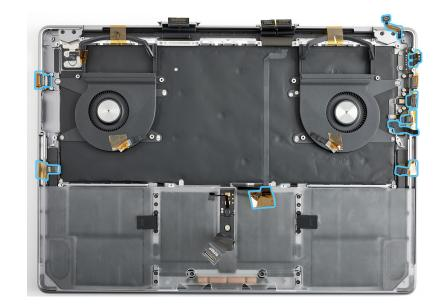
14. Hold the logic board by the edges. Tilt down the edge of the logic board to position it in the top case (1). Then lower the logic board into the top case (2). Guide the Touch ID board flex cable through the gap between the thermal module and logic board (3).
