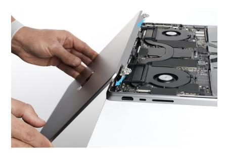
3. Use the T8 screwdriver to partially reinstall the six T8 screws (923-07042) into the display hinges in the order shown.
