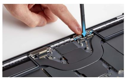
11. Press the ends of the display backlight power flex cable, FaceTime HD camera flex cable, and eDP flex cable to their connectors on the logic board.
