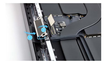
9. Use the black stick to tuck the display flex cables into the gap between the display and internal frame.
