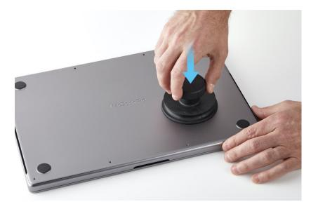
8. Pull up the handle of the suction cup until you feel the two internal clips on the right release.
