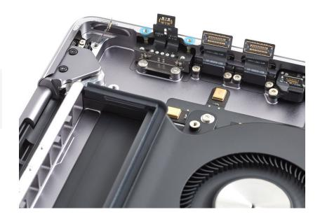
2. Use the T5 screwdriver to remove the two T5 screws (923-06959) from the MagSafe 3 board.
