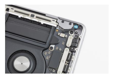
5. Remove the lid angle sensor from the top case.
