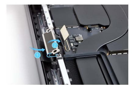
31. Use the black stick to tuck the display flex cables into the gap between the display and internal frame.
