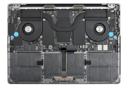
26. Use the T6 screwdriver to fully reinstall the two T6 screws.
