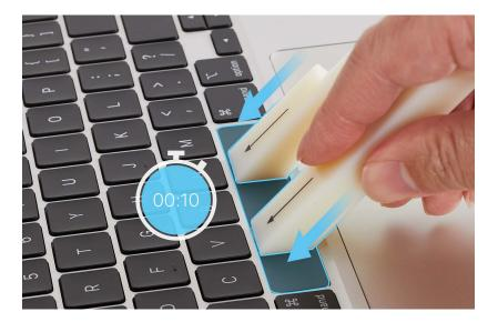
7. Tilt up the keycap levers in the direction of the arrows until you feel the snaps release.
