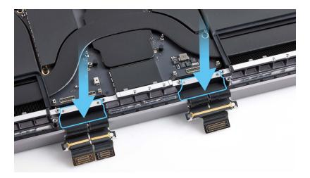
30. Align the display flex cables around the edge of the bumpers (1). Then press the display cable clips down over the bumpers and onto the internal frame (2).
