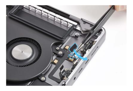
2. Use the T5 screwdriver to partially reinstall the two T5 screws (923-06938).
