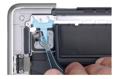
4. Use the T3 screwdriver to remove the two short T3 screws (923-06942) (1) from the Touch ID board flexible cowling. Then use the T3 screwdriver to remove the four long T3 screws (923-06942) (2) from the Touch ID board flexible cowling.
