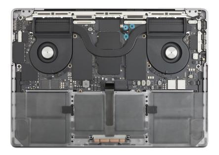
2. Use the antenna tool to lift the end of one antenna coaxial cable off the connector. Then repeat the process on the other two antenna coaxial cables.
