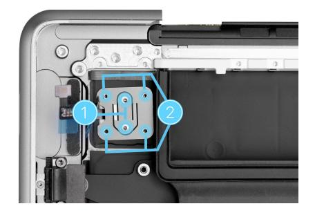
5. Use ESD-safe tweezers to remove the Touch ID board flexible cowling from the top case. Save the flexible cowling for reassembly.
