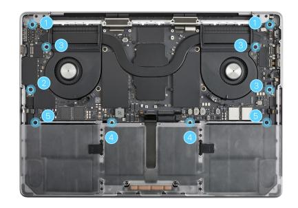
14. Fold back the thermal duct covers and fan flex cables. Use Kapton tape to hold them back as shown.
