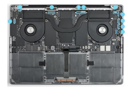
4. Lift the display flex cable clips off the internal frame of the top case. Gently fold them back to reveal the black bumpers underneath.
