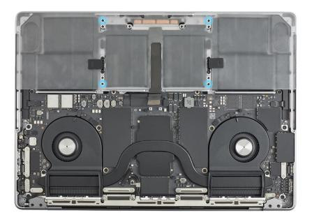
10. Turn over the computer. Insert four gap offsets into the corners of the trackpad. Secure each gap offset with a piece of Kapton tape.
