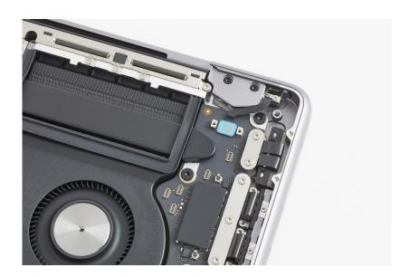
4. Use the blue torque driver and Torx security bit to remove the 1IPR screw (923-06852) from the lid angle sensor flex cable clip.
