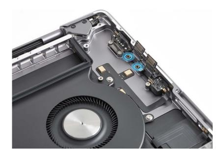
3. Plug one end of the USB-C charge cable into the port to ensure USB-C board alignment. Adjust the alignment of the USB-C board until the end of the cable is easy to insert and remove.
