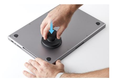
5. Four internal clips attach the bottom case to the top case. Pull up the handle of the suction cup until you feel the two internal clips on the left release.
