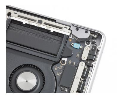
3. Position the lid angle sensor flex cable clip so the hole is aligned with the screw hole in the top case.
