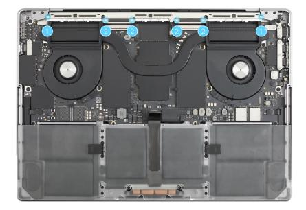
4. Use the blue torque driver and the Torx security bit to remove the nine 1IPR screws (923-07033) from the vent/antenna module.
