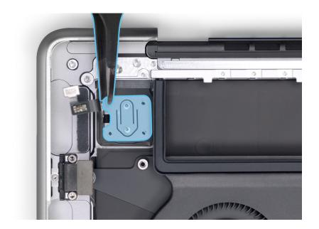
6. Tilt up the corner of the top case as shown. Then guide the Touch ID board flex cable out through the slot in the top case to remove the Touch ID board.
