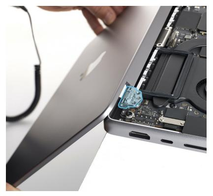
8. Remove the display from the top case as shown.
