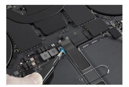
5. Flip down the locking lever of the BMU flex cable (1). Then press the polyester film tab to the locking lever (2).
