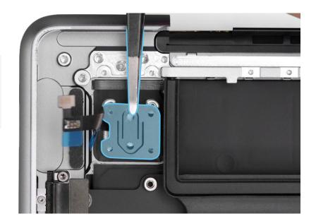
12. Use the T3 screwdriver to partially reinstall the two center T3 screws (923-06942) (1). Then use the T3 screwdriver to reinstall the four outer T3 screws (923-06955) (2).
