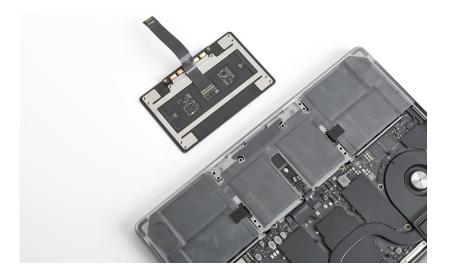
8. Flip up the locking lever on the trackpad flex cable connector (1). Then slide the end of the trackpad flex cable out of the connector (2).
