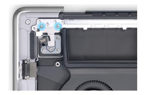
3. Use ESD-safe tweezers to remove the Y-shaped cowling from the top case. Save the cowling for reassembly.
