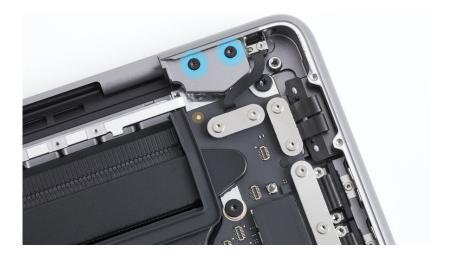
2. Use the black stick or ESD-safe tweezers to remove the two display hinge covers from the top case.
