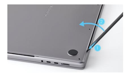
11. Remove the bottom case and set it faceup on a clean, flat surface.
