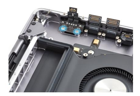
3. Lift the MagSafe 3 board out of the top case.
