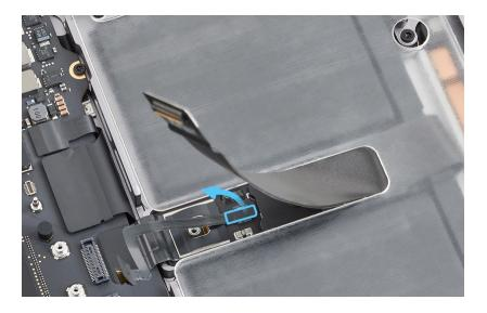
3. Use the black stick to flip up the locking lever of the BMU flex cable connector.
