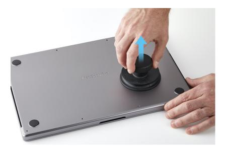
9. Squeeze the edges of the suction cup to release it.
