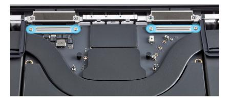
2. Lift the ends of the display backlight power flex cable, FaceTime HD camera flex cable, and eDP flex cable off the connectors.
