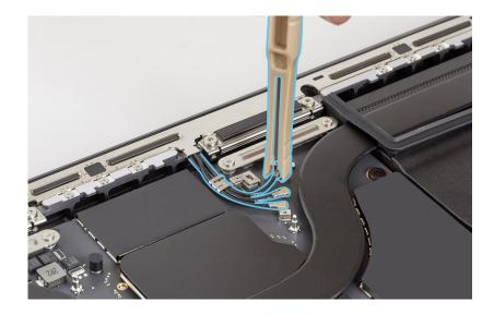
3. Use the T5 screwdriver to remove the two long outer T5 screws (923-06850) (1) and the four short inner T5 screws (923-07032) (2) from the vent/antenna module.
