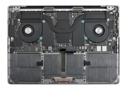
29. Rotate the top case as shown. Then position the black bumpers on the internal frame.
