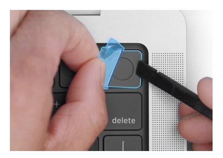
9. Set two Y-shaped alignment tools against the Touch ID button as shown. Secure the Y-shaped tools with Kapton tape.
