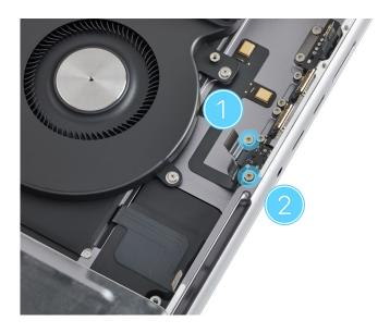
2. Lift the audio board out of the top case.
