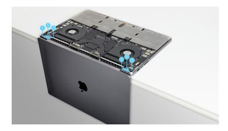
4. Close the display and stand the computer on its edge. Adjust the display until it's flush with the top case.
