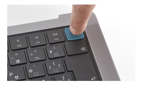
15. Turn the top case upside down. Use the T3 screwdriver to fully tighten the two center screws. Then ensure that the Touch ID button still clicks when pressed.
