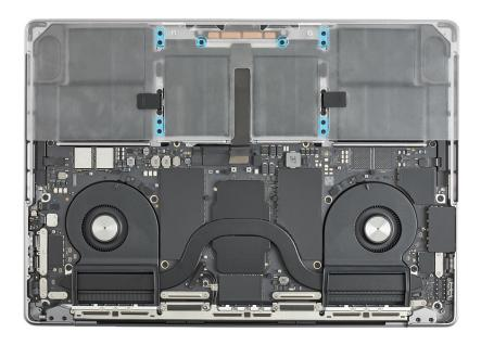
19. Hold the battery cover by the edges and lift it off the top case.
