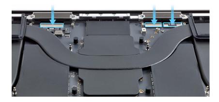
12. Position the two display connector cowlings over the ends of the display backlight power flex cable, FaceTime camera cable, and eDP flex cable connectors. Then use the T3 screwdriver to reinstall two T3 screws (923-06854) into each of the cowlings.
