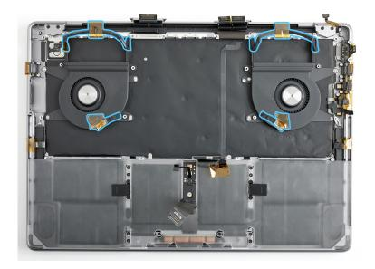
12. Ensure that the display backlight power flex cable and FaceTime HD camera and eDP flex cable are folded back over the edge of the top case.
