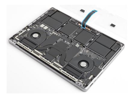
Lift the computer off the table and allow the trackpad flex cable to pass through the opening in the top case. Leave the trackpad flat on the table to keep the shims in place.
