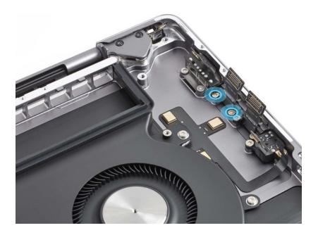
2. Slide the USB-C board out of the top case.
