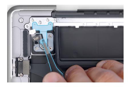
20. Use the T3 screwdriver to reinstall the two T3 screws (923-06940) into the Y-shaped cowling.
