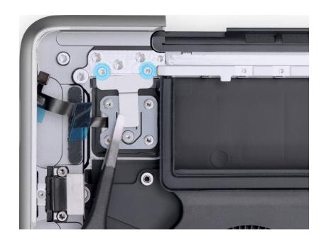
21. If you're installing a replacement Touch ID board, remove the blue protective liner under the Touch ID board flex cable.
