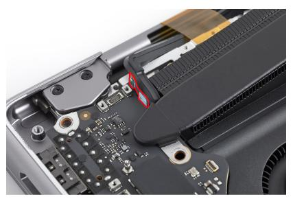
15. Gently remove the Kapton tape from the thermal ducts and flex cables.
