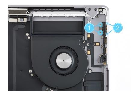
4. Plug the MagSafe 3 end of the USB-C to MagSafe 3 cable into the MagSafe 3 port to ensure MagSafe 3 board alignment. Use the flat end of the black stick to hold the MagSafe 3 board in place to create an even gap between the MagSafe 3 connector and top case.
