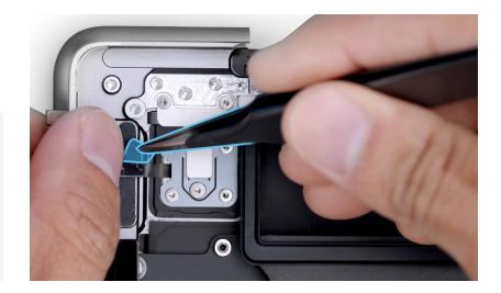
22. Gently run the flat end of the black stick along the length of the Touch ID board flex cable to adhere it to the Y-shaped cowling.
