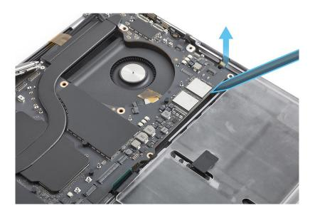
16. Gently tilt up the logic board as shown (1). Then slide the logic board out of the top case (2). Use the black stick to fold back the trackpad and BMU flex cables as you remove the logic board.
