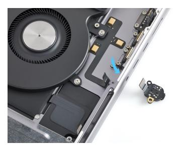
2. Use the T5 screwdriver to partially reinstall the short upper T5 screw (923-06936) (1) and the long lower T5 screw (923-06937) (2) into the audio board.
