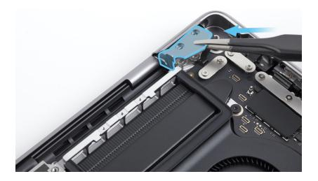
2. Use the T5 screwdriver to reinstall the two T5 screws (923-06853) into each display hinge cover.
