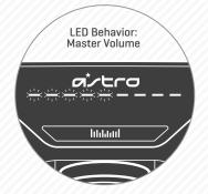
LED Array will fill up according to Volume.
