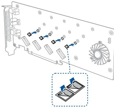
3. Secure the stand screws onto the ASUS HYPER M.2 X16 GEN 4 CARD.
