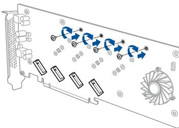
4. Insert the M.2 storage devices into the PCIe M.2 storage device connectors (A), then secure the M.2 storage devices with the bundled screws (B).
