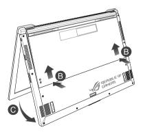
D. Secure the bottom cover using the screws you removed earlier.
