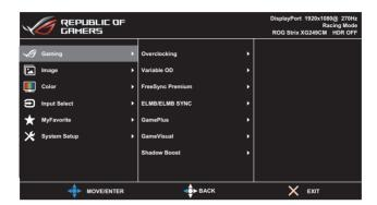
Overclocking: Allows to adjust the refresh rate.
