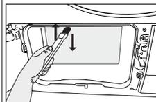
Clean the fibre on the metal surface of the condenser with damp cloth or the brush on the air deflector in up - down direction. Do not clean with left - right direction since it will damage the metal plates of the condenser.
