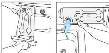
If lint builds up in the funnel on the water tank, remove it under running water.
