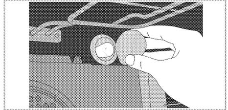
3. Remove the oven lamp by turning it counter clockwise and replace it with the new one.
