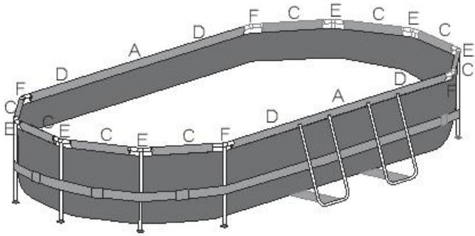
**Note:** The installation drawing for the Top Rail and the T-Connector of 4.88m x 3.05m x 1.07m (16' x 10' x 42")
