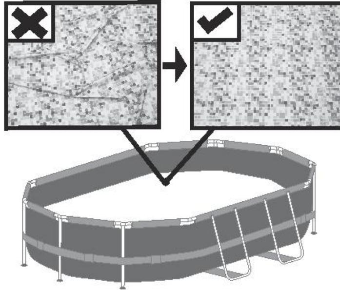
Put 1" to 2" water in the pool to cover the floor. Once pool floor is slightly covered, gently smooth out all wrinkles. Start in the center of the pool and work your way clockwise to the outside.
