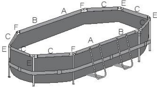
**Note:** The installation drawing for the Top Rail and the T-Connector of 3.00m x 2.00m x 84cm (9'10" x 6'7" x 33")
