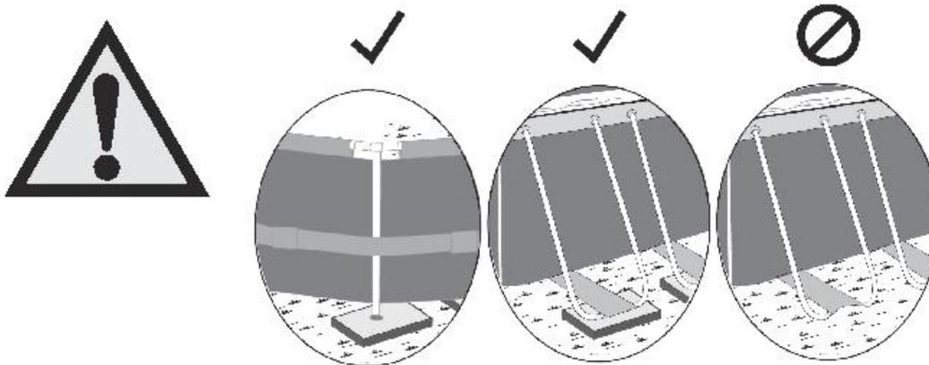
Do not assemble on soft lawn. If you must assemble the pool on a soft surface, timber boards (not included) must be placed under the feet of the vertical supports to spread the load.
