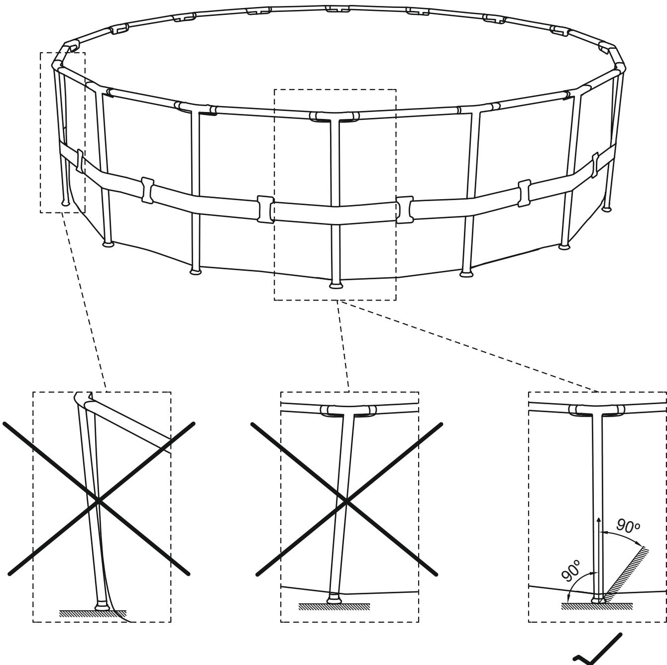
After the installation of the pool's steel frame is completed, ensure that the verticals are perpendicular to the ground. If they aren't, the verticals could be bent or deformed.
