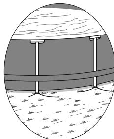
Do not assemble with pool legs on soft lawn. If you must assemble the pool on a soft surface, timber boards (not included) must be placed under the feet of the vertical support rods for even weight distribution.
