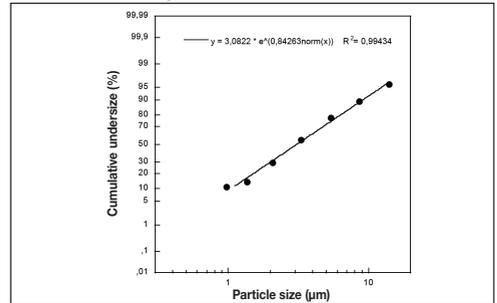
Measurements were performed using a sodium fluoride solution with a “Next Generation Impactor” (NGI).
