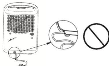
This device must be connected with the plug supplied via an outlet, do not use other connections for the connection.
