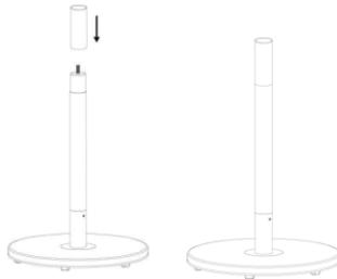
3. Screw the upper column (6) clockwise onto the middle column.
