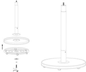
2. Screw the middle column (7) onto the lower column.
