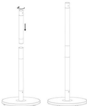
4. Insert the "fan head" on the upper column so that the two holes coincide and make certain it is blocked by tightening the screws (5) clockwise and making certain they are tight. At the end of the operation, check that the fan head and the column are assembled solidly and correctly.
