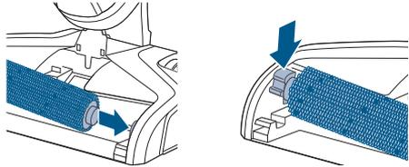
Replace brush roll by inserting the brush roll end into the right side of the foot. Then lock the pull tab into place by pressing downward.
