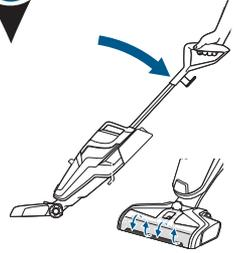
Recline the body of the machine backward to start the brush roll spinning. To stop the brush roll spinning, you will need to stand the machine upright.
