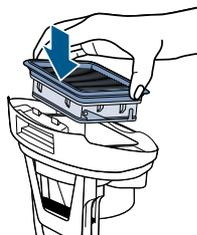
Place vacuum filter back into dirty water tank top.
