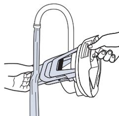
Rinse the float located at the bottom of the dirty water tank's top.
