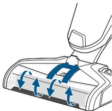
Before each use, hold the solution spray trigger for 10 seconds to prime the system with cleaning solution. LED lights illuminate when holding the trigger.
