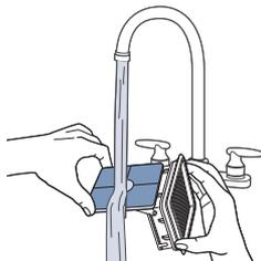
Hand wash the vacuum filter and screen with warm water and mild detergent.
