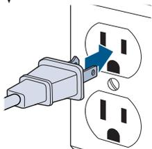
Plug machine into a properly grounded outlet.
