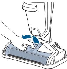
Grasp brush roll window at the front of the window and pull upward to remove.
