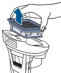
Remove the filter from the dirty water tank top by pulling it up.
