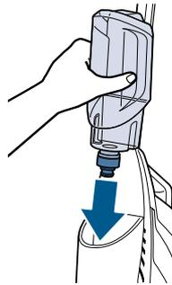
Then, on the back of the machine, align clean water tank with the grooves and slide tank into place until you hear a click.
