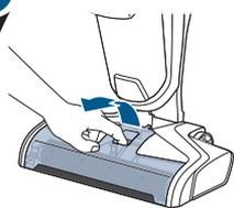
Grasp brush roll window at the front and pull upward to remove.
