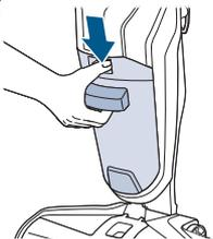
To release dirty water tank, press down on recessed button on the top of the dirty tank.
