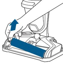
Pull brush roll out by grabbing the brush roll tab and pulling upward.
