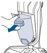
Grab the front handle while pressing down on button and pull dirty water tank away from the unit.
