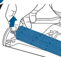
Pull brush roll out by grabbing the brush roll tab and pulling upward.
