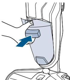
Angle the dirt tank back into body of machine inserting bottom first. Then tilt the top of the dirt tank toward the machine and push into place until you hear a click.
