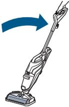
Recline the machine while in storage tray. Allow the machine to run for 10-15 seconds until all water is picked up. Repeat as needed.
