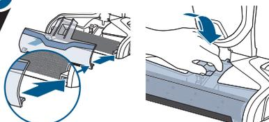
Replace the brush roll window by first lining up the brush window tabs with the edges of the foot. Then press the window back into place until you hear a click.
