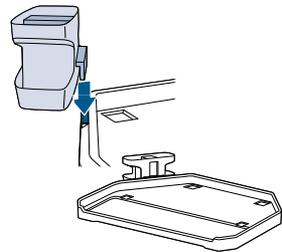
The Easy Clean Storage Tray consists of a machine storage tray and a brush roll drying tray. To assemble the Easy Clean Storage Tray, align arrows on the storage tray with the arrows on the brush roll drying tray and slide into place.
