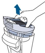
Grasp top of dirty water tank in recessed areas on each side of the filter and pull upward to remove the top of the tank.
