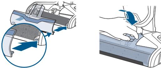
Replace the brush roll window by first lining up the brush window tabs with the edges of the foot. Then press the window back into place until you hear a click.
