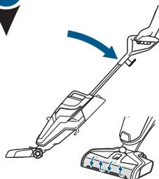
Recline the body of the machine backward to start the brush roll spinning. To stop the brush roll spinning, you will need to stand the machine upright.
