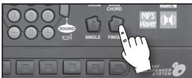
When using chords in SINGLE or FINGER mode, pressing **SYNC** (15) enables an automatic rhythm and accompaniment. Press **BASS CHORD** (18) to add a bass sound to the chord (up to 5 different sounds).
