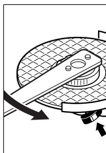
If the quick-clamping nut has been attached correctly and is not damaged, you can loosen it by hand by turning the knurled ring anticlockwise. **Never loosen a tight quick-clamping nut with pliers. Always use the combination wrench.** Insert the combination wrench as shown in the figure.
