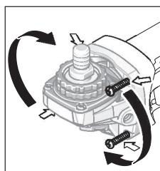
The machine head can be rotated in 90° increments. In this way, the on/off switch can be brought into a more favourable handling position for particular applications, e.g. for left-handed tool users.
