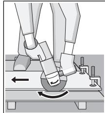
The power tool must always work in an up-grinding motion. Otherwise, there is a risk that it will be pushed uncontrolled out of the cut. For best results when cutting profiles and rectangular tubing, start at the smallest cross section.
