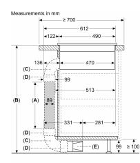
A: Tube length B: Kitchen height C: 90° L-size bow D: Connector sleeve E: Diffusor
