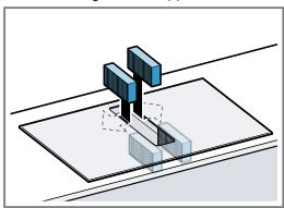
6. Insert the grease filter.
