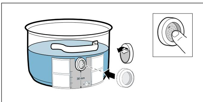
3. Press down all over the surface of the silicone patch, including in the centre. The adhesive requires one hour to fully harden. Do not use or clean the pan during this time.
