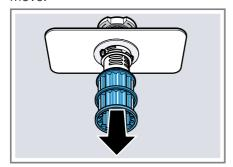
4. Press the locking catches 1 together and lift the coarse filter out (2).
