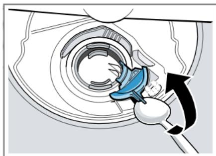
6. Lift the pump cover inwards at an angle and remove.
