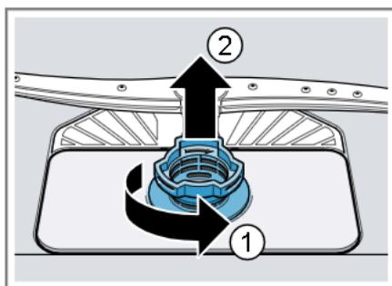
3. Pull down the micro filter to remove.
