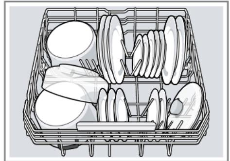
Large plates up to a diameter of 31 cm can be arranged in the bottom basket as shown.
