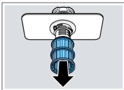
4. Press the locking catches
