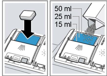
If you are using tablets, one is enough. Insert the tablets in a horizontal position.
