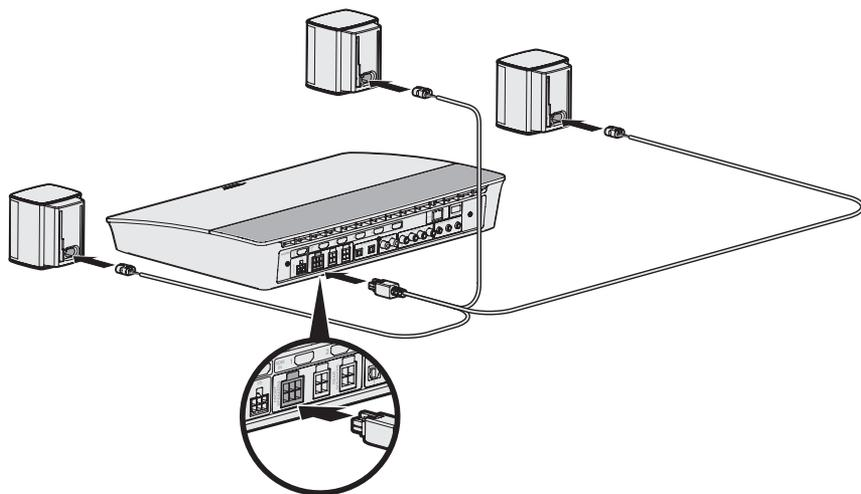
**Note:** The four-pin FRONT SPEAKERS connector on the back of your console is not used.
