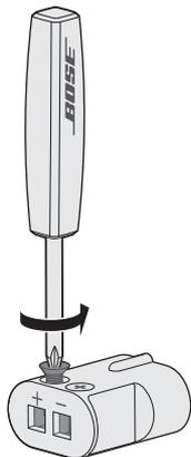
2. **For front speakers:** Insert the bare ends of the four-pin cable into the adapter by placing the red wire marked **L+**, **C+** or **R+** into the red terminal ( **+** ) and the plain wire into the plain silver terminal ( **-** ).
