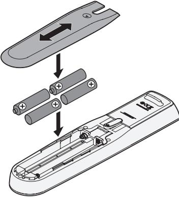
3. Slide the battery compartment cover back into place.
