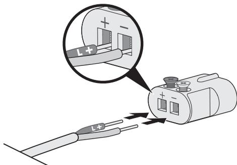
**Note:** Be sure to only insert the bare ends of each exposed wire to avoid clamping the wire's insulation.
