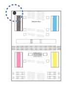
Follow the LCD instructions, and then press [OK] or ▶. The machine prints the Print Quality Check Sheet. Follow the LCD instructions to check the quality of the four colour blocks on the sheet, and then start the cleaning procedure.
