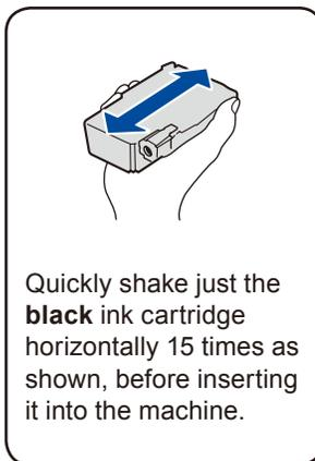
Quickly shake just the **black** ink cartridge horizontally 15 times as shown, before inserting it into the machine.
