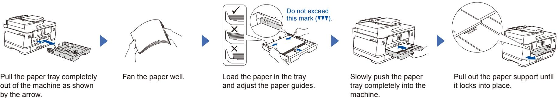
Pull the paper tray completely out of the machine as shown by the arrow.
