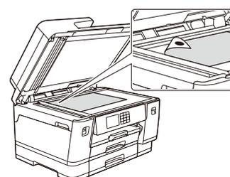
Place the Adjustment Sheet face down on the scanner glass. Make sure the black circle is in the upper left corner of the scanner glass.
