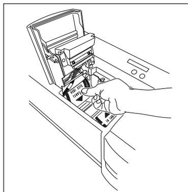
For a jam near the xenon lamp unit (“REMOVE LABEL 3” appears in the LCD):
