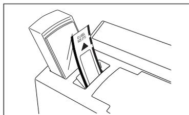
For a jam in the ink ribbon compartment (“REMOVE LABEL 1”, “REMOVE LABEL 2” or “REMOVE LABEL 3” appears in the LCD):
