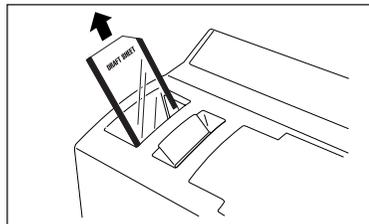
For a jam at the ID label slot (“REMOVE LABEL 1” or “CHANGE LABEL” appears in the LCD):
