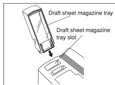
After installing the ink ribbon cassette and the magazine tray loaded with draft sheets, you can use the Stampcreator P-touch Editor software or Stampcreator Express software to create any layout containing graphics and text, and then engrave it into a stamp.
