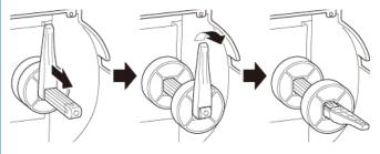
Place the label roll on the Label Supply Spindle and then flip the Label Roll Guard upwards to hold it in place.
