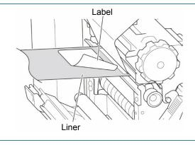
12. Thread the liner through the Label Peeler Cover Slot.
