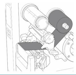
Wind the Ribbon Rewind Spindle counterclockwise about three to five turns until the ribbon is smooth, flat, and without wrinkles.
