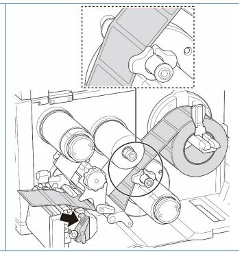
5. Move the Media Sensor by adjusting the Media Sensor Position Adjustment Knob. Make sure the position of the Gap or Black Mark Sensor matches the position of the Gap/Black Mark on the label roll.
