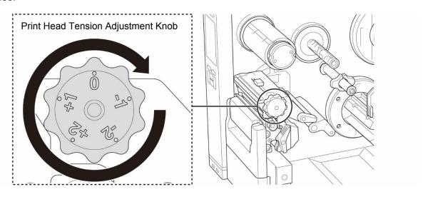
For labels (less than 2" width), set the Print Head Tension Position Adjustment Slider as close to the label center as possible to prevent unnecessary friction between the Print Head and the Platen Roller.
