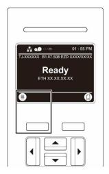
To select an option on the Main Menu, use the Navigation buttons to browse the options and then press the button under the  $\bigcirc$  icon.
