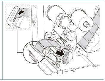
6. Move the Media Sensor by adjusting the Media Sensor Position Adjustment Knob. Make sure the position of the Gap or Black Mark Sensor matches the position of the Gap/Black Mark on the label roll.
