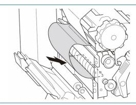
13. Adhere the liner to the Media Rewind Spindle. Wind the liner on the Media Rewind Spindle until the liner is fully stretched.
