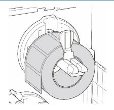
4. Push the Print Head Release Lever and thread the label through the Media Guide Bar, Damper, Media Sensor, and Front Label Guide to install the media. Align the Label Roll Guard with the label width.
