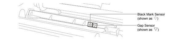
6. Adjust the Front Label Guide to fix the media position.
