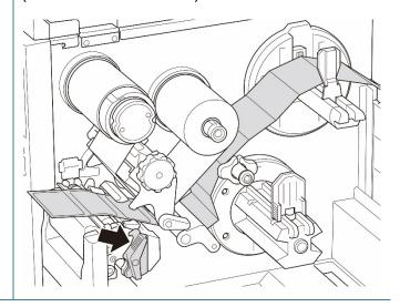
4. Move the Media Sensor by adjusting the Media Sensor Position Adjustment Knob. Make sure the position of the Gap or Black Mark Sensor matches the position of the Gap/Black Mark on the label.
