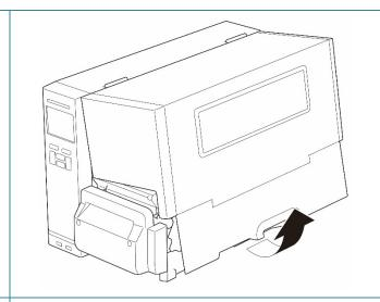
Slide the Label Roll Guard horizontally to the end of the Label Supply Spindle, and then flip down the Label Roll Guard.
