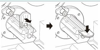
11. Install the Paper Core onto the Media Rewind Spindle.
