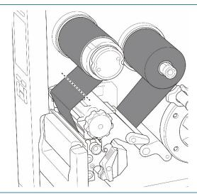
While pushing the Ribbon Release Button (1), remove the ribbon from the Ribbon Rewind Spindle, and discard it.
