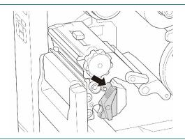
4. Thread the ribbon under the ribbon guide bar and through the ribbon sensor slot following the loading path printed on the Media Cover.
