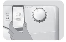
In order to restart a cycle which has already been downloaded to the Smart Touch position, select it with the programme knob, and then simultaneously press the START/PAUSE and the OPTIONS buttons as indicated on the control panel. Thick cases or metallic stickers on your smartphone could affect or prevent the transmission of data between machine and telephone. If necessary, remove them.
