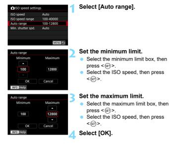
The [Minimum] and [Maximum] settings will also function as the minimum and maximum speeds for ISO speed safety shift (p.473).
