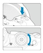
Press a button such as  $\langle M-F_{\eta} \rangle$  or  $\langle ISO \rangle$ , then turn the  $\langle 0 \rangle$  dial.
