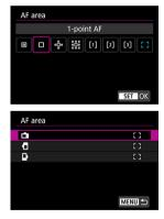
The screen above is displayed when [AF: Orientation linked AF point] ((i)) is set to [Separate AF pts: Area+pt]. Set separate AF areas after choosing vertical and horizontal orientations.
