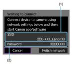
Check the SSID (1) and Password (2) displayed on the camera screen.
