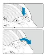
Press a button such as < M-Fn > or < ISO >, then turn the <  $\stackrel{\text{\tiny cons}}{=}$  > dial.
