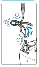
Pass the end of the strap through the camera's strap mount eyelet from the bottom. Then pass it through the strap's buckle as shown in the illustration. Pull the strap to take up any slack and make sure the strap will not loosen from the buckle.
