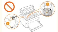
Do not turn OFF the machine during printing. Also, do not open and close the cover and do not remove or insert paper during printing. Doing so can cause paper jams.
