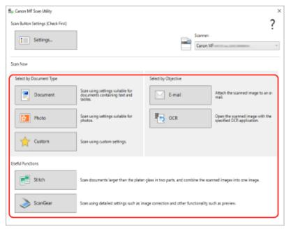
Click [ScanGear] to display ScanGear MF and configure the advanced scan settings. For more information, click [ " ] on ScanGear MF to display help.
