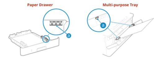
• Check that the paper guides are aligned with the markings and are not too loose or too tight.
