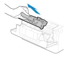
**3** Remove the replacement toner cartridge from the protective case.
