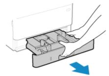
Always hold the paper drawer with both hands and pull it out gently. If you pull the drawer out with only one hand, it may be too heavy to hold, causing it to fall and be damaged.
