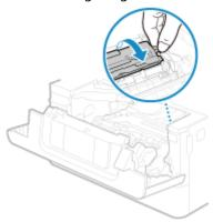
Do not release the transport guide until you have returned it to its original position in step 6.
