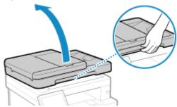
Place the front of the ID card face down on the platen glass in the portrait orientation while aligning the corner of the ID card with the top left corner of the platen glass.
