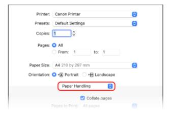
2 Select the [Scale to fit paper size] checkbox, and in [Destination Paper Size], select the paper size to print on.
