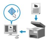
You can scan an original and save the scanned data to a computer connected to the machine. You can set the format and save location when scanning from a computer. This method lets you see the scanned data immediately on the computer screen so you can check the image quality and make adjustments.
