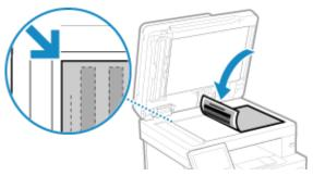
Place the print side of the calibration image face down with the fine black line on the left.
