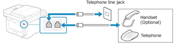
Connect the handset or telephone to the handset/external telephone jack (HAND SET/EXT.) on the machine.
