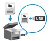
You can scan an original and save the scanned data to a USB memory device connected to the machine.
