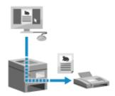
You can convert a document or photo to a black and white image and send it via a fax driver installed on a computer connected to the machine.
