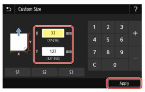
When frequently used non-standard sizes are registered, you can call these up by pressing [S1] to [S3].
