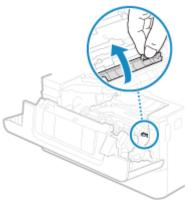
Do not release the transport guide until you have returned it to its original position in step 3.
