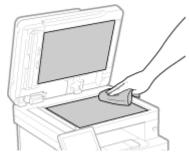
Wipe with a cloth soaked in water and wrung out. Next, wipe with a soft, dry cloth.
