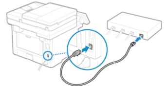
When the machine is connected to the wired LAN, [ ] appears on the [Home] screen and screen of each function.
