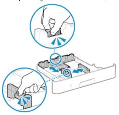
2 Align the projections on the paper guides with the size markings of the paper to be loaded.
