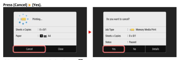
If the above screen is not displayed, press [๗] on the control panel ▶ [Yes].
