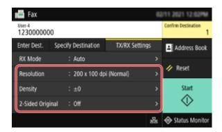
If the recipient cannot read the text or the sent fax was not as intended, the settings can be adjusted and the fax resent.
