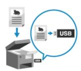
You can save scanned data to a USB memory device connected to the machine. This is convenient when using scanned data on a computer without a network connection or when on the go.
