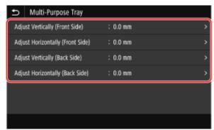
**Example:** When adjusting the print position of the front side of the paper in the vertical direction Select [Adjust Vertically (Front Side)].
