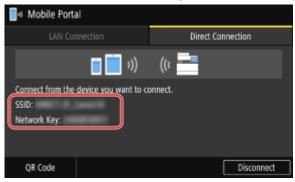
In the Wi-Fi settings of the mobile device, select the SSID of the machine, and enter the network key. For details about how to configure the Wi-Fi settings, see the manual of the mobile device.
