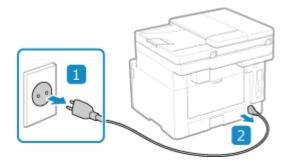
**3** Unplug all cables and cords connected to the machine.
