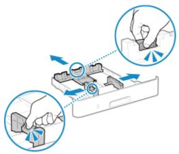
While pressing the lock release lever, move the paper guides.
