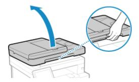
**3** Wipe the platen glass and rear of the feeder.
