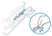
While pressing the lock release lever, move the paper guides.
