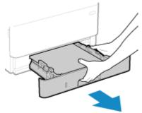
Always hold the paper drawer with both hands and pull it out gently. If you pull the drawer out with only one hand, it may be too heavy to hold, causing it to fall and be damaged.
