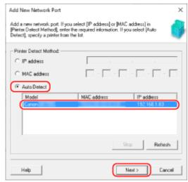
If the machine is not displayed, click [Refresh]. If the machine is still not displayed, select [IP address] or [MAC address], enter the IP address or MAC address of the machine, and then click [Next].
