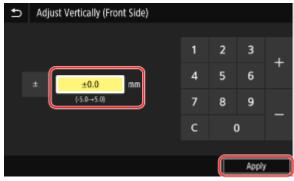
Specify the adjustment direction using + and -, and specify the adjustment width in units of 0.1 mm.
