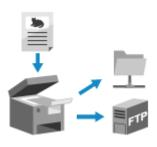
You can save scanned data to a shared folder on a computer or FTP server. This is convenient for sharing the scanned data of a paper document on a network
