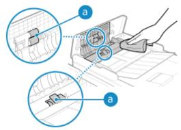
Wipe with a cloth soaked in water and wrung out. Next, wipe with a soft, dry cloth.
