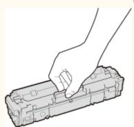
• To avoid scratching the surface ( a) of the drum inside the machine or exposing it to light. Do not touch the electrical contacts ( b) or the toner cartridge memory ( ).
