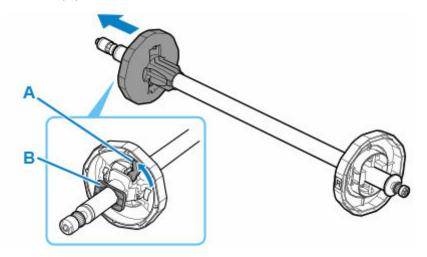
**2.** If using 3-inch core paper, align 3-inch paper core attachment tabs (A) with roll holder holes (B) and insert firmly.
