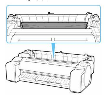
If the paper is jammed by the ejection guide
