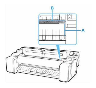
**5.** Pull the release lever forward and close the top cover.
