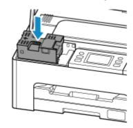
**9.** Slide the maintenance cartridge to the right until it reaches the end.
