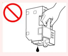
• Put the used one immediately into the plastic bag that came with the new maintenance cartridge and seal the bag by tying the opening tightly to prevent the ink from leaking.
