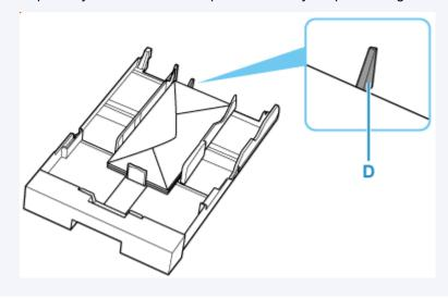
**4.** Move the paper guide and adjust the guides to edge of the paper stack.
