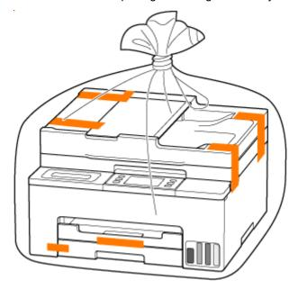
**12.** Attach the protective material to the printer when packing the printer in the box.
