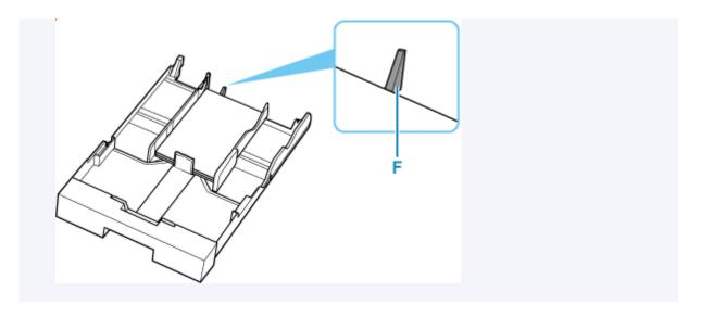
**4.** Move the paper guide and adjust the guides to edge of the paper stack.
