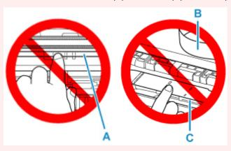
If you soil or scratch this part by touching it with paper or your hand, it could damage the printer.
