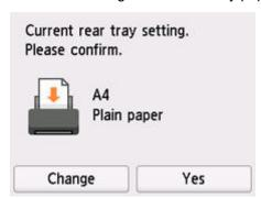
If the page size on the touch screen matches the size of the paper loaded in the rear tray, select **Yes**. If not, select **Change** to change the setting in accordance with the size of the loaded paper.
