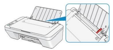
If there are any foreign objects in the rear tray, be sure to turn off the machine, unplug it from the power supply, then remove the foreign object.
