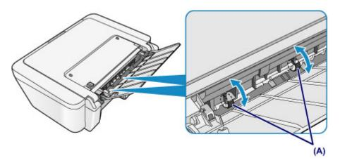
After cleaning the paper feed rollers, turn on the power, then clean the paper feed rollers again.
